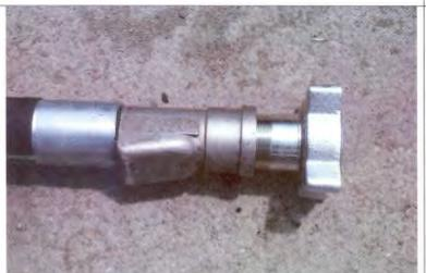
Completed Delivery Hose Assembly. Is the delivery hose assembly with the attached coupling required to be tested in accordance with 180.416(f).
