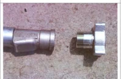
Hose assembly with attached coupling (Acme Fitting) in the process of creating a Delivery Hose Assembly
