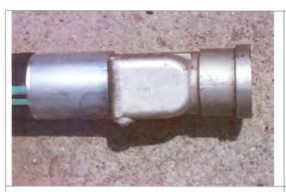
Hose assembly. Note this hose assembly comes with complete test paper work is marked with a unique ID number and the month and year the hose assembly was tested.
