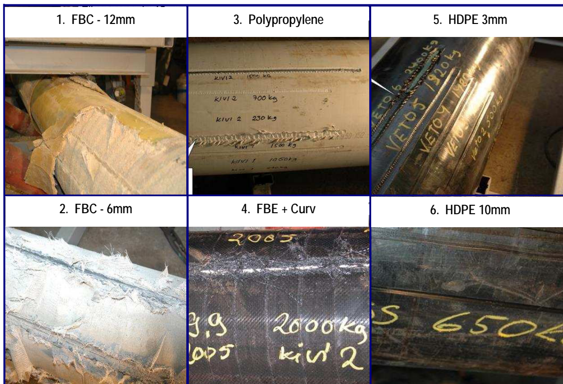
Figure 5.3 – Pipeline Coatings Tested for Severe Construction Conditions (Christianson, 2006)
