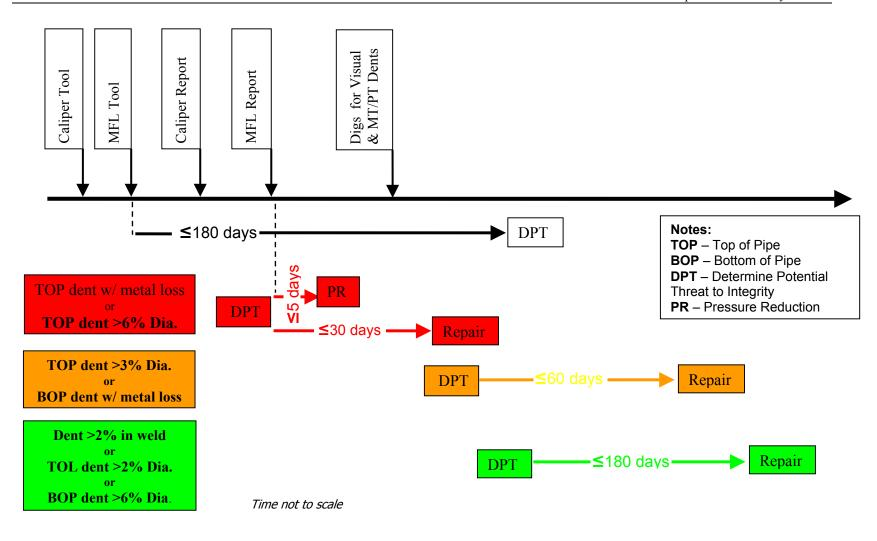
Figure 8-1 Time Line for Response to Geometry Defects – Liquid Pipelines
