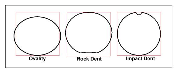
Figure 5-1 Schematic illustrating the three types of deformation that are the primary focus of this report.
