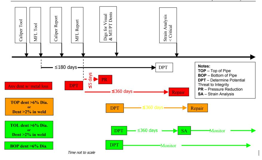
Figure 8-2Time Line for Response to Geometry Defects – Gas Pipelines
