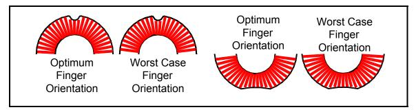
Figure 3-6 Schematic illustrating the function of a fourth-generation caliper tool equipped with closely spaced fingers of approximately 0.75 inch width for two types of dents and in two orientation.
