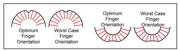
Figure 3-5 Schematic illustrating the function of a third-generation caliper tool equipped with narrow fingers for two types of dents and in two orientation.
