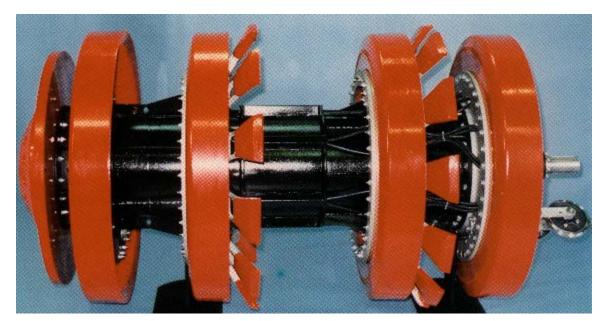
Figure 3-3 Photograph of a third-generation caliper tool with two staggered rows of paddles with a radius tip that conforms to the inside surface of the pipeline.
