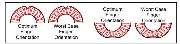
Figure 3-4 Schematic illustrating the function of a third-generation caliper tool equipped with radius-tipped paddles for two types of dents and in two orientations.
