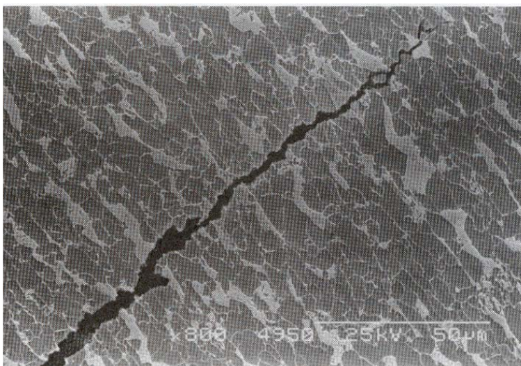
Figure 4-9 Transgranular Cracking in Pipeline Steel (Revie 2000)
