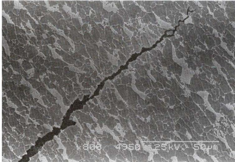
**Figure 4-9 Transgranular Cracking in Pipeline Steel (Revie 2000)**
