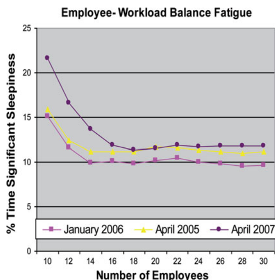
FIGURE 5. Effect of reducing the staffing level (number of qualified marine pilots) on fatigue risk (% time significantly sleepy) at three different levels of workload (ships per month to pilot) in 3 separate months. Reprinted from Moore-Ede et al, 73 by permission of CIRCADIAN®.
