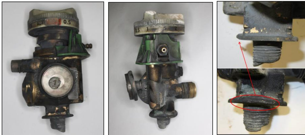
Figure 6 – Views of VIPR (Rotated Clockwise) and Flange Close-up
