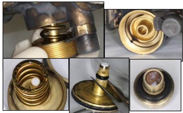
D - Regulator Assembly, PTFE Piston, Spring and Inlet Filter (lubricant on filter surface)
