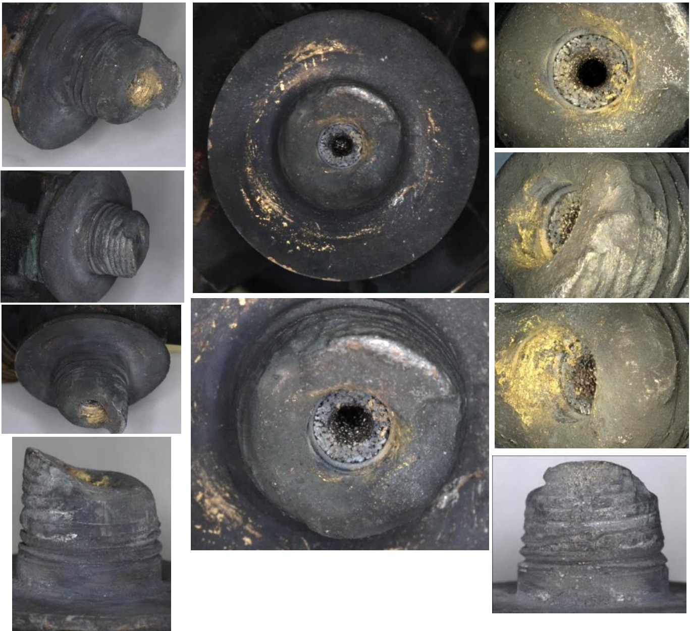
Figure 8 – Magnified Images of the VIPR Thread Damage
