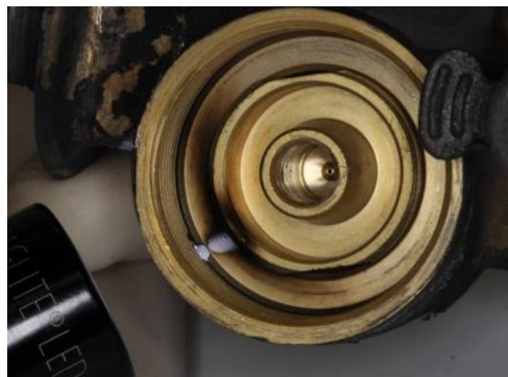
Figure 10 – Regulator Atmospheric Vent Port Illuminated from Exterior
