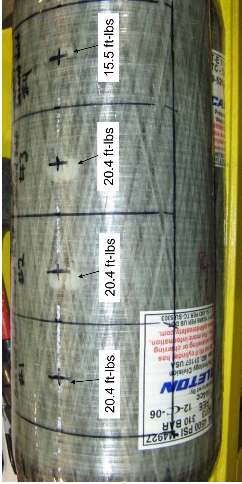
Figure 12. Photograph of impact sites for cylinder 52079
