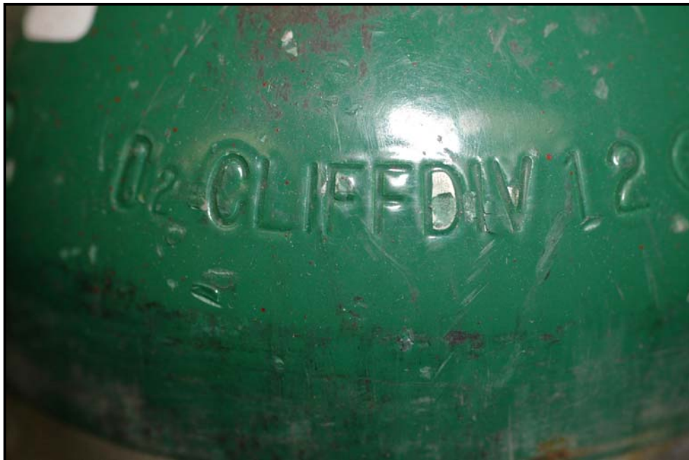
Figure 68: Indented marking on the DOT-3AL cylinder # AR0119572
