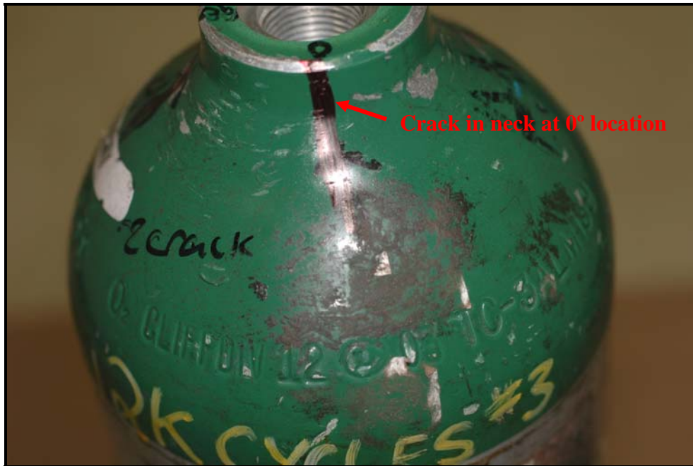
Figure 47: Shows the orientation of the crack in the shoulder area of DOT-3AL cylinder # AR0116501 at 0° location with respect to the indented markings.
