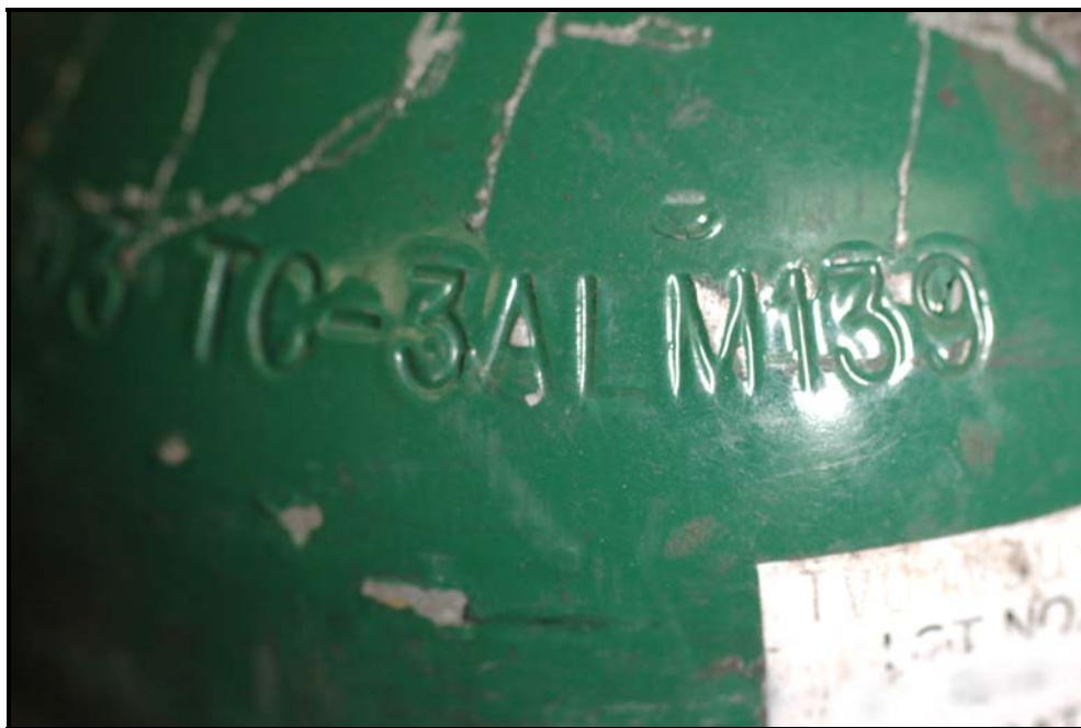
Figure 54: Indented marking on the DOT-3AL cylinder # AR0118110
