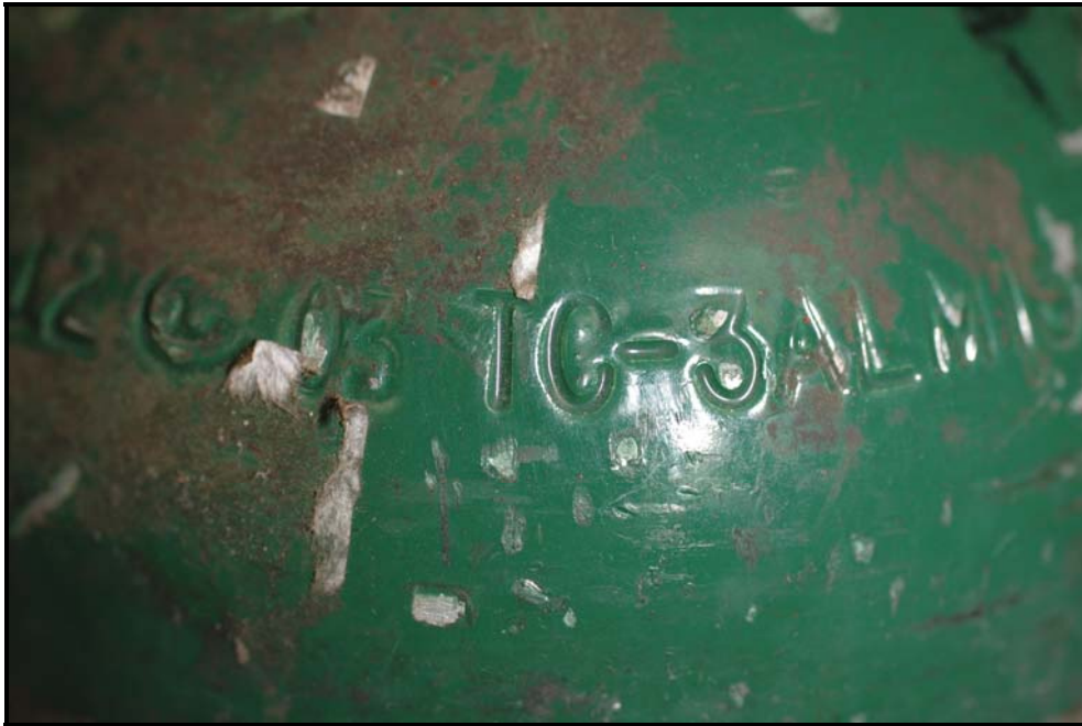
Figure 37: Indented marking on the DOT-3AL cylinder # AR0116501
