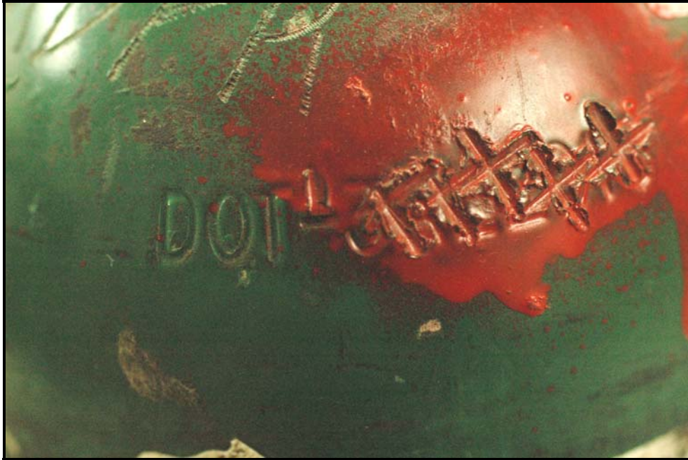
Figure 3: Indented marking on the DOT-3AL cylinder # AR0119582
