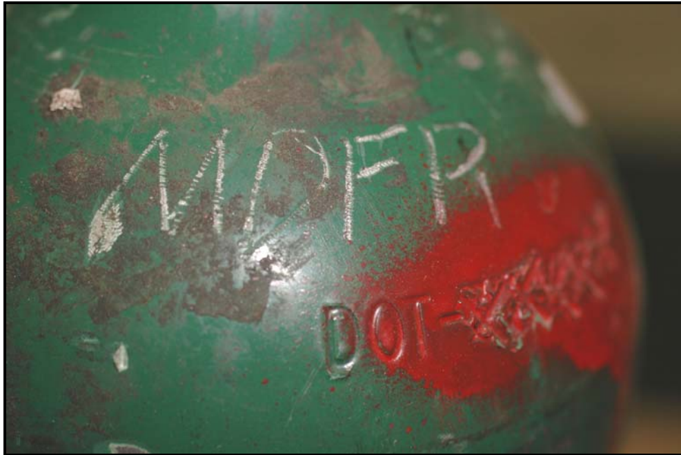
Figure 71: Indented marking on the DOT-3AL cylinder # AR0119572
