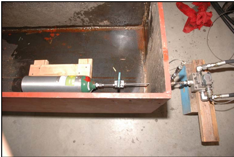
Figure 82: Test set up for pressure cycling DOT-3AL 2015 cylinders up to 12,000 cycles and until failure of the cylinder
