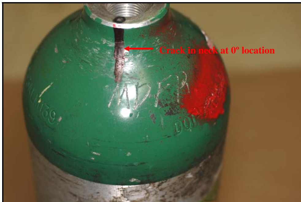
Figure 14: Shows the orientation of the crack in the shoulder area of DOT-3AL cylinder # AR0119582 at 0° location with respect to the indented markings.
