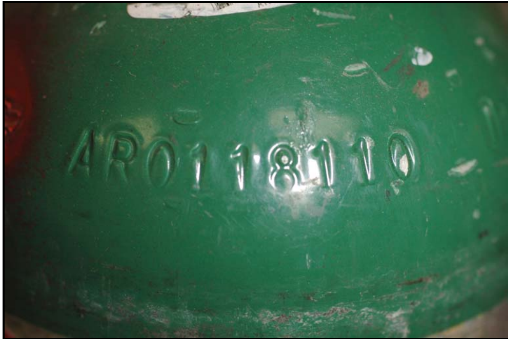
Figure 51: Indented marking on the DOT-3AL cylinder # AR0118110
