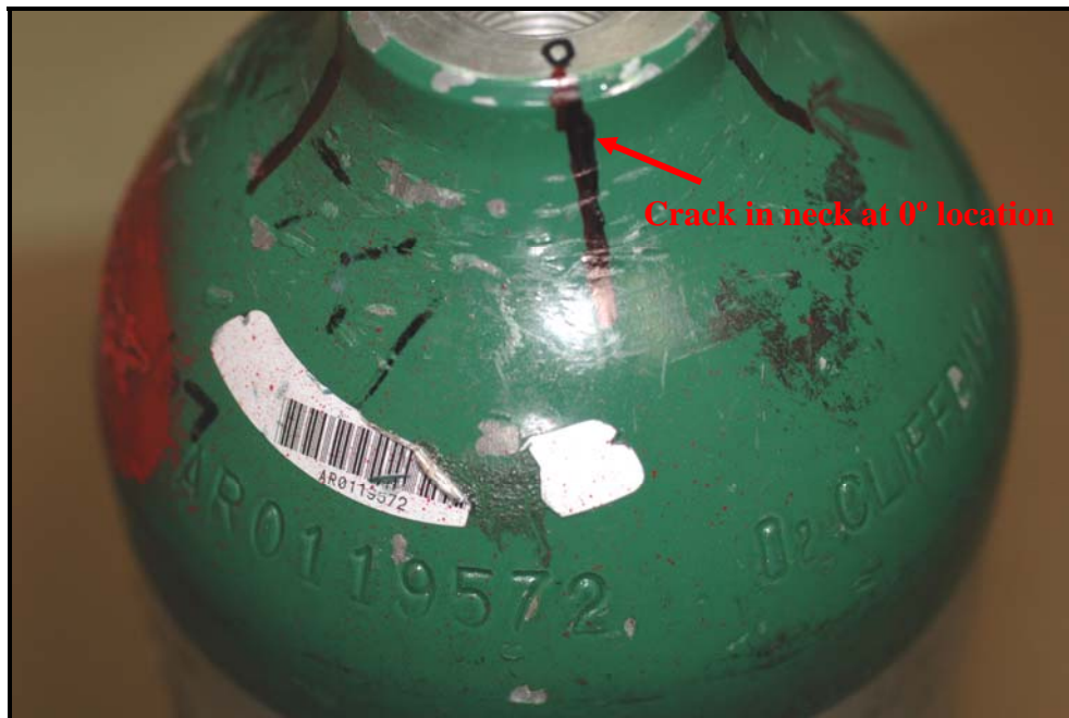
Figure 80: Shows the orientation of the crack in the shoulder area of DOT-3AL cylinder # AR0119572 at 0° location with respect to the indented markings.
