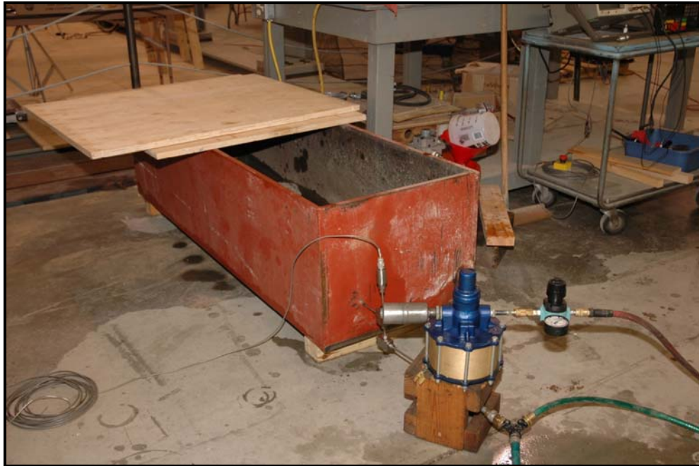
Figure 95: Test set up for hydraulic burst testing of cylinder #AR0119582
