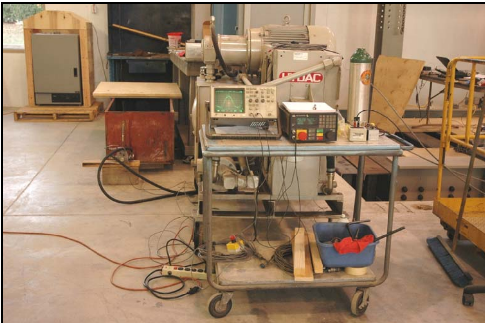
Figure 84: Test set up for pressure cycling DOT-3AL 2015 cylinders up to 12,000 cycles and until failure of the cylinder
