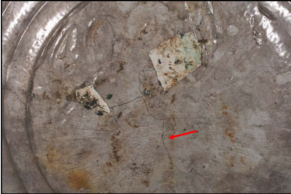
Figure 91: Shows the leak at the base of the cylinder # AR0119572
