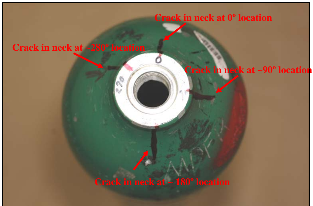
Figure 81: Shows the orientation of the cracks in the shoulder area of DOT-3AL cylinder AR0119572 with respect to the 0° crack location.
