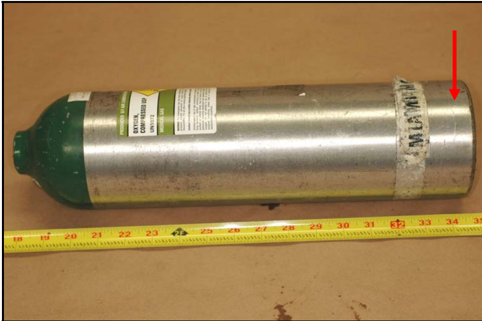
Figure 93: Shows the location where the leak occurred as indicated by the arrow. The cylinder # AR0118110 leaked on the wall of the cylinder near the bottom of the cylinder.
