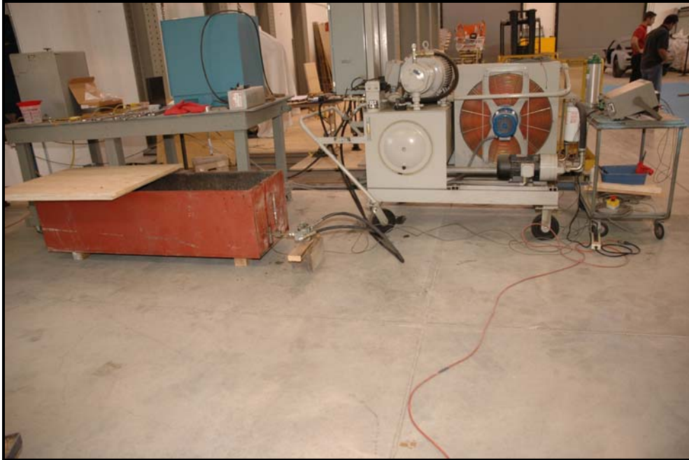
Figure 83: Test set up for pressure cycling DOT-3AL 2015 cylinders up to 12,000 cycles and until failure of the cylinder
