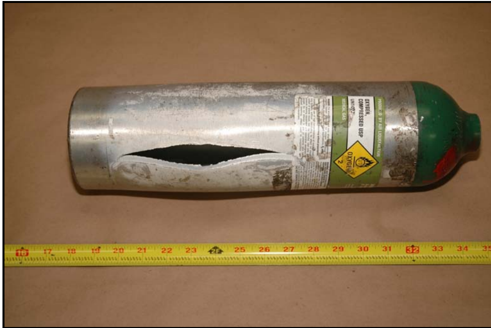
Figure 99: Ruptured cylinder #AR0119582 after hydraulic burst testing
