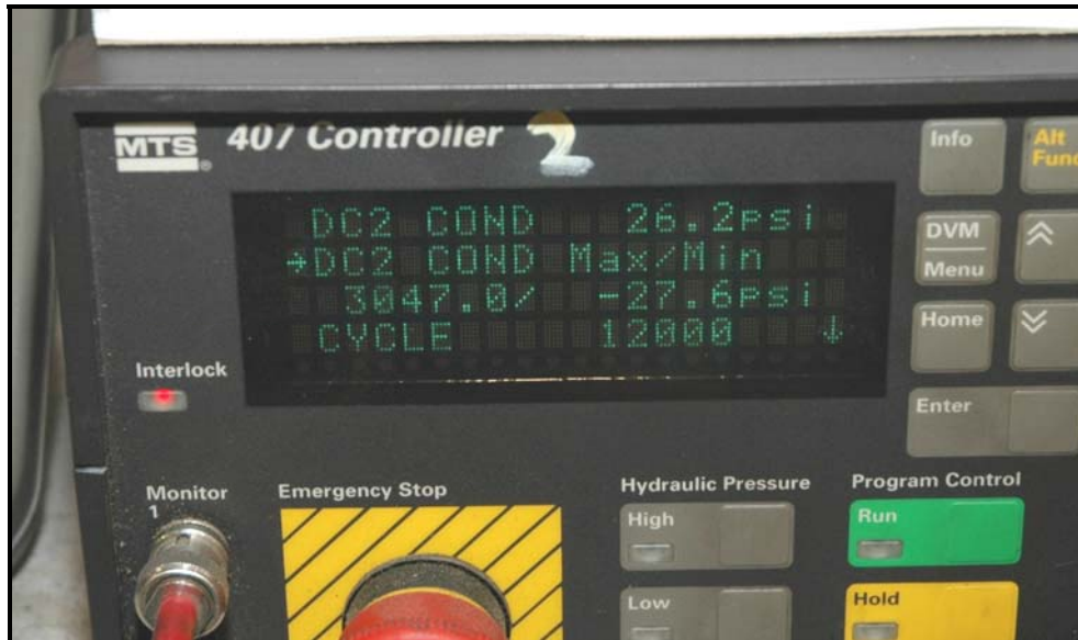
Figure 87: Shows the maximum/minimum pressure and the number of cycles completed during the pressure cyclic testing of the DOT – 3AA cylinder # AR0118046
