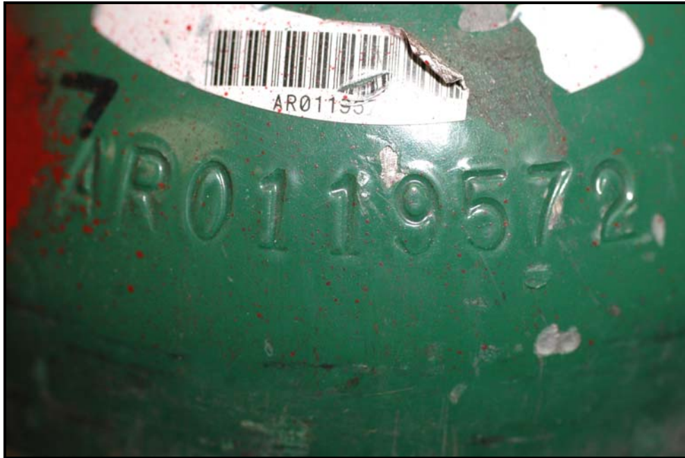
Figure 67: Indented marking on the DOT-3AL cylinder # AR0119572
