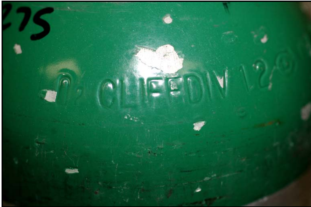
Figure 19: Indented marking on the DOT-3AL cylinder # AR0118046
