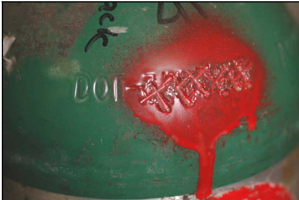
Figure 50: Indented marking on the DOT-3AL cylinder # AR0118110
