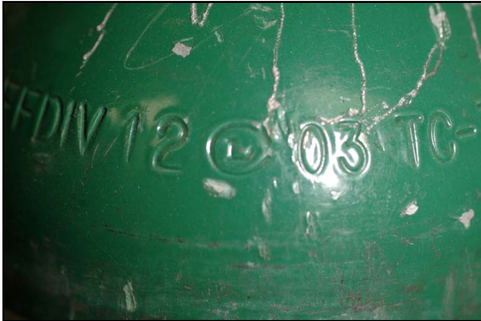
Figure 53: Indented marking on the DOT-3AL cylinder # AR0118110
