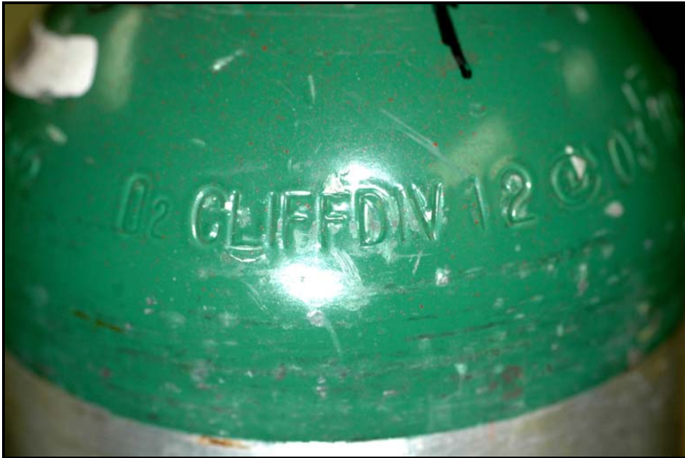
Figure 5: Indented marking on the DOT-3AL cylinder # AR0119582
