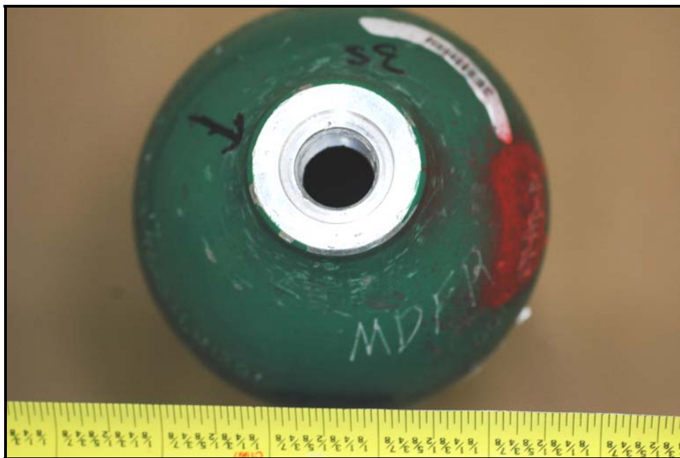
Figure 10: Shows neck and shoulder of DOT-3AL cylinder # AR0119582
