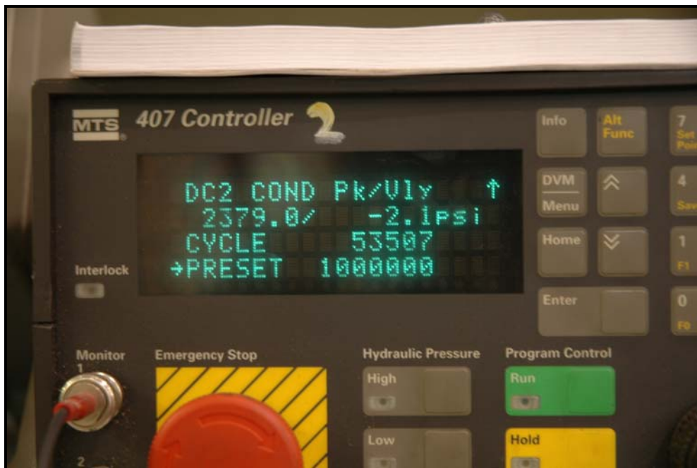
Figure 92: Shows the maximum/minimum pressure and the number of cycles until the failure of the DOT – 3AA cylinder # AR0118110. The cylinder leaked after 53,507 cycles.
