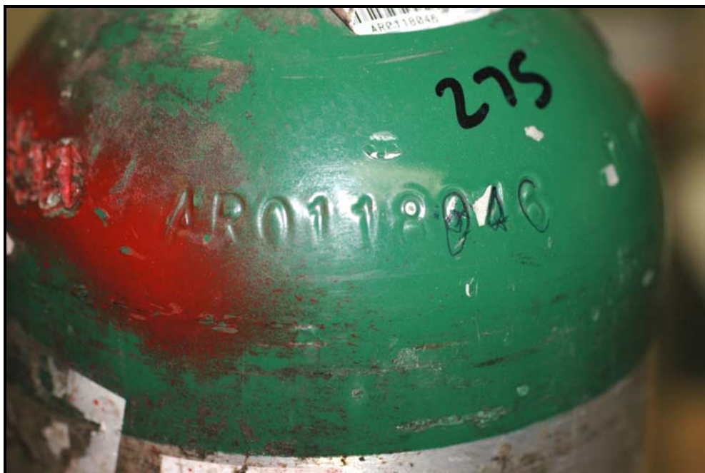
Figure 18: Indented marking on the DOT-3AL cylinder # AR0118046
