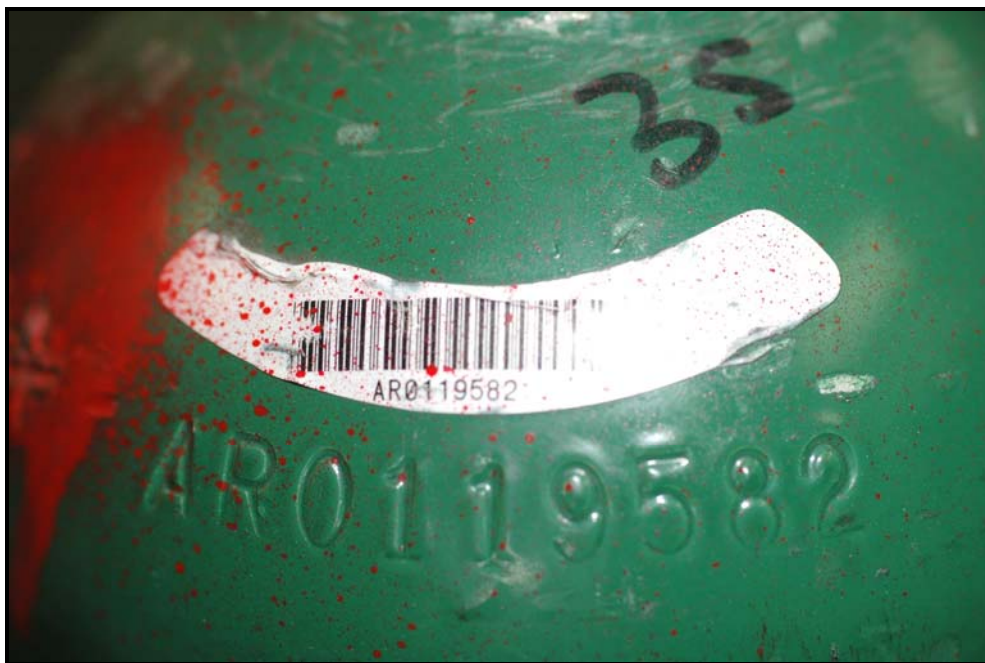
Figure 4: Indented marking on the DOT-3AL cylinder # AR0119582
