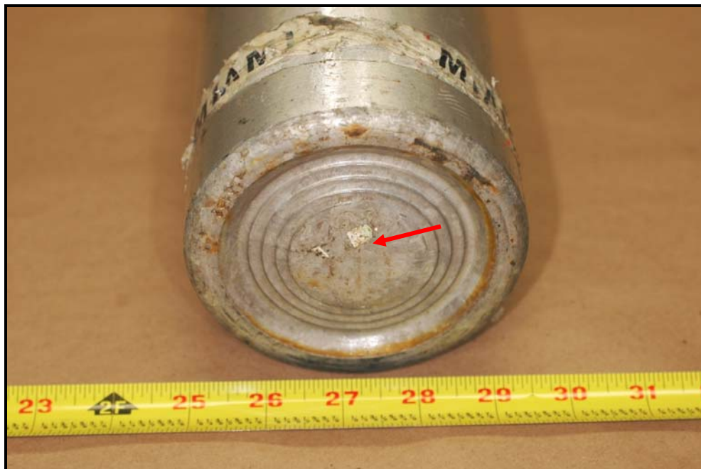
Figure 90: Shows the location where the leak occurred as indicated by the arrow. The cylinder # AR0119572 leaked at the base of the cylinder.
