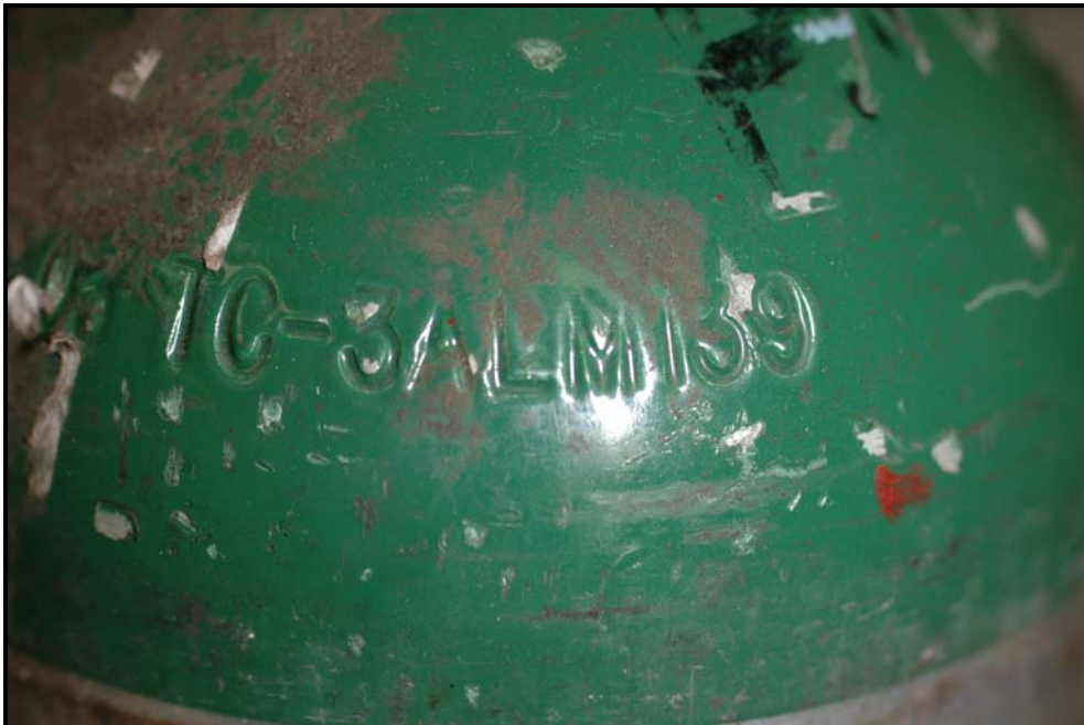
Figure 38: Indented marking on the DOT-3AL cylinder # AR0116501
