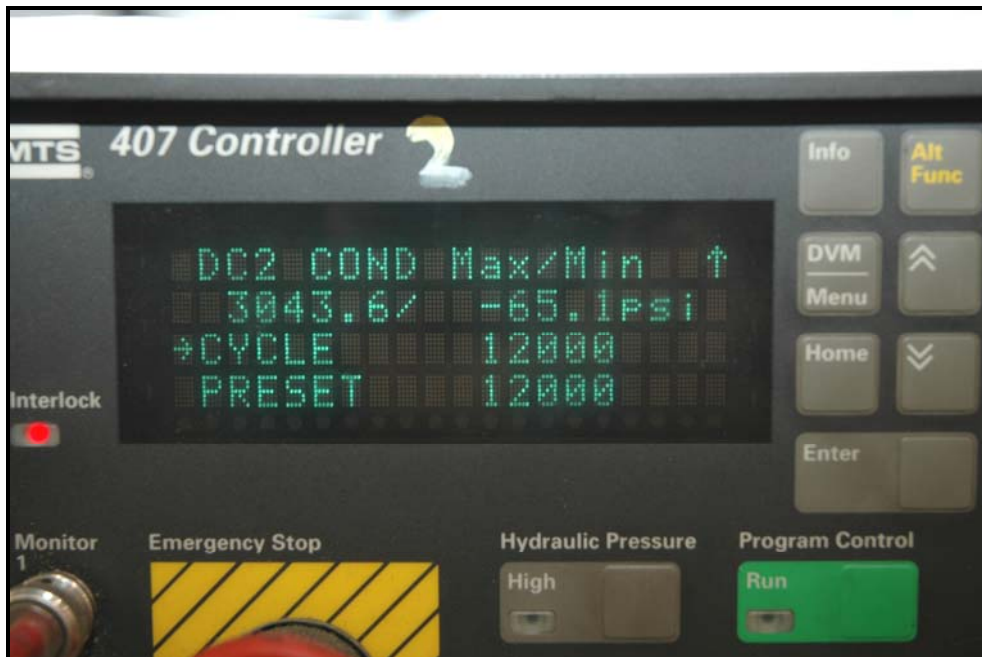
Figure 88: Shows the maximum/minimum pressure and the number of cycles completed during the pressure cyclic testing of the DOT – 3AA cylinder # AR0116501
