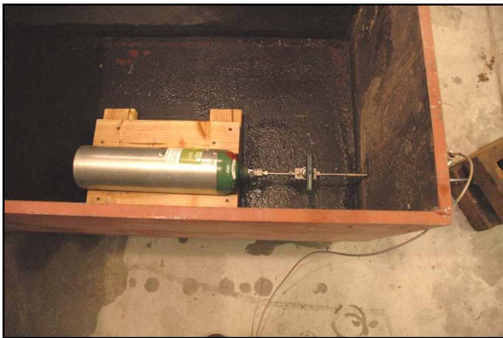
Figure 96: Test set up for hydraulic burst testing of cylinder #AR0119582
