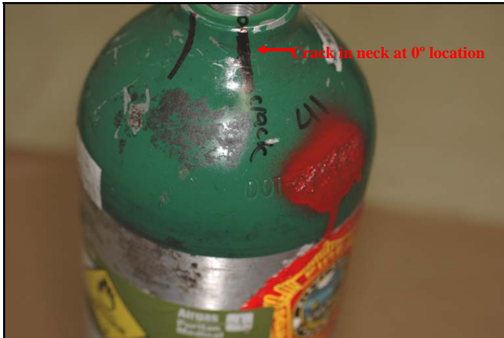
Figure 63: Shows the orientation of the crack in the shoulder area of DOT-3AL cylinder # AR0118110 at 0° location with respect to the indented markings.
