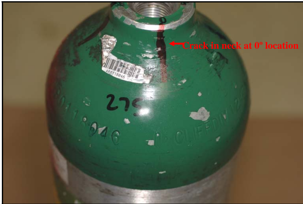
Figure 31: Shows the orientation of the crack in the shoulder area of DOT-3AL cylinder # AR0118046 at 0° location with respect to the indented markings.
