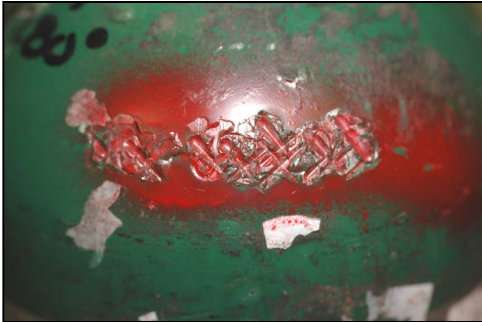
Figure 17: Indented marking on the DOT-3AL cylinder # AR0118046
