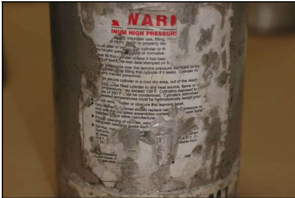
Figure 59: Labels on the DOT-3AL cylinder # AR0118110
