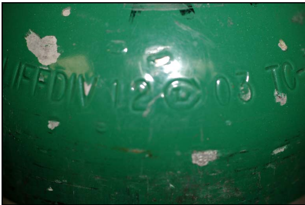
Figure 20: Indented marking on the DOT-3AL cylinder # AR0118046
