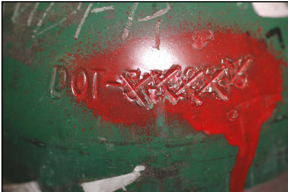
Figure 66: Indented marking on the DOT-3AL cylinder # AR0119572
