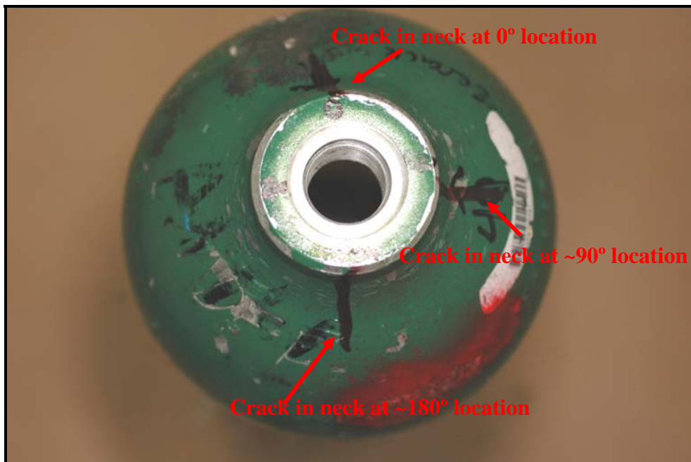
Figure 48: Shows the orientation of the cracks in the shoulder area of DOT-3AL cylinder # AR0116501 with respect to the 0° crack location.
