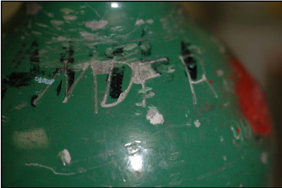
Figure 39: Indented marking on the DOT-3AL cylinder # AR0116501
