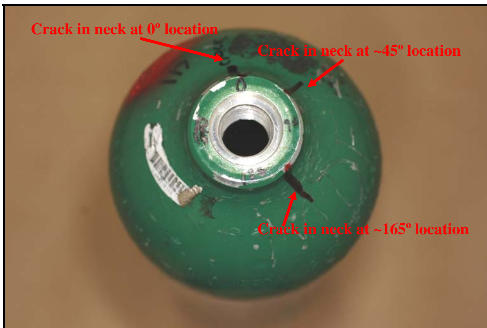
Figure 64: Shows the orientation of the cracks in the shoulder area of DOT-3AL cylinder # AR0118110 with respect to the 0° crack location.
