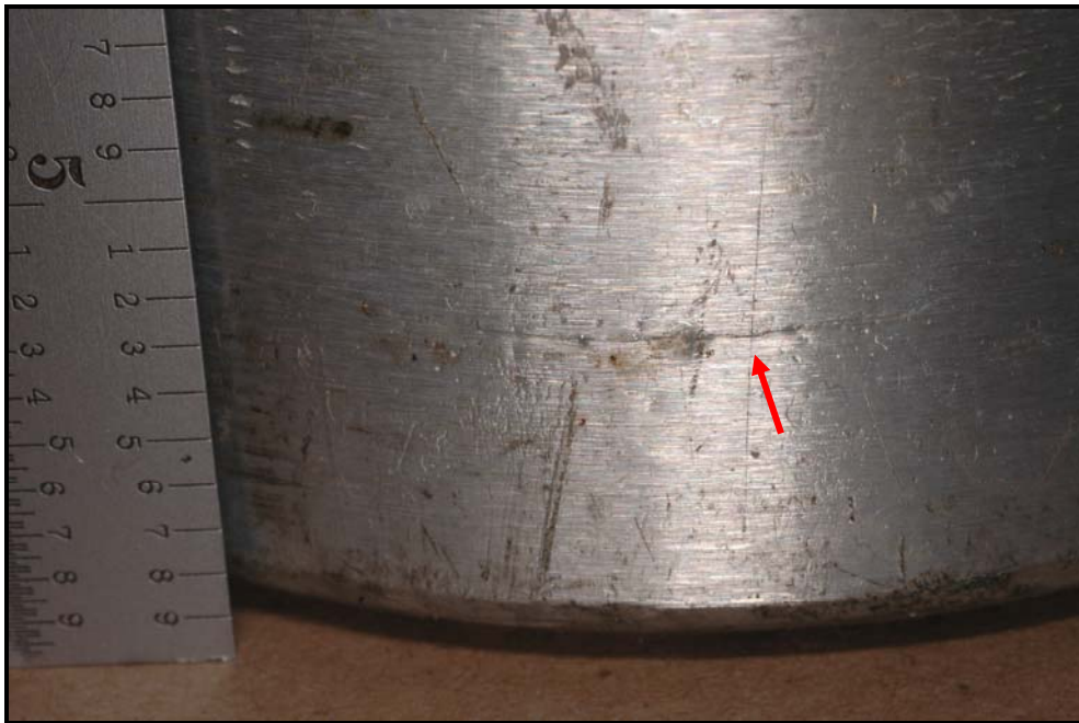
Figure 94: Shows the leak on the wall of the cylinder near the bottom of the cylinder # AR0118110
