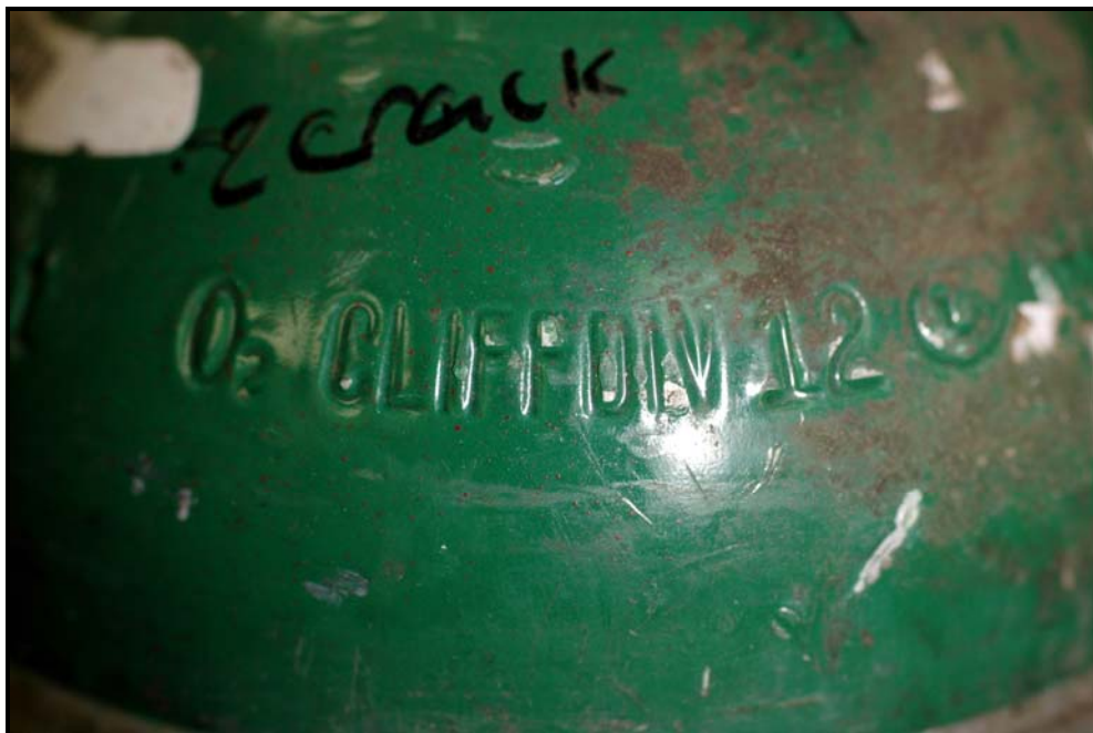
Figure 36: Indented marking on the DOT-3AL cylinder # AR0116501
