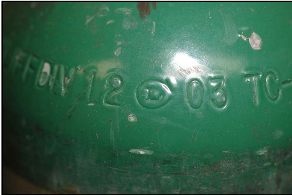
Figure 69: Indented marking on the DOT-3AL cylinder # AR0119572
