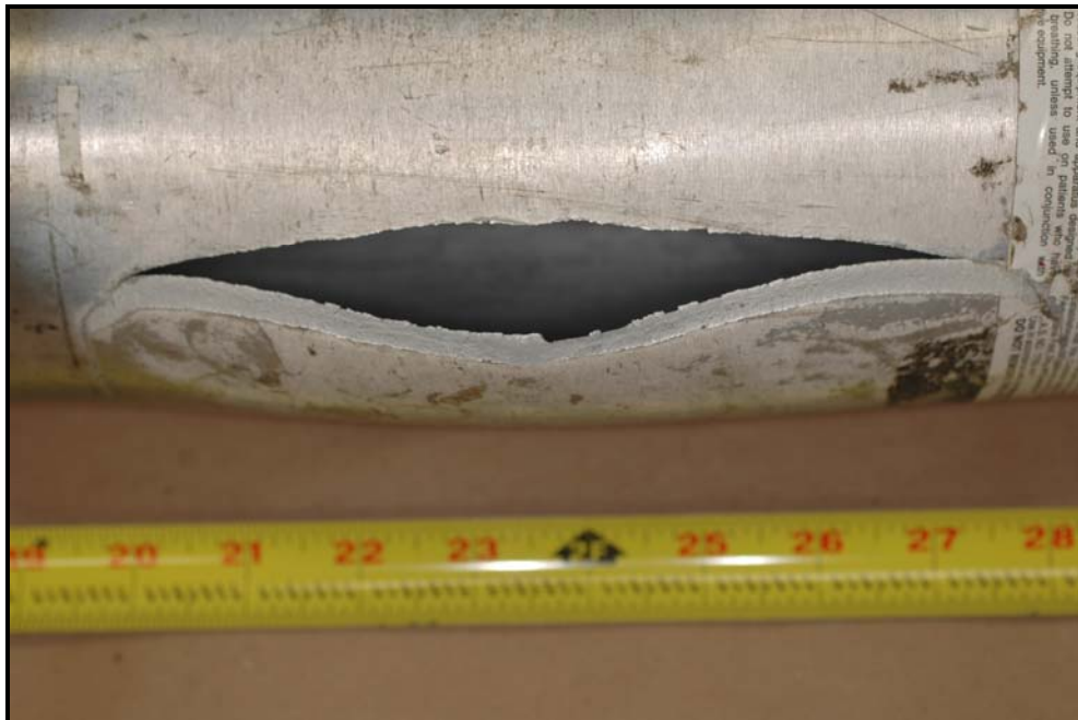
Figure 100: Ruptured cylinder #AR0119582 after hydraulic burst testing
