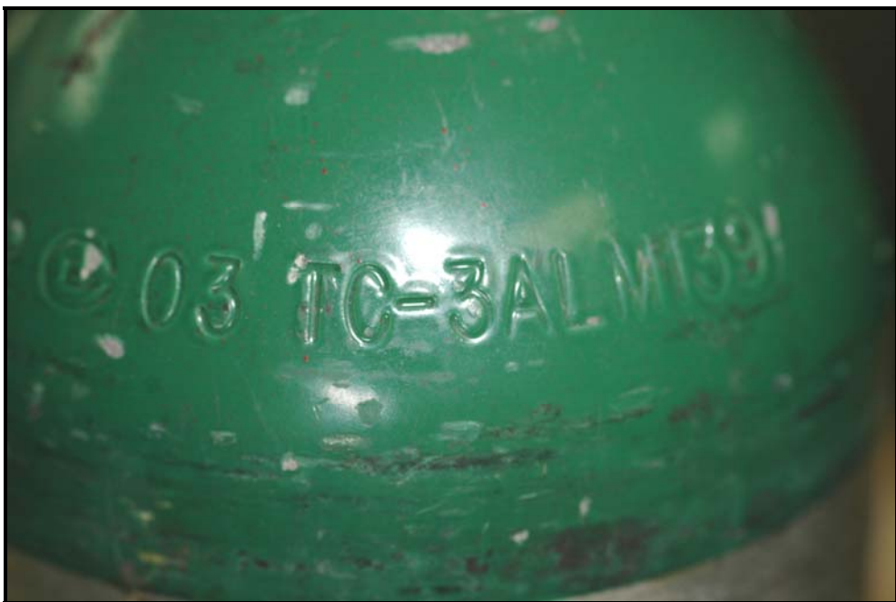
Figure 6: Indented marking on the DOT-3AL cylinder # AR0119582
