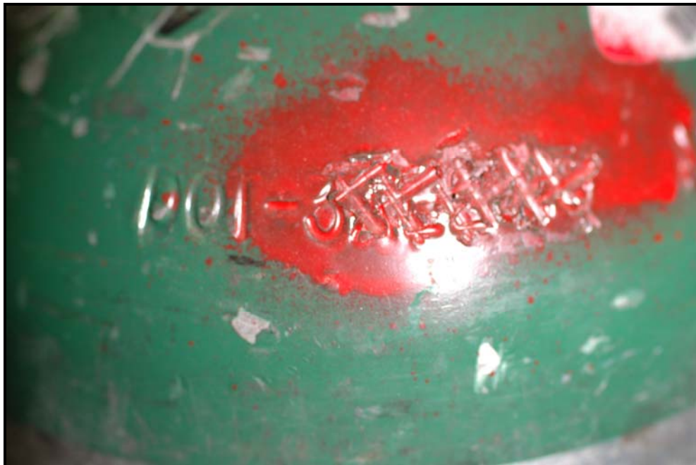
Figure 34: Indented marking on the DOT-3AL cylinder # AR0116501
