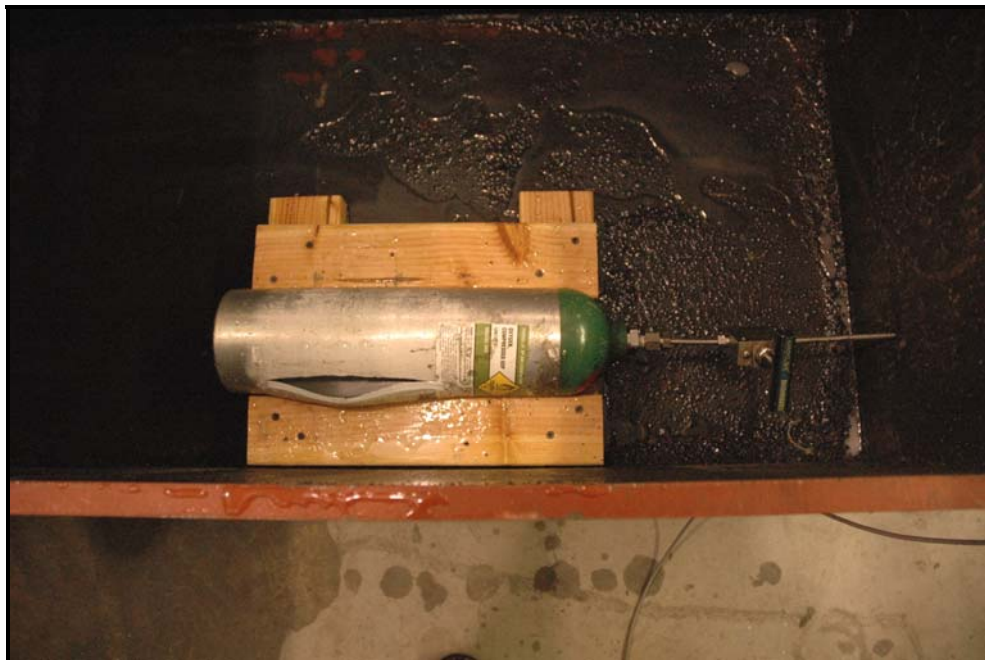
Figure 98: Ruptured cylinder #AR0119582 after hydraulic burst testing
