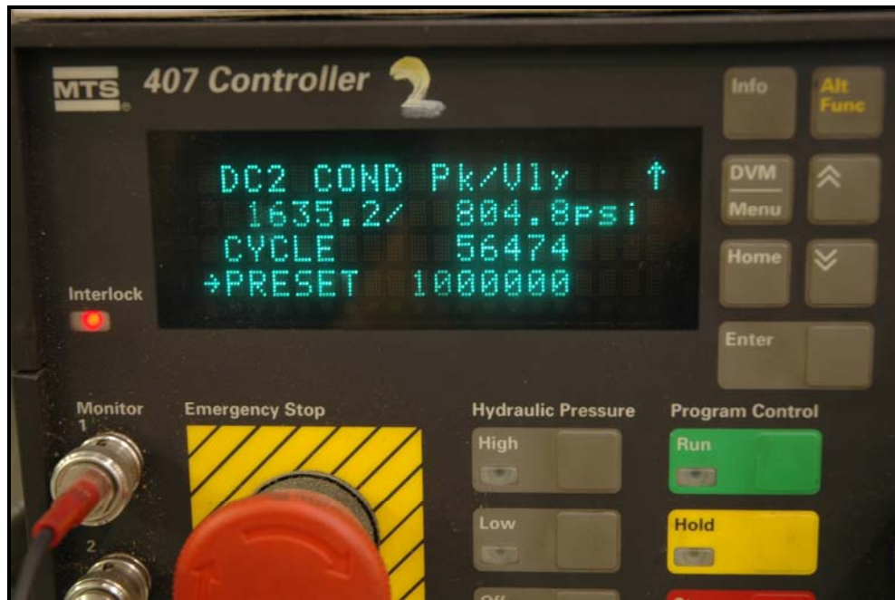
Figure 89: Shows the maximum/minimum pressure and the number of cycles until the failure of the DOT – 3AA cylinder # AR0119572. The cylinder leaked after 56,474 cycles.
