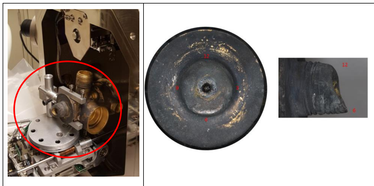
Figure 17 – SEM Chamber Positioning Fixture and Orientation of VIPR Threads for Elemental Characterization of Residues
