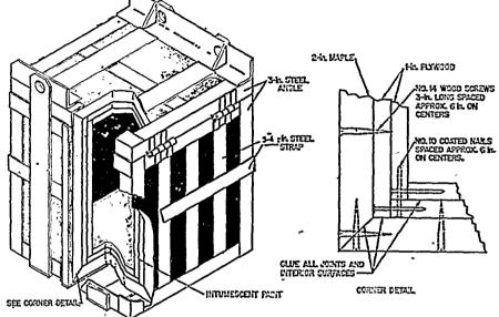
RADIOISOTOPE CHIPPING CASK FIRE AND IMPACT SHIELD.
