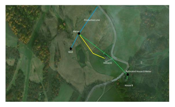
Prior to the end of March 2020, the pressure in the production line upstream of both regulators for House A and House B was 10 pounds per square inch, gauge ("PSIG") and the pressure in the lines downstream of both regulators was approximately 4-6 ounces. Subsequent to the relocation of the meter and regulator for House B, the pressure in the line upstream of the relocated House B regulator (downstream from the original regulator location) increased from 4-
