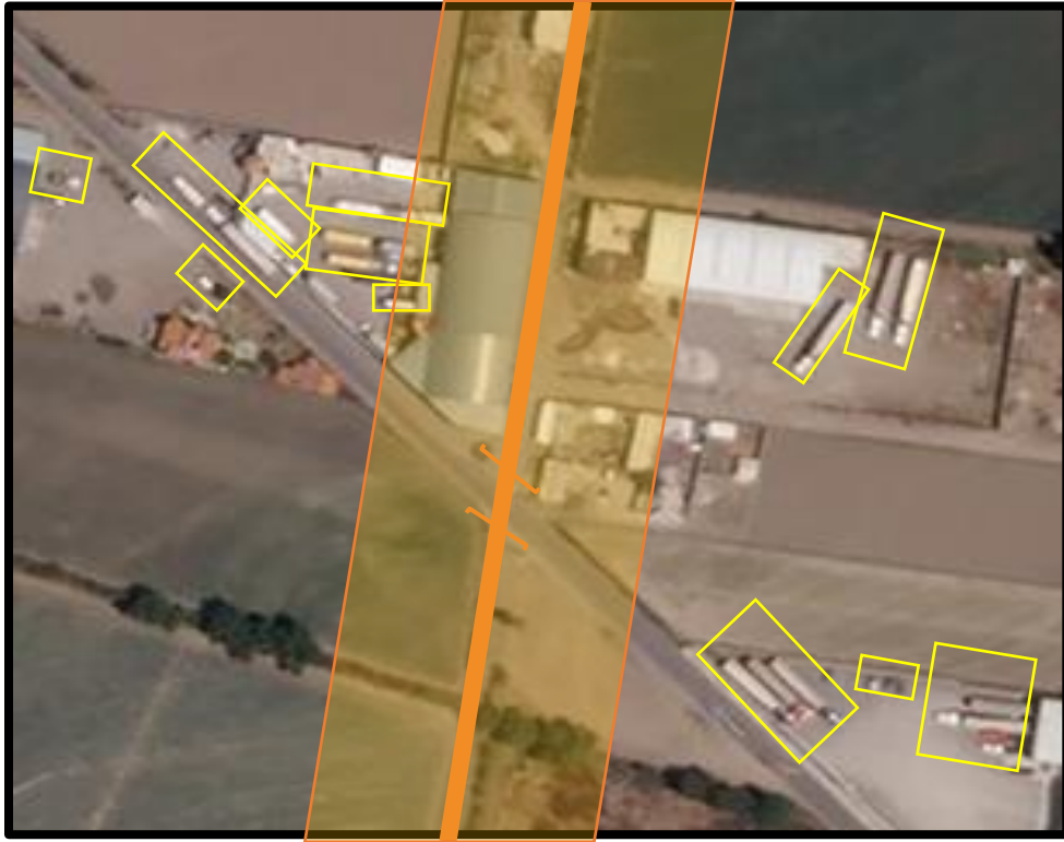
Figure 1. Identification of Vehicles and Mechanical Threats on or near a Right of Way
