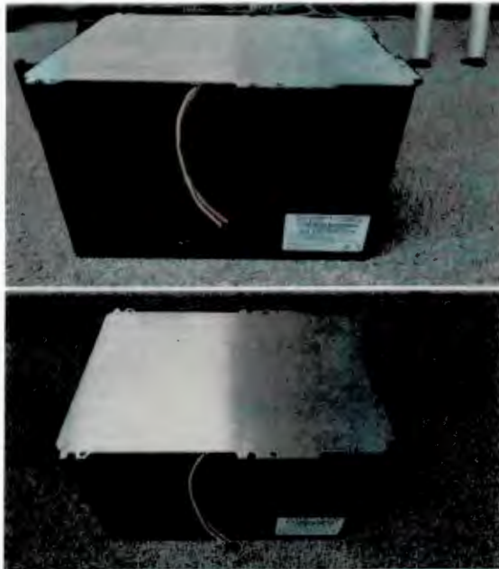
Figure 2: Yeti 3000 Battery Pack, 3074 Wh Battery LG M26 2.6Ah Cells, shipped as UN 3480
