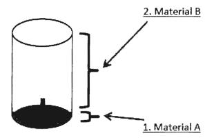
When used, the loose Material B pours easily from the tube while Material A remains in the grid inside the tube. To loosen/remove Material A, the bottom of tube must be tapped.
