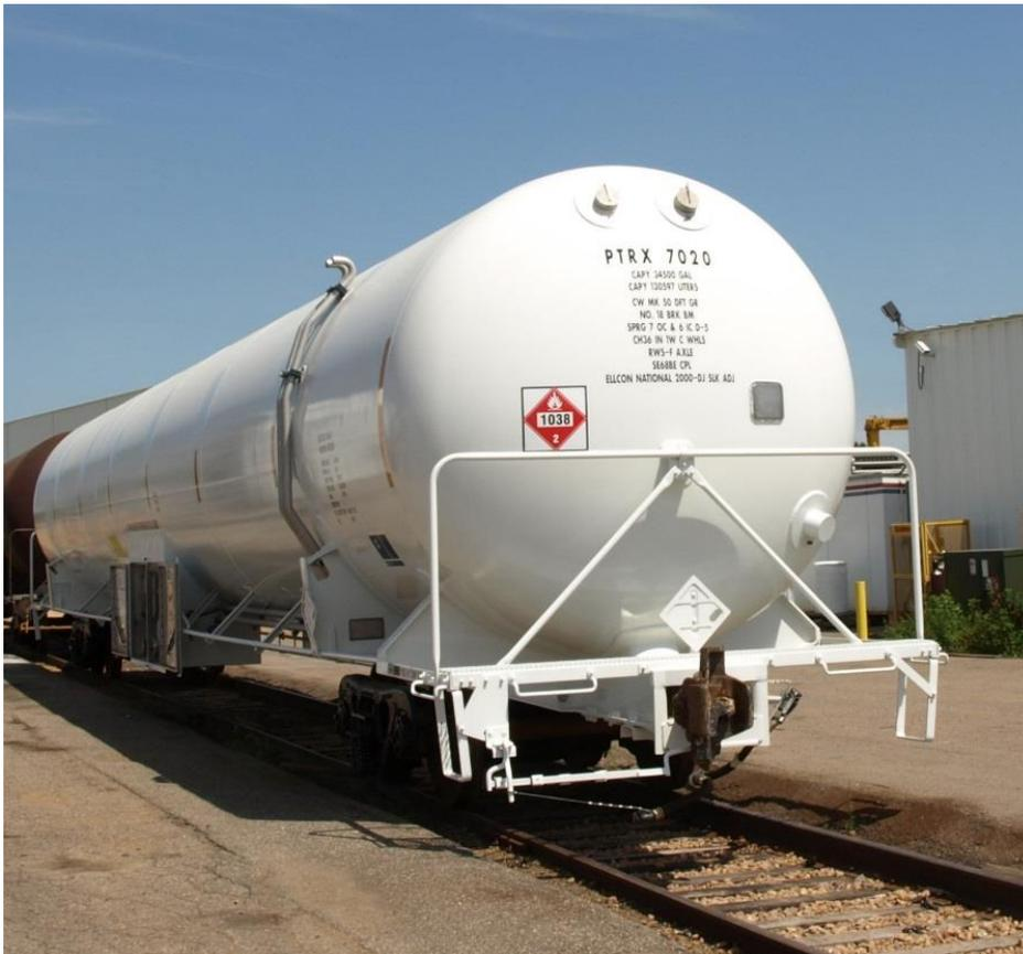
**Figure F.6 DOT 113 Rail Tank Car (Back End)**
