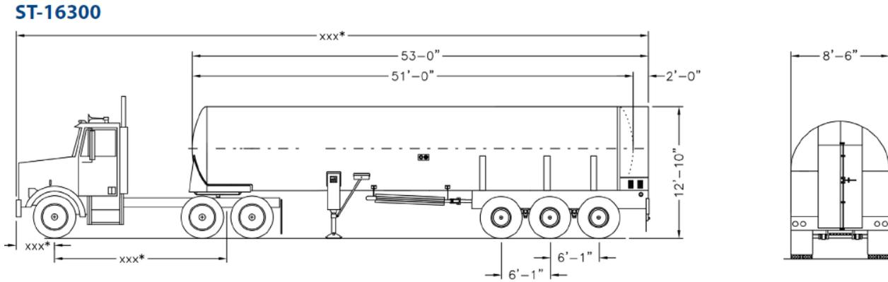
**Figure F.2 Cargo Trailer Specifications—ST-16300**
