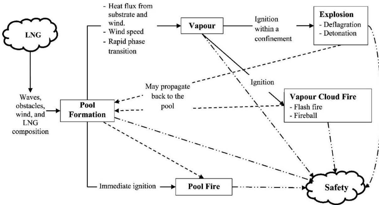
**Figure 6.10 LNG Release Consequence Diagram**
