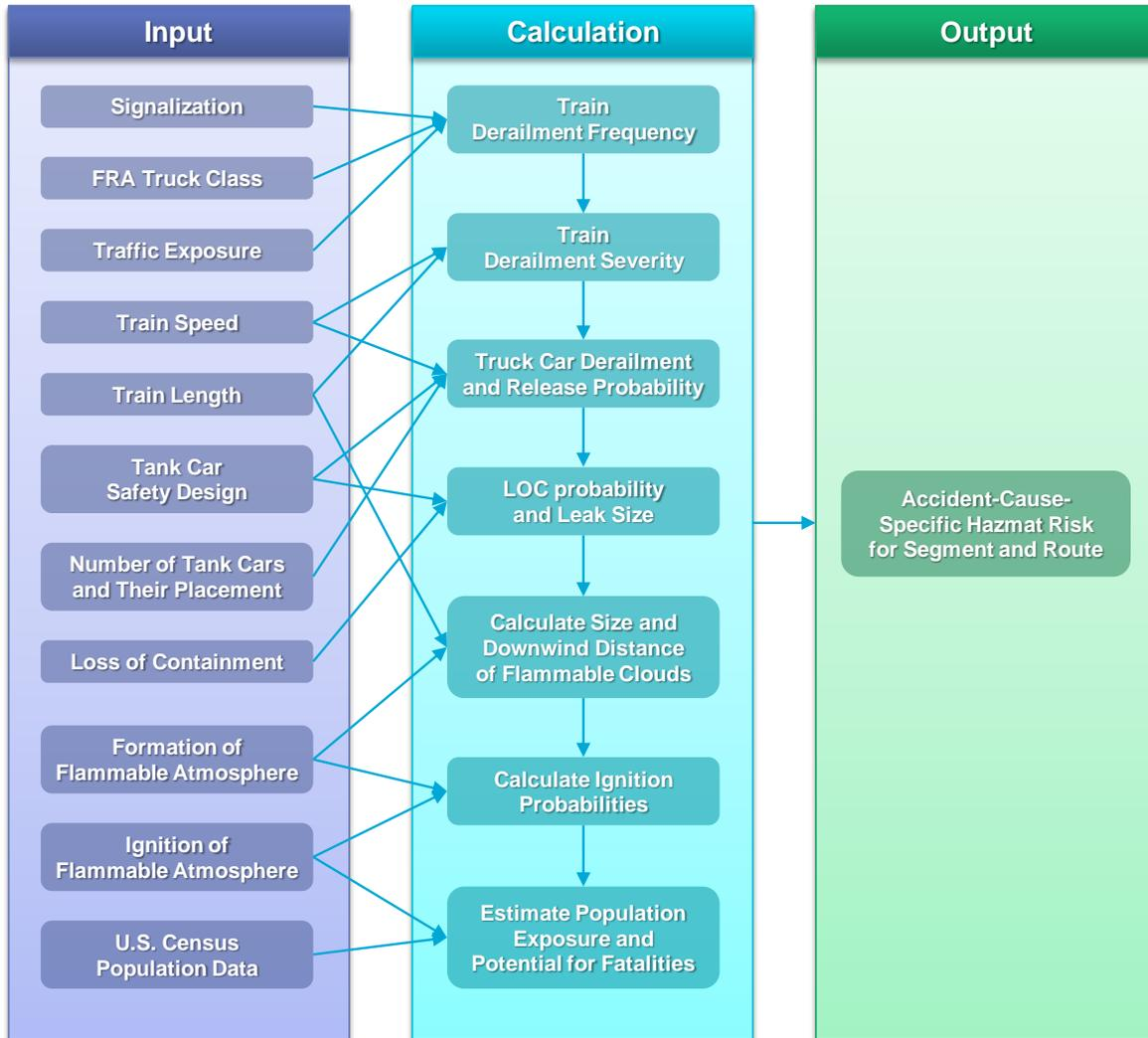
**Figure 6.2 Risk Inputs, Calculations, and Outputs for Rail LNG Transport**
