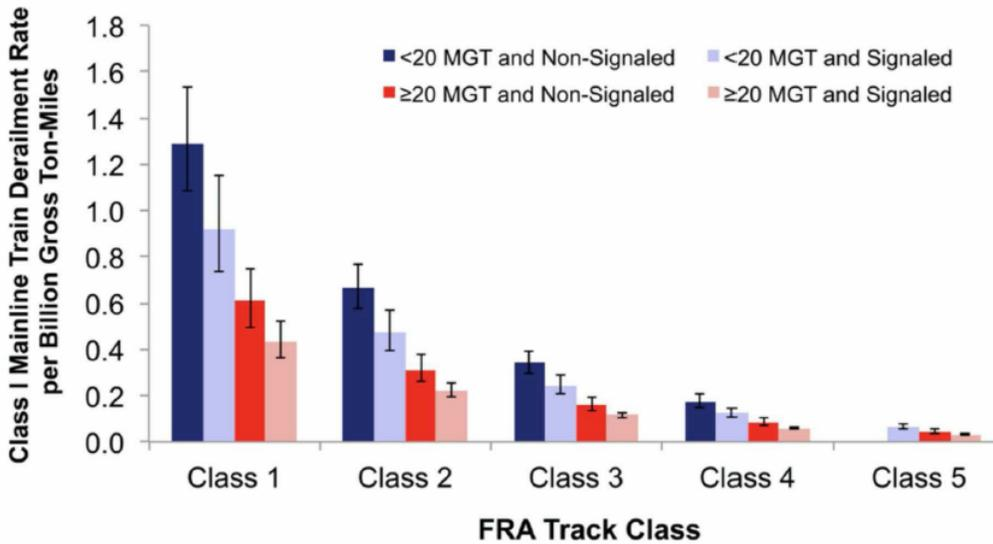
**Figure 6.4 Estimated Train Derailment Rates By Track Class**
