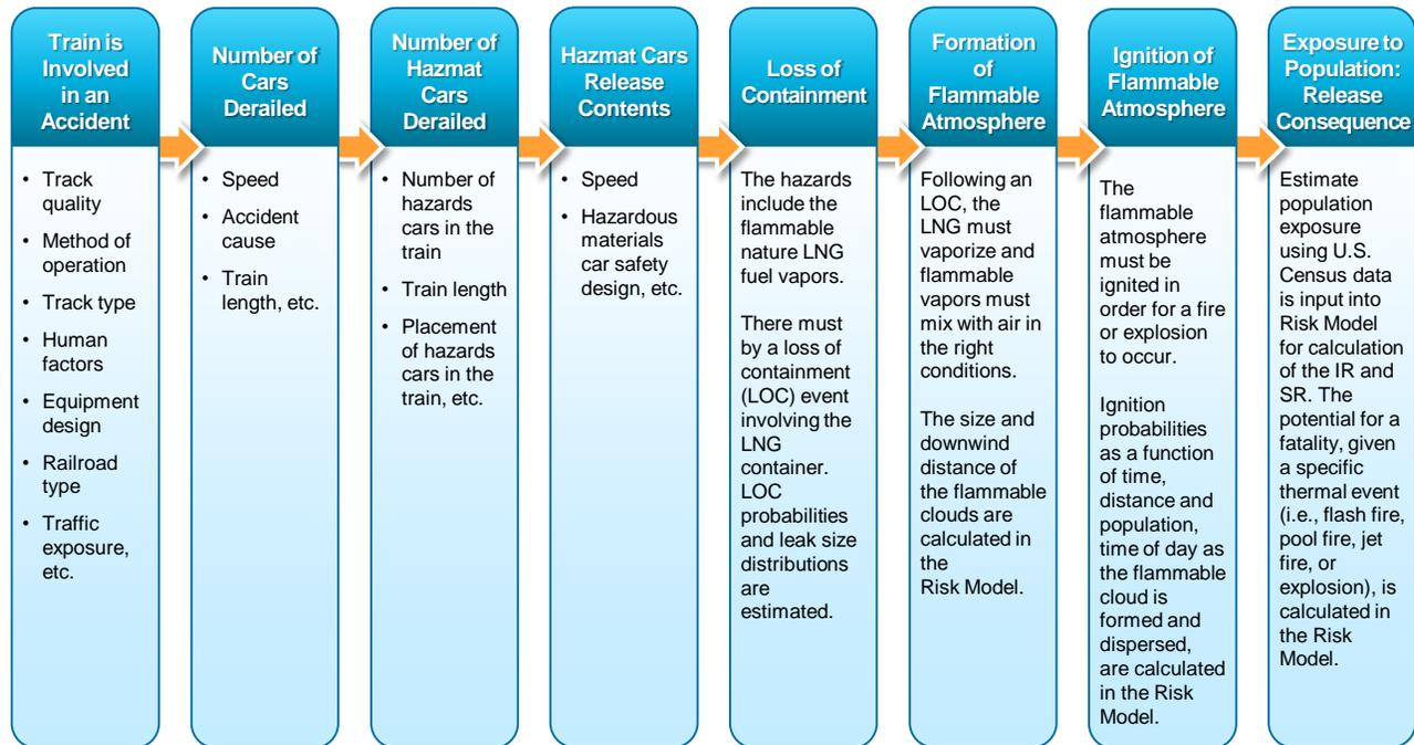
**Figure ES-3 Rail LNG Event Chain Diagram**
