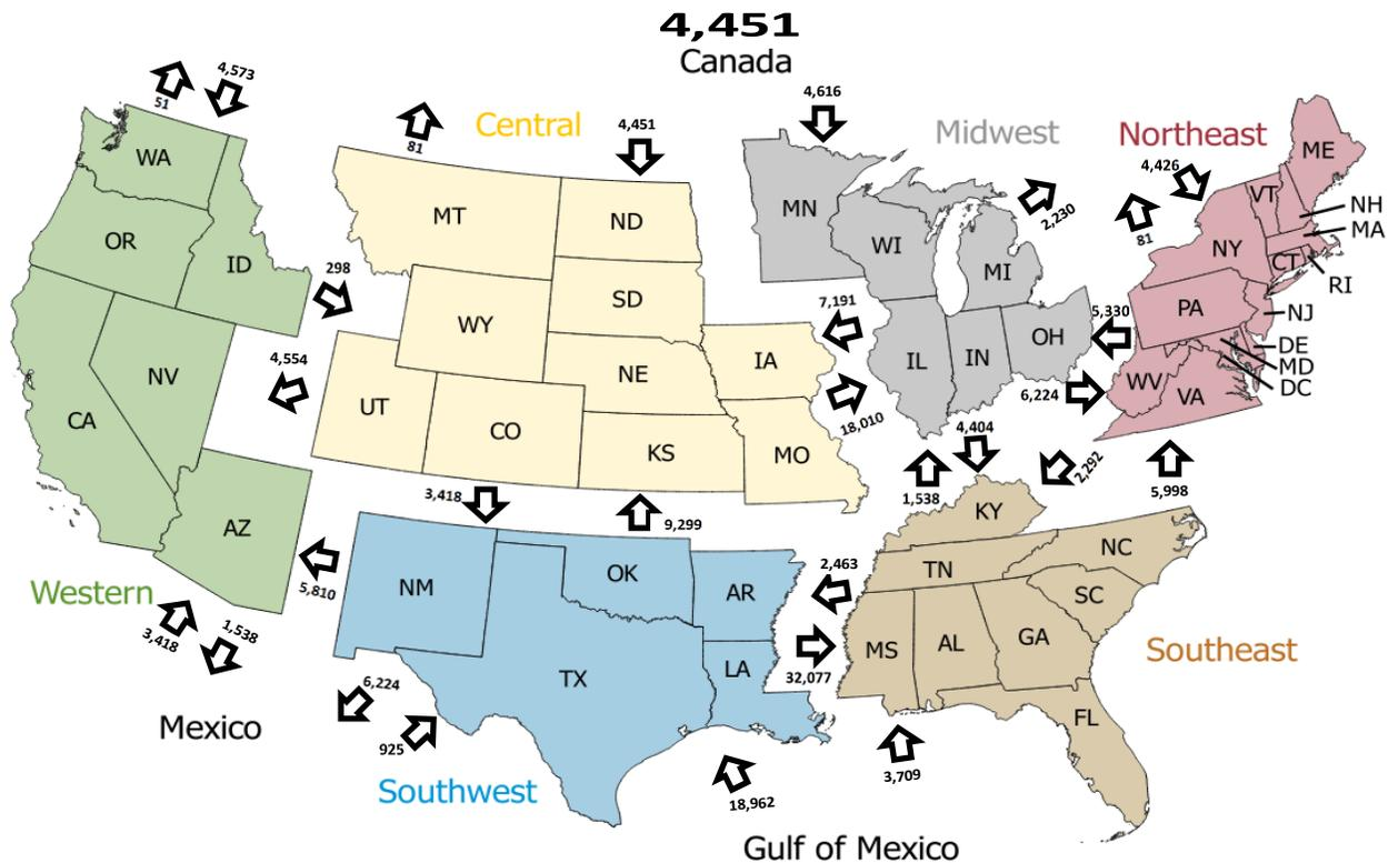
**Figure 4.13 U.S. Pipeline Capacity between EIA Regions**
