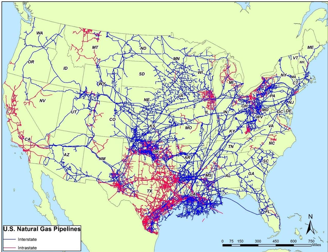
**Figure 2.1 U.S. Natural Gas Pipeline Network**
