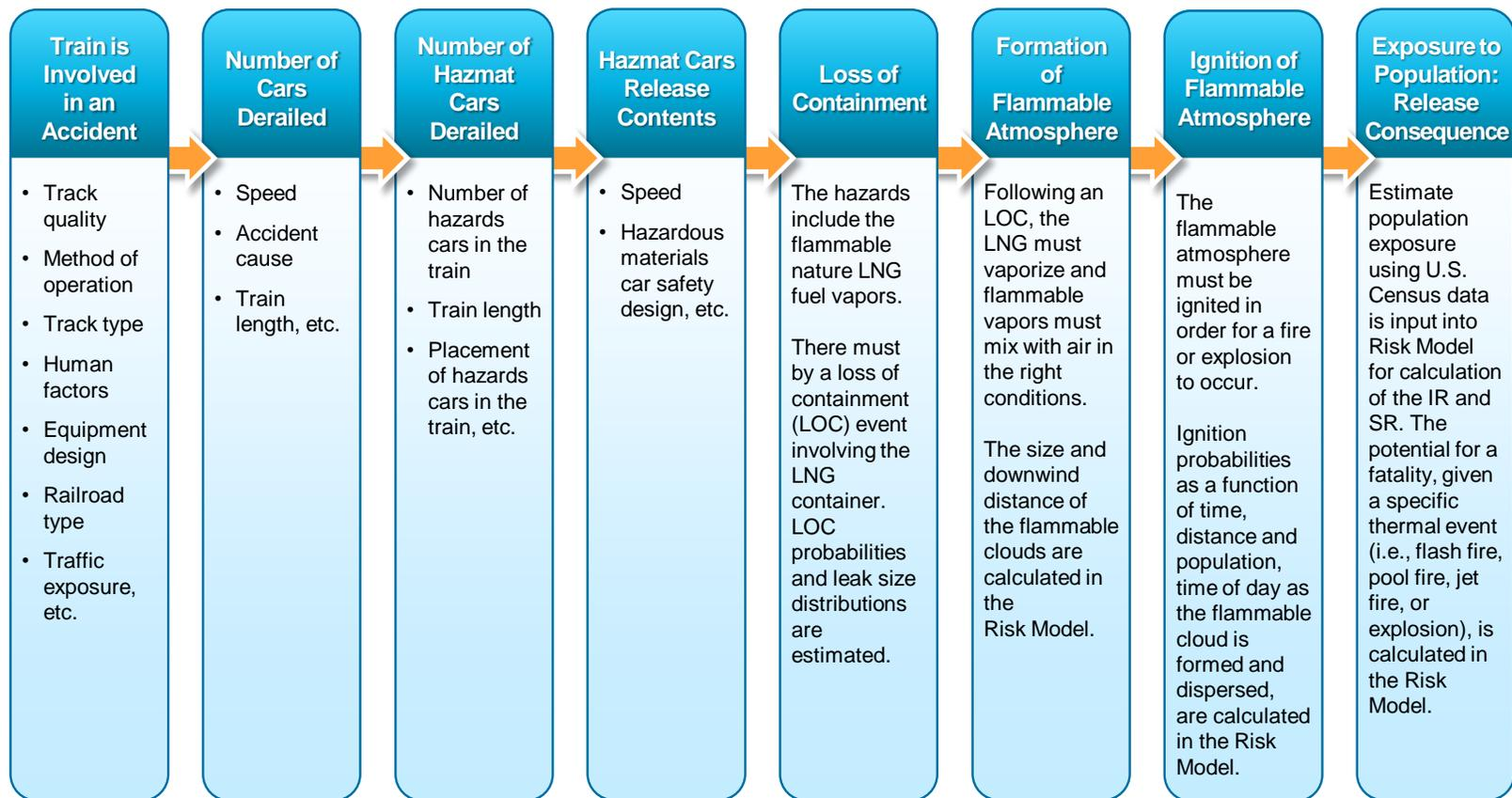
**Figure 6.1 Rail LNG Event Chain Diagram**
