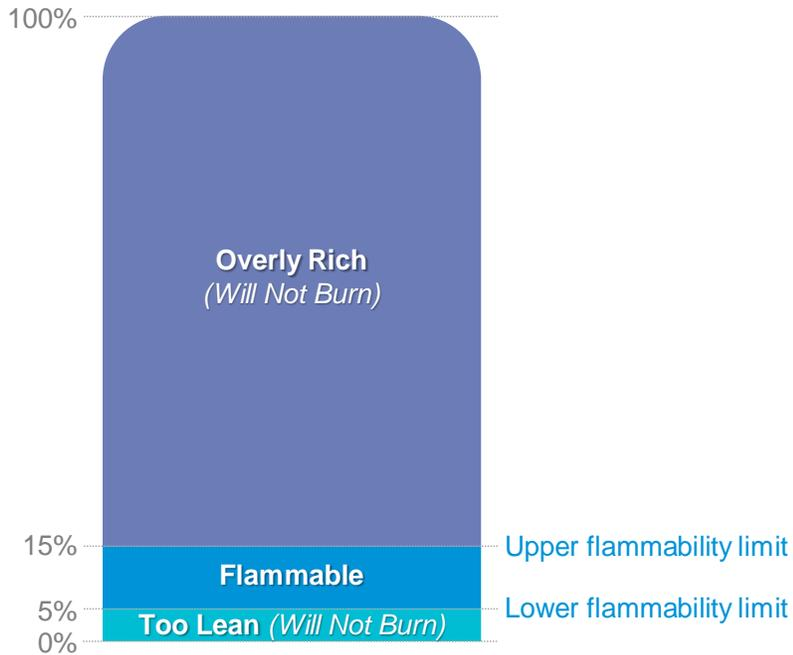
**Figure 6.9 LNG Flammability Range**
