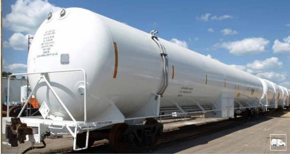
**Figure F.5 DOT 113 Rail Tank Car (Front End)**
