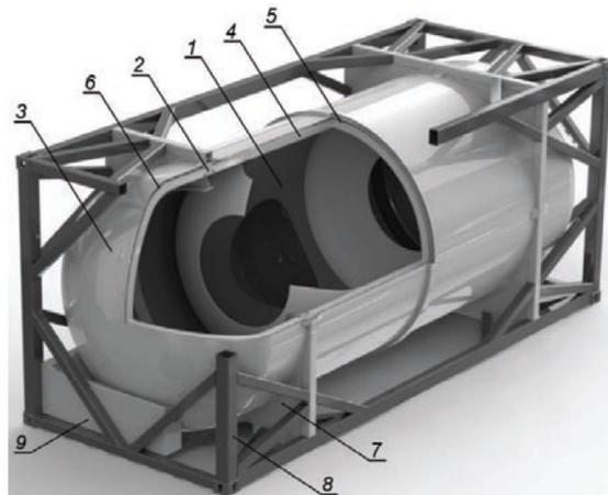
Fig. 1. Model of the LNG tank container for LNG transportation and storage, tank type I and II : 1 – inner tank, 2 – inner supports made of plastic materials, 3 – outer tank, 4 – insulation, 5 – radiation shields, 6 – the vacuum, 7 – outer supports, 8 – container frame, 9 – fittings
