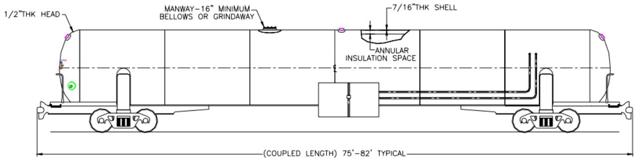
**Cutaway Drawing of Tank Car
