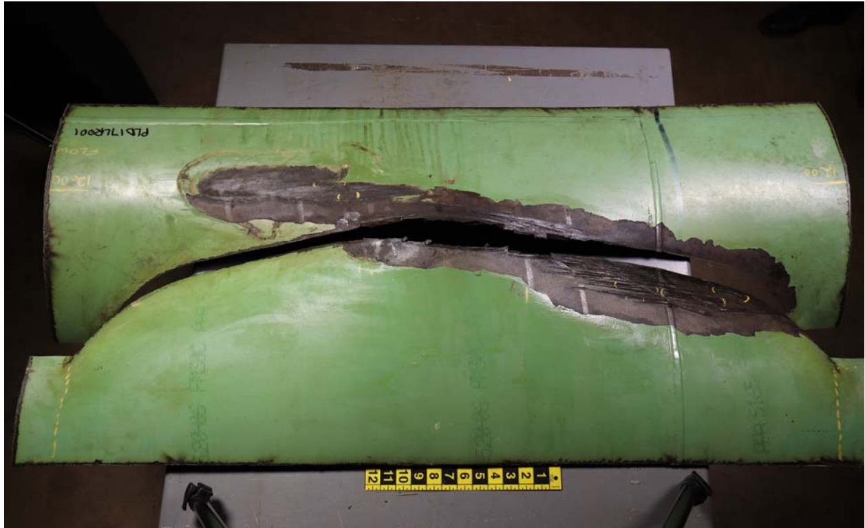
NTSB Photo – Additional Gouges Adjacent to Rupture Opening
