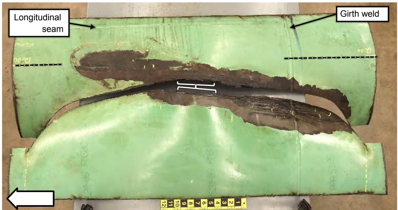
Copied from the NTSB Metallurgical report: Figure 13. Overall view of the exterior surface after sectioning with the two sides of the fracture placed in close proximity. Dashed lines indicate the 12 o'clock position, and unlabeled brackets indicate the fatigue crack region.
