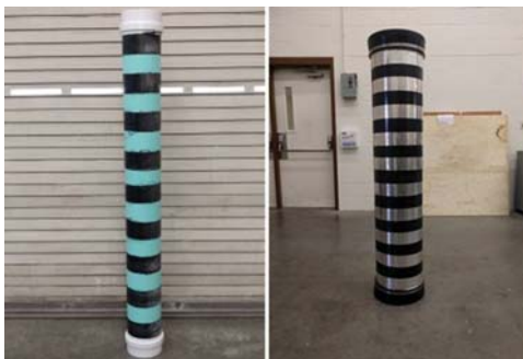
Figure 3. PVC pipe with CFRP rings and GFRP pipe with Aluminum rings.
