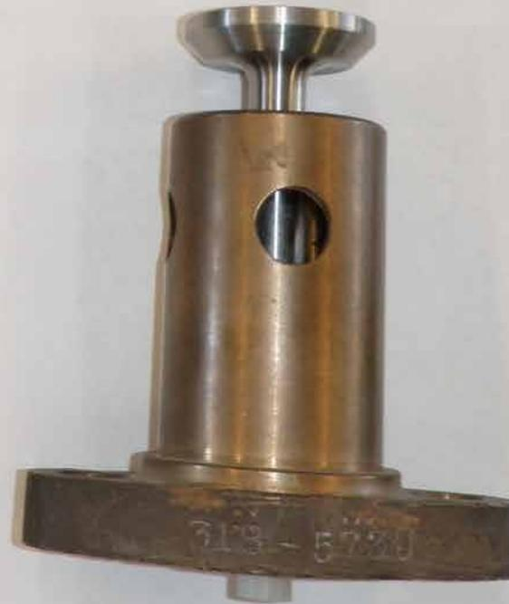
The air start valve is operated directly from the cam of the engine. As the valve opens it allows air to flow to the air start check valve. Air pressure at 250 psig overcomes the spring tension on the air start check valve and air enters the cylinders. The air pressure causes the cylinders to begin to rotate.
