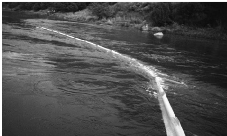
Figure 3-3. Boom submergence failure in swift current.
