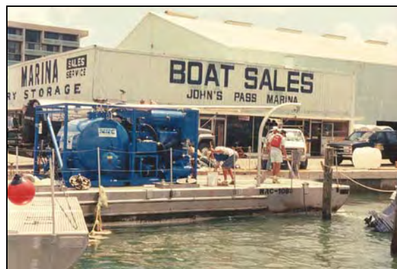
Figure D.1ba Special Purpose Vacuum Recovery System
