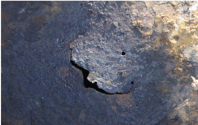
Figure 3 Failed Strainer (external view)
