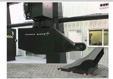
Figure 3-5. Photograph of the Lockheed Martin LaserUT<sup>™</sup> system testing a complex composite duct.
