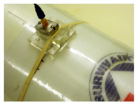
*Figure* **4-6***. Close-up picture of the angle beam wedge on tank*
