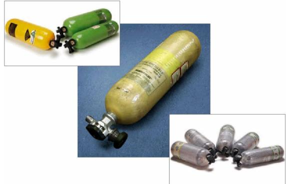
Figure 2-1. Compressed gas cylinders: fiberglass (upper left), Kevlar (center), and carbonwrapped (lower right). Fiberglass and carbon cylinders were used for the initial feasibility study; Kevlar cylinders, although not used during this phase of study, were acquired for followon work.
