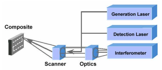
Figure 3-4. Schematic of a laser ultrasonic system.
