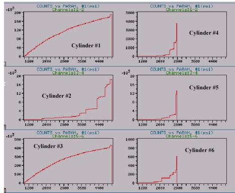
Figure 4-2. Cumulative AE counts vs. pressure for the test cylinders (note the different scales used in the graphs).
