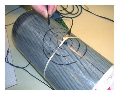
*Figure 4-7. Graphite epoxy tank showing source and receiver probe placements.*
