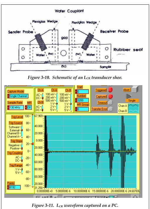
example of a transducer shoe for  $L_{CR}$  inspections is shown in Figure 3-10.
