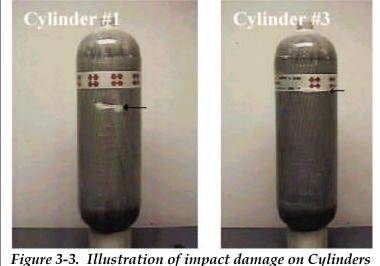
Figure 3-3. Illustration of impact damage on Cylinders 1 and 3.
