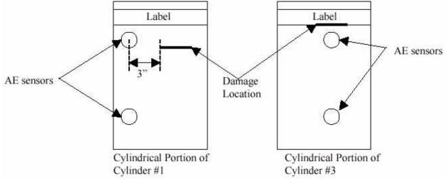
Figure 3-6. Illustration of sensor location on two of the damaged cylinders.
