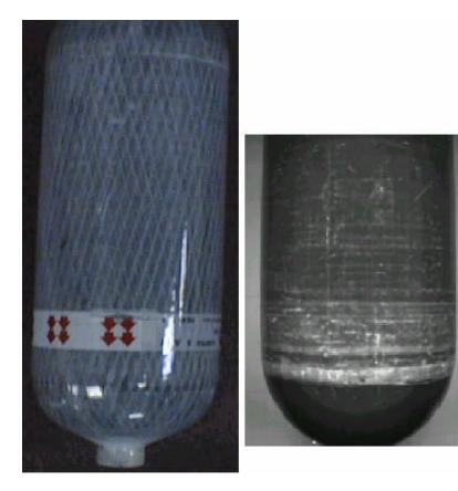
Figure 4-4. Comparing visible and thermographic indications of impact damage in Cylinder 3 (IL35250). In contrast with the thermograph of Cylinder 1, which has a similar severe impact anomaly, the impact damage in Cylinder 3 is not as clearly visible as in Cylinder 1.
