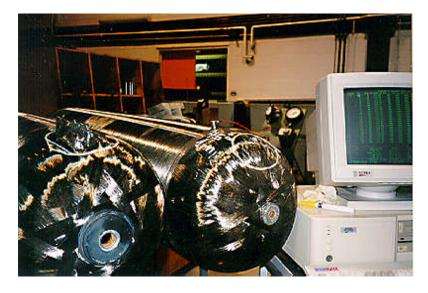
Figure 3-7. Assessment of composite compressed natural gas cylinders following drop tests, from work conducted in 1999 for Transport Canada by Powertech Laboratories. The cylinder on the right is undergoing acoustic emissions testing to assess damage. The one on the left has been pressurized to failure.
