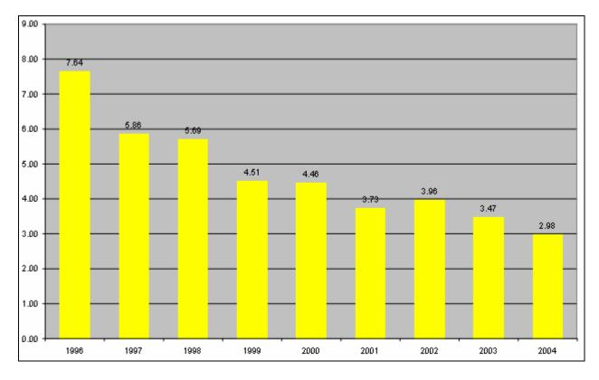
Figure 6: Minnesota Gas Distribution Excavation Damages per 1000 Tickets
