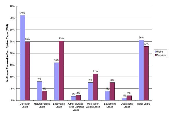
Figure 4: 2004 Leaks Removed by Causes and System Types
