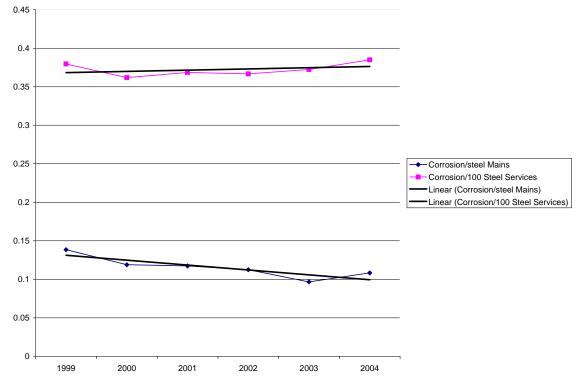
Figure 10: Trends in Corrosion Leaks Removed in Steel Main Miles and Steel Services
