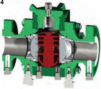
Make Sure all seals are in place and in good condition on the closure and in the body. Replace the closure and verify the vent fitting and body fittings are closed.
