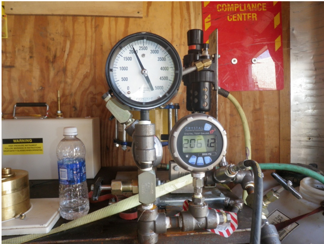
View of Pressure Gauge During Hydrostatic Test of Replacement Pipe
