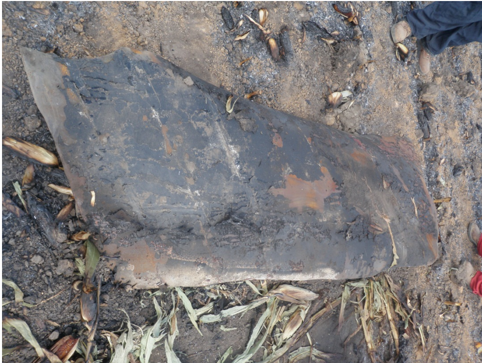
Exterior View of Piece # 2 (Containing Failure Origin)
