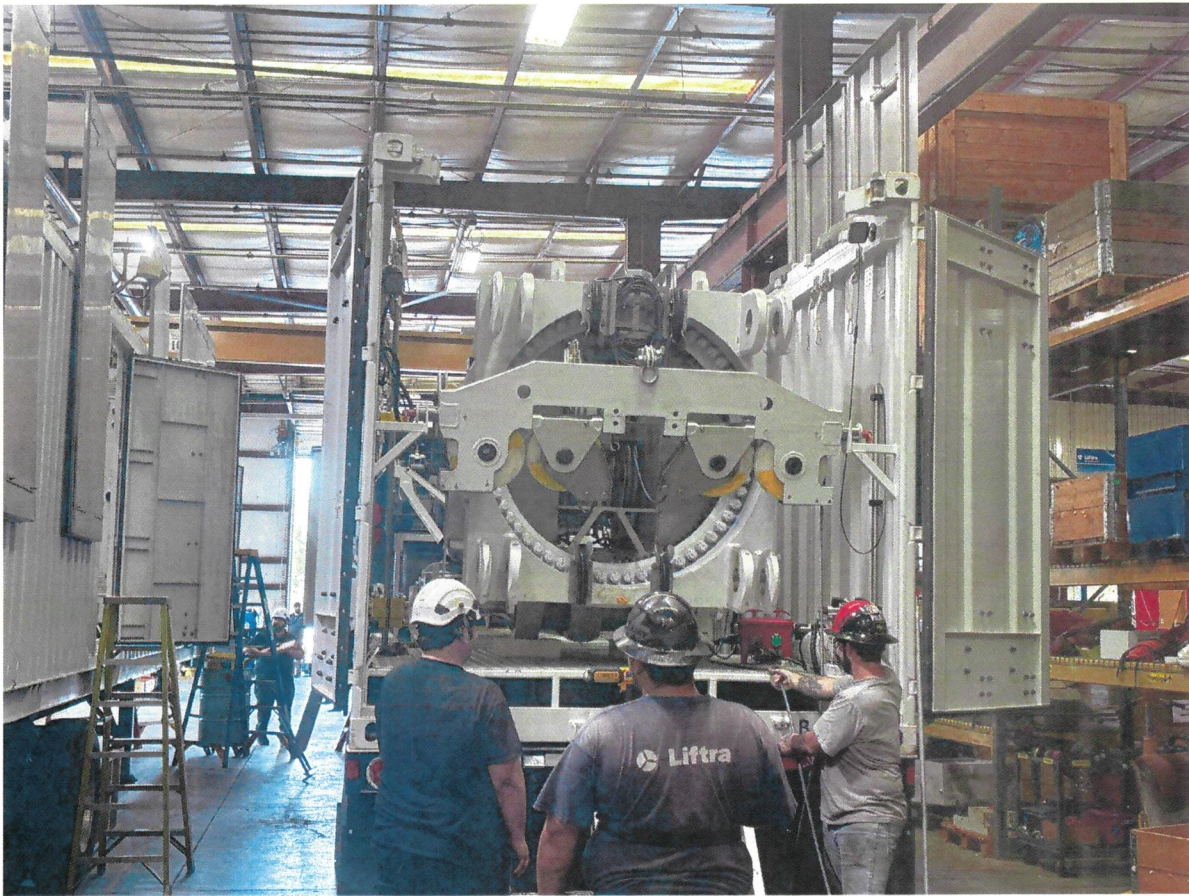
Exhibit Figure A-2. Rear view with the LT1200 nacelle system stowed inside the dedicated enclosure for transport. Dedicated geometry and restraint features are visible around the crane.
