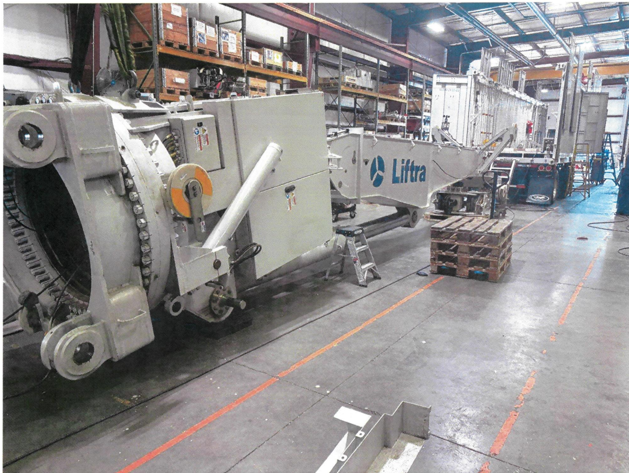
Exhibit Figure A-3. LT1200 nacelle system outside the enclosure during workshop activity, illustrating the industrial machine that is stowed in the enclosure for transportation and deployed for wind-turbine operation.
