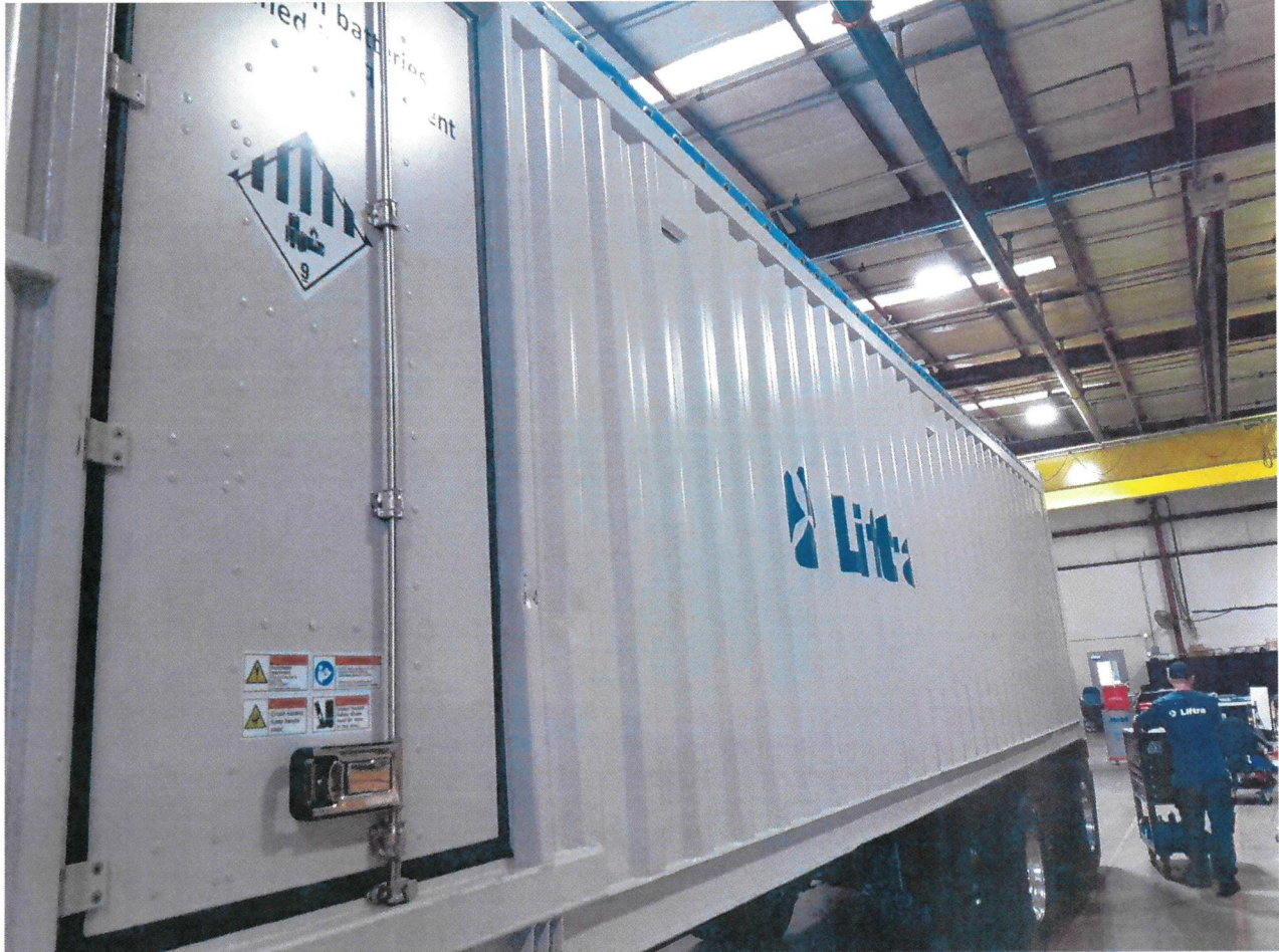
Exhibit Figure A-1. LT1200 dedicated enclosure positioned on a highway trailer, illustrating the normal transport form of the complete system.
