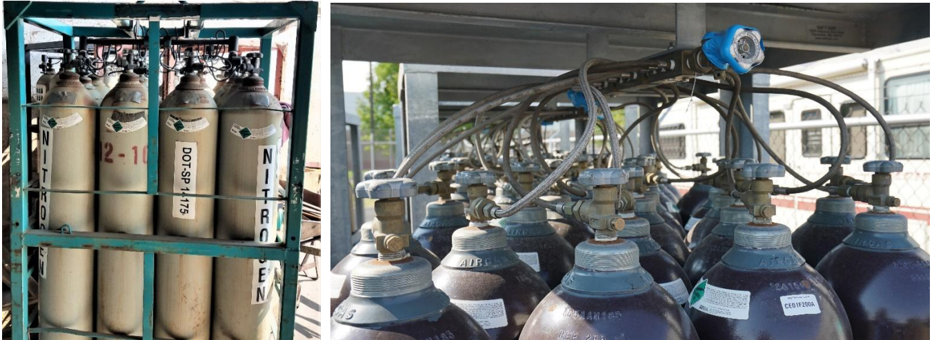
Compressed gas cylinders, with individual closures, manifolded together for transport.
