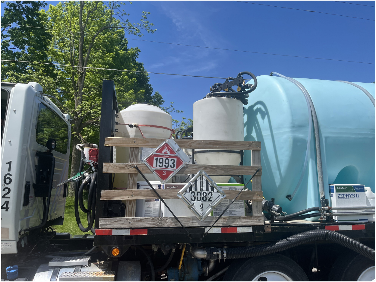
Front of truck showing the Green water tank and the 55-gallon "inductor tank"
