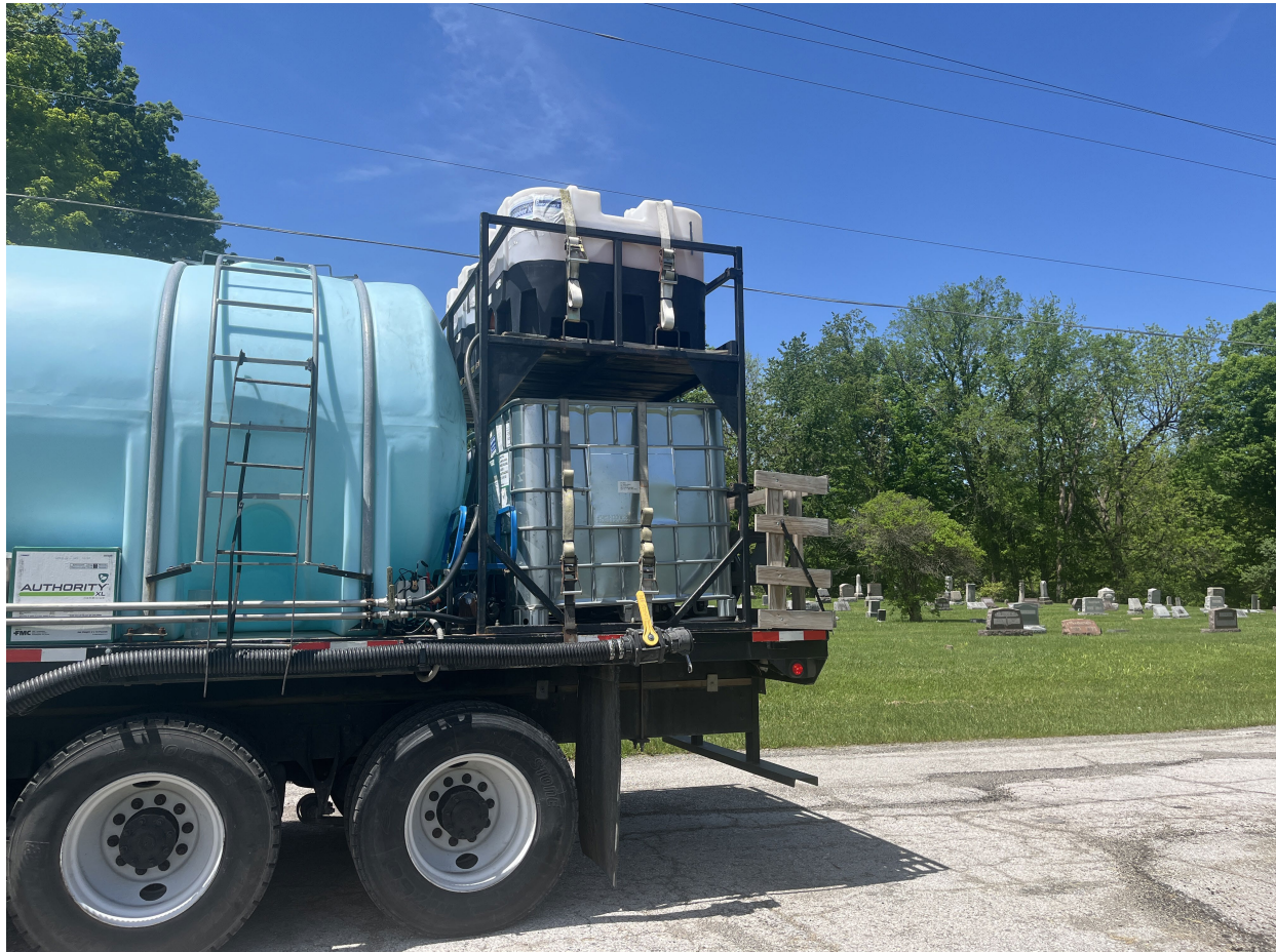
Rear of truck showing some of the IBCs and the discharge hose with the valve and yellow shut off handle
