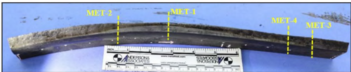
Figure 33 – Overall view of the seam-side panel containing the fatigue crack detailing the locations of the sections cut for metallographic examination.
