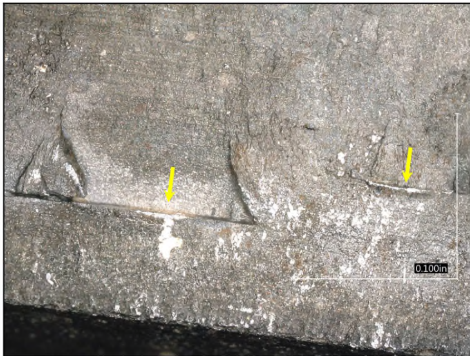
Figure 16 – Low magnification view of several secondary crack-like features identified on the fatigued surface. The secondary cracks were oriented perpendicular to the fatigue crack growth direction. The secondary cracks appeared visually consistent with hydrogen induced cracking (HIC).
