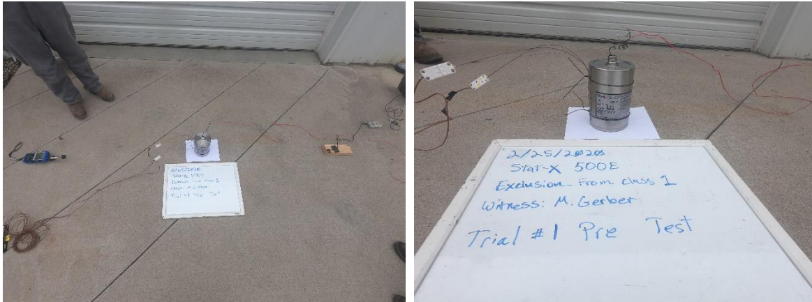
Figure 2: Basic Exclusion from Class 1 test setup, Stat-X 500E sample
