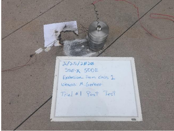
Picture 9: Stat-X 500E post-test
