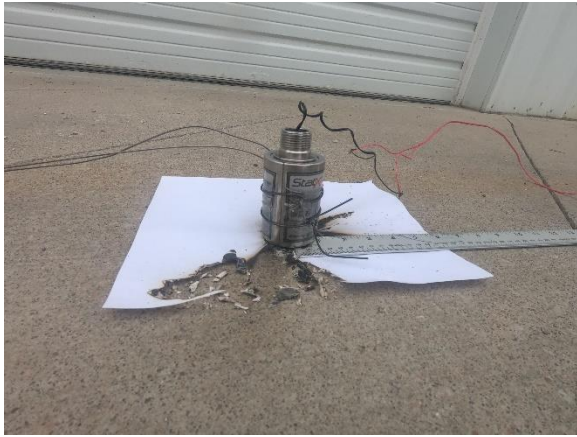
Picture 3: Stat-X 30E post-test
