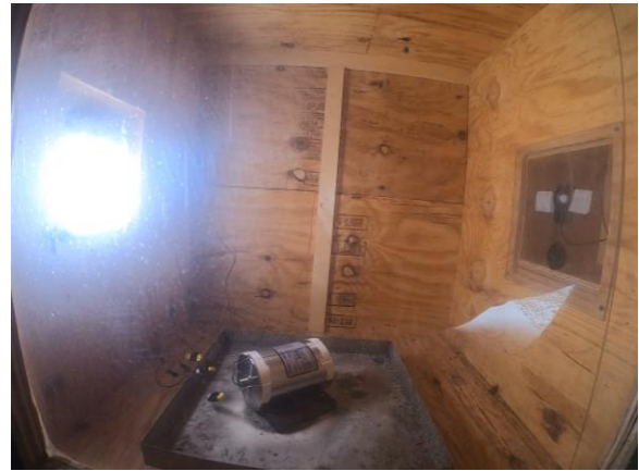
Picture 10: Stat-X 500E Smoke Box pre-Test
