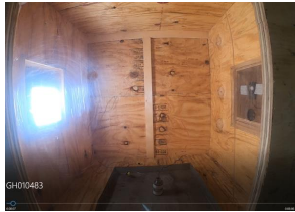
Picture 4: Stat-X 30E smoke box setup
