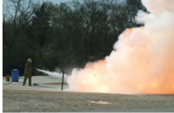
If the spill occurs outside a confined area, the burning pool fire is free to flow based on topography and the geometry of the spill. Spraying water on an LNG pool only increases the vaporization rate and intensifies any fire; spraying a gallon of water will vaporize about two gallons of LNG.
