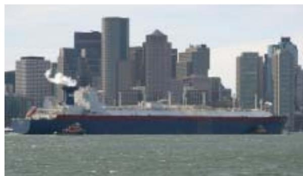
LNG ships vary in size from 20,000 to over 145,000 cubic meters cargo capacity but most modern vessels are between 125,000 and 140,000 cubic meters capacity (58,000 to 65,000 tons). A typical modern LNG ship has a length of about 975 feet (300 m), width of about 140 feet (43 m), draft of about 39 feet (12 m) and is capable of sailing at speeds of up to 21 knots. A new LNG ship will cost about \$170 million.<sup>10</sup>
