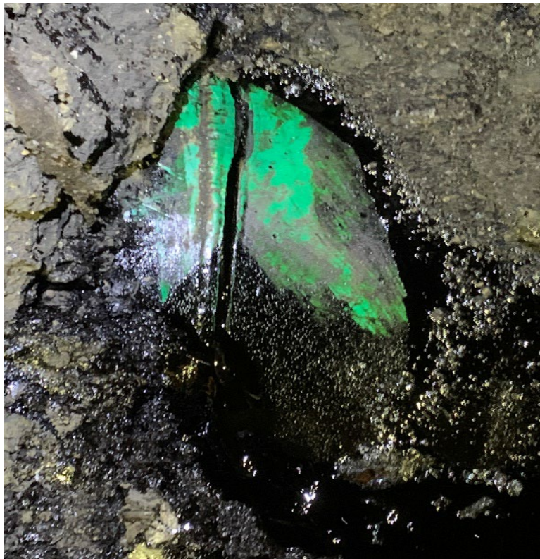
Figure 4. Initial View of Failed Girth Weld Exposed.
