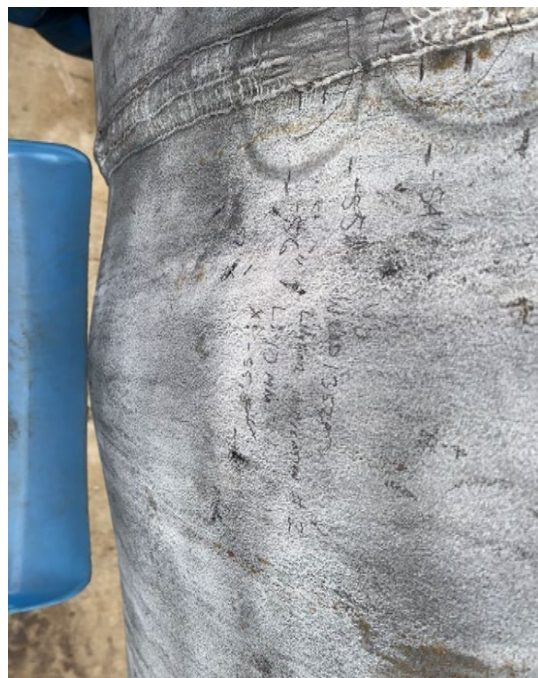
Figure 11. Sandblasted Pipe with Mag Particle Contrast Paint Applied. The Bulge is Located at the 6:00 Position.
