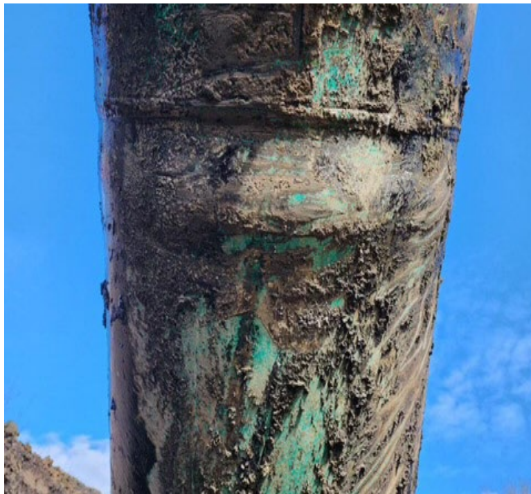
Figure 5. The Compression Stress Bulge in the 6:00 Position. This Single Compression Point Caused the Pipeline to Bulge out About 1/2-Inch from the Normal Plane of the Pipeline. This Photo Was Taken After the Failure in December 2022 Looking Up.
