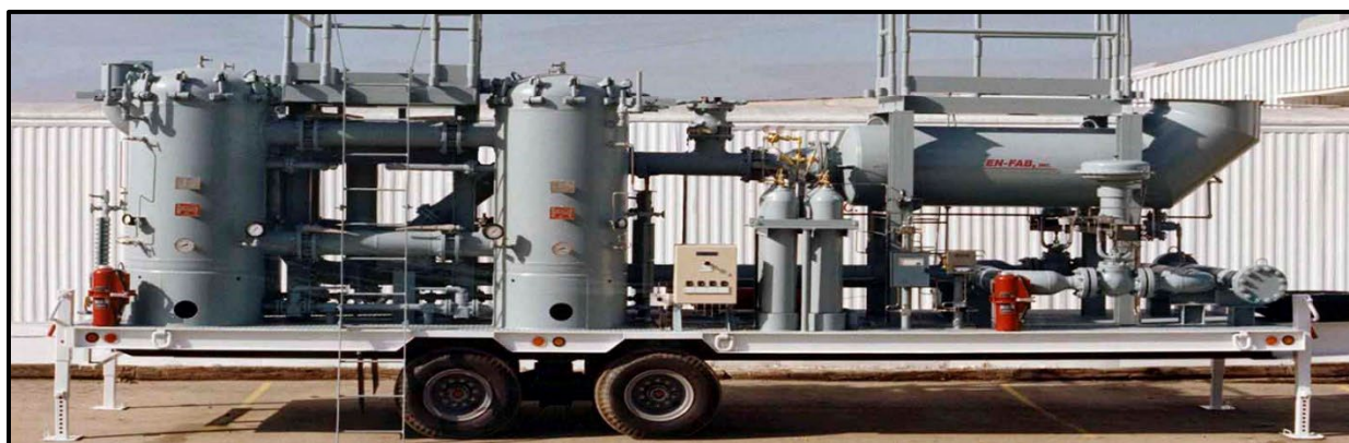
Figure 40: Modularized Trailer Unit for Pipeline Blowdown (Courtesy of EN-FAB, Inc.)
