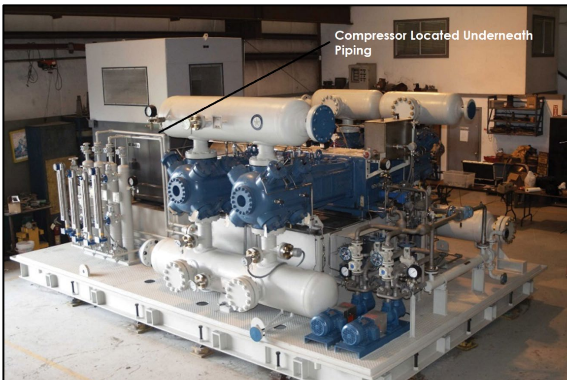
Figure 16: Packaged Medium-Speed, Short-Stroke Compressor Unit (Courtesy of the Ariel Corporation)
