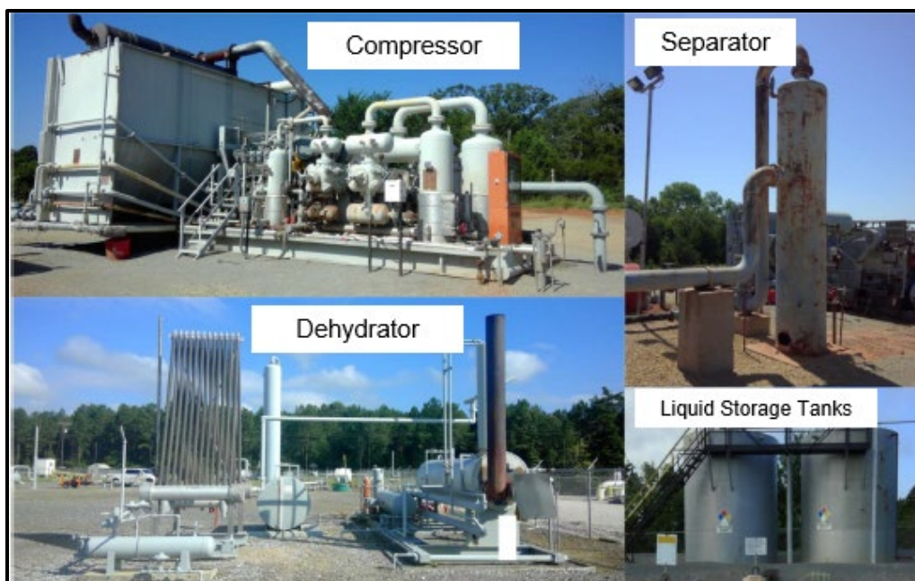
Figure 2: Typical Gathering Station Components (Courtesy of the Energy Institute at Colorado State University)
