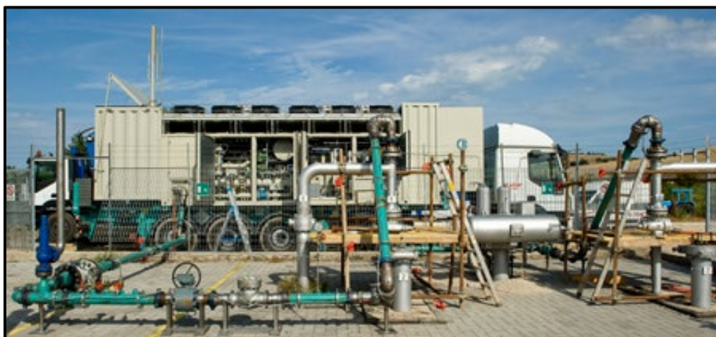
Figure 33: Mobile Electric Compressor (Courtesy of the EDF)
