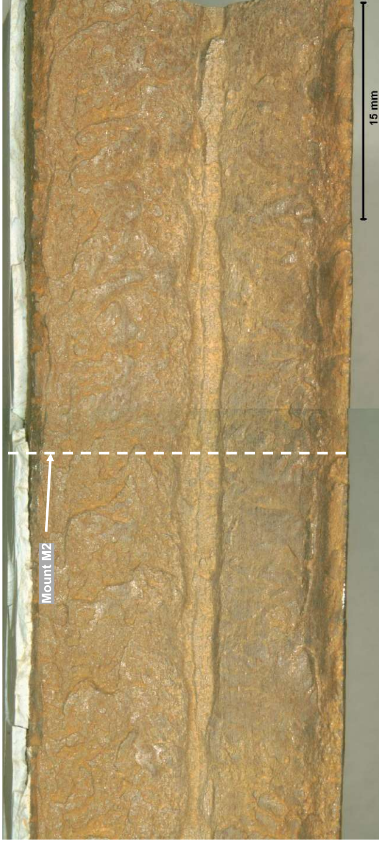
Figure 31. Light photomicrograph of Sample S2 showing the fracture surface; area indicated in Figure 5. The figure shows where Mount M2 was removed. Examination in the SEM showed similar features as Sample S1, with areas of smearing and areas of dimples. There was no evidence of pre-existing flaws. The slight difference in this fracture surface from Sample S1 is that midwall is flatter in the thickness direction, which is obvious when looking at the fracture surface in cross-section in Mount M2 in Figure 16. As mentioned above, this sample was removed from this location along the fracture surface in order to examine the midwall vertical portion.
