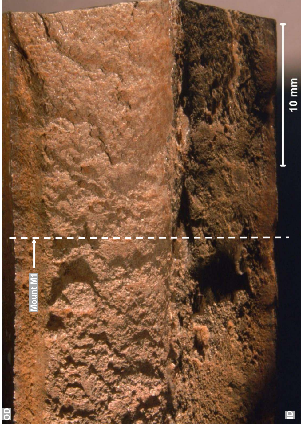
Figure 24. Light photomicrograph of Sample S1 showing the fracture surface; area indicated in Figure 23. The figure shows where Mount M1 was removed. The fracture surface is somewhat smooth from the ID surface to midwall, transitions to a rougher portion from midwall to just below the OD surface, and then the remaining portion adjacent to the OD surface is similar to the portion adjacent to the ID surface.
