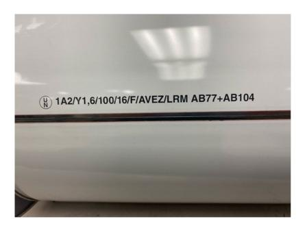
You will notice the tested gross weight of the package is indicated as 1,6. The are mean this to indicate that it was tested and certified to 1.6 kg. However, they have used the European indication for a decimal place.
