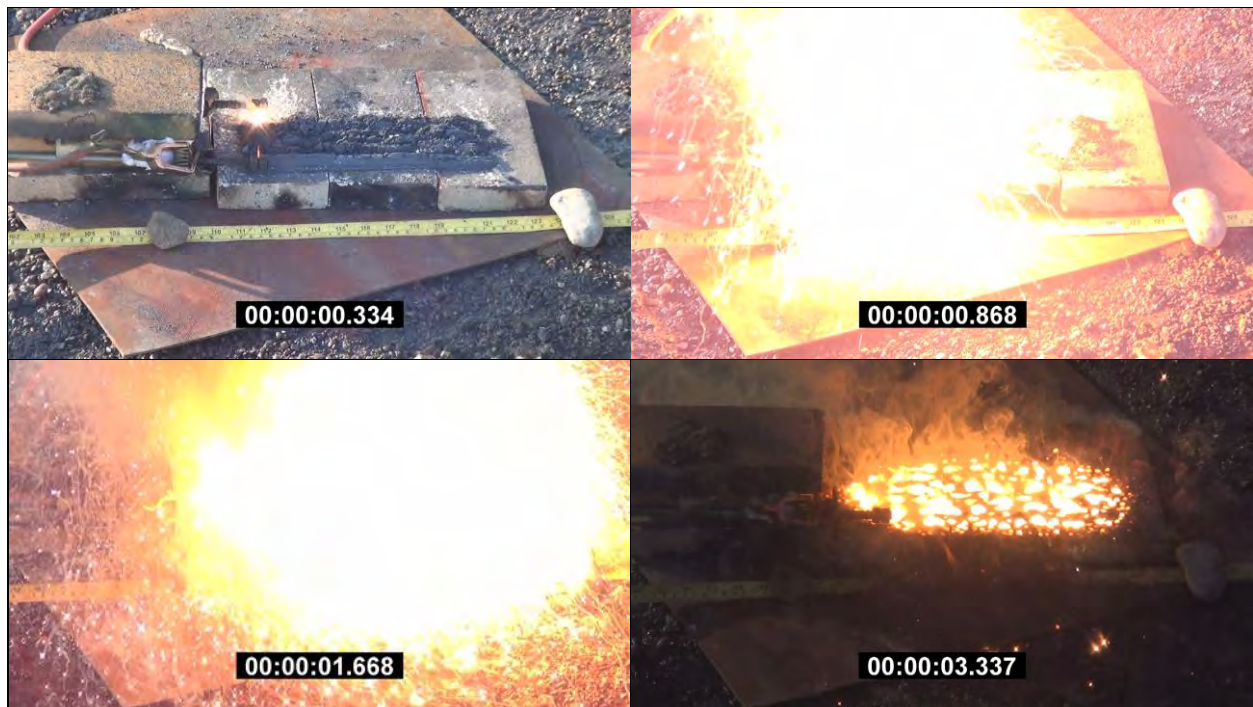
Photo 135: Large-Scale Readily Combustible Test Results - Hot Wire on Plate for Fine Al-CuO Thermite - Mix ID #4 (SMS mixed) with Ignition and Full Consumption over 1.3 seconds
