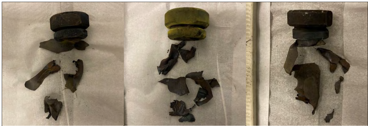
Photo 24: Koenen Test Results for SS #24 Al-Bi 2 O 3 , Trials 1 - 3 (left to right)
