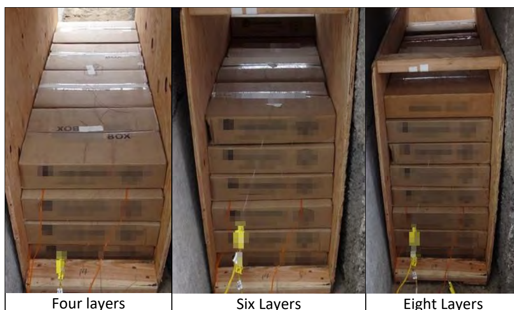
Photo 6: Simulated Pallet at Various Stages of Loading
