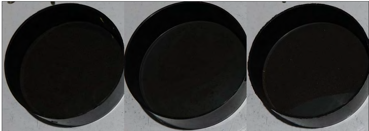
Photo 8: Small-Scale Mix ID #3B Thermite with Medium Ti and MnO 2 as Fine (left), Medium (center), Coarse (right)
