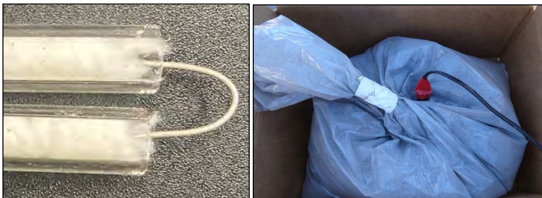
Photo 18: Insulated Nichrome Hotwire Igniter - typical
