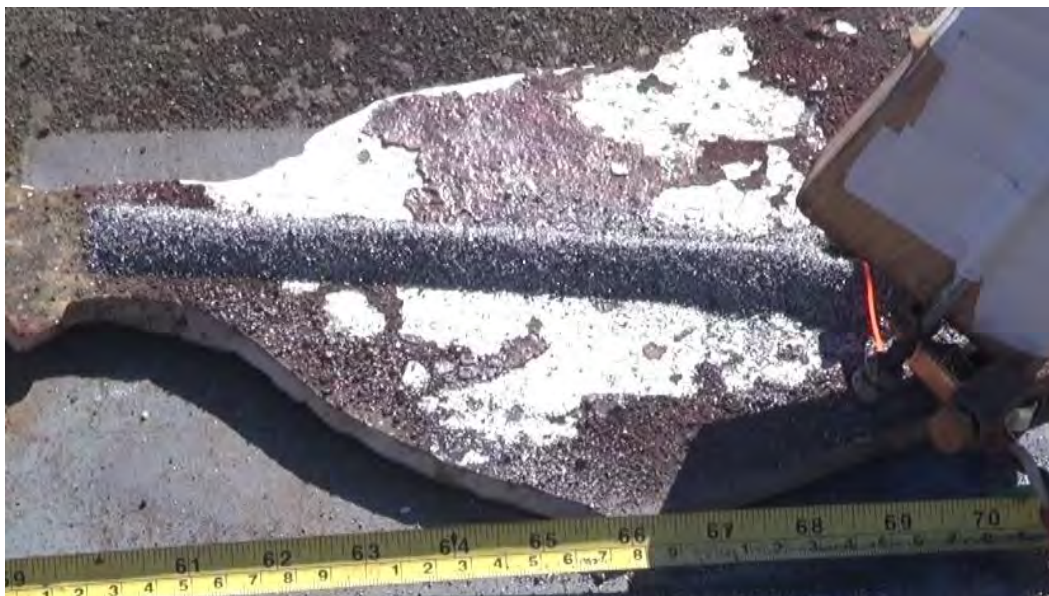
Photo 114: Readily Combustible Test Results - Hot Wire for Coarse Al-Fe 2 O 3 Thermite A - Mix ID #2 (Commercial) with No Reaction in 5 minutes
