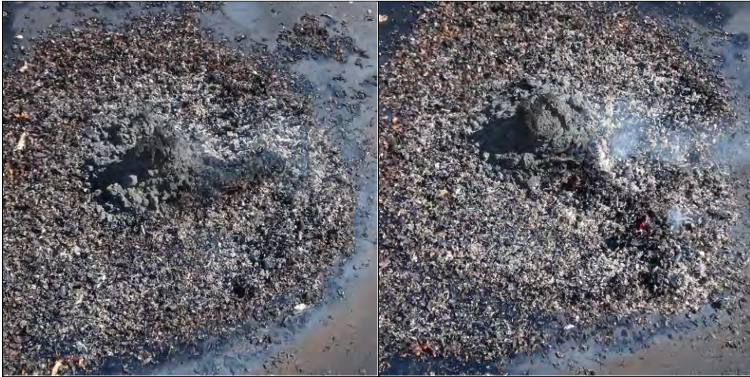
Photo 67: Small-scale Burning Test Results for Fine Al-Ni 2 O 3 Thermite - Mix ID #6 (SMS mixed)
