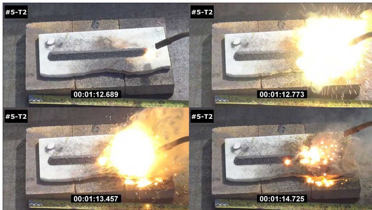
Photo 109: Readily Combustible Test Results - Gas Torch for Medium Al-CuO Thermite - Mix ID #5 (Commercial) with Ignition and Propagation (Trial 2)
