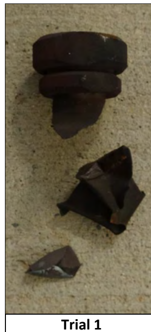
Photo A 3: LS #4-5-A10 Koenen Test Results
