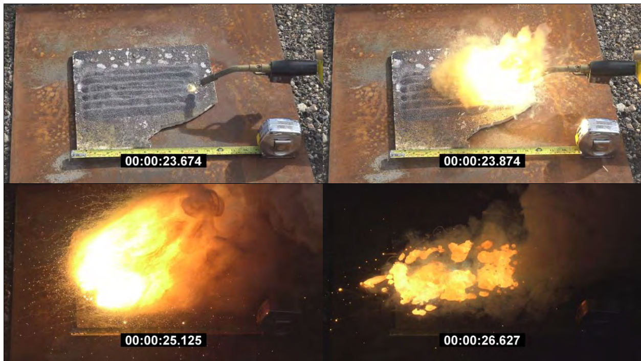
Photo 137: Large-Scale Readily Combustible Test Results - Gas Torch on Plate for Medium Al-CuO Thermite - Mix ID #5 (Commercial) with Ignition and Full Propagation over 1.5 seconds
