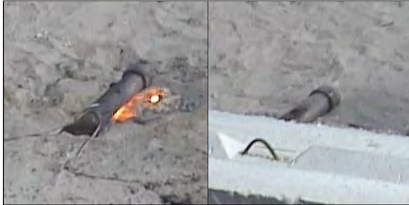
Photo 53: Internal Ignition Test Results for Coarse Al-Fe 2 O 3 Thermite B - Mix ID #3 (Commercial) - typical
