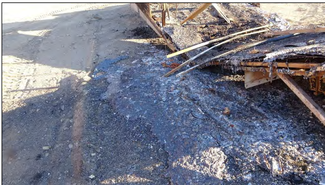
Photo 25: Box Truck Trailer Test Results - Solidified Pool of Thermite Slag, Left Side
