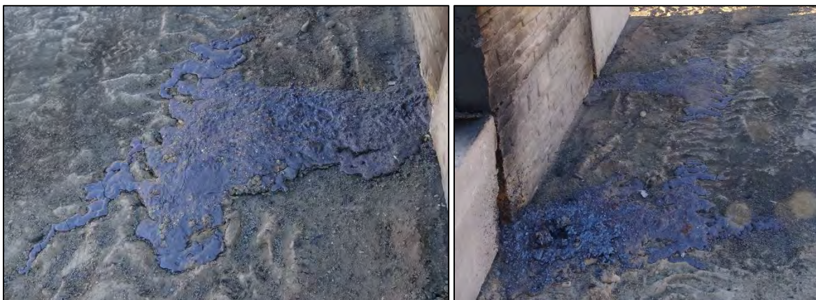
Photo 9: Solidified Pools of Thermite Slag (Fe and Al 2 O 3 ) from the Modified 800-lb Stack Test
