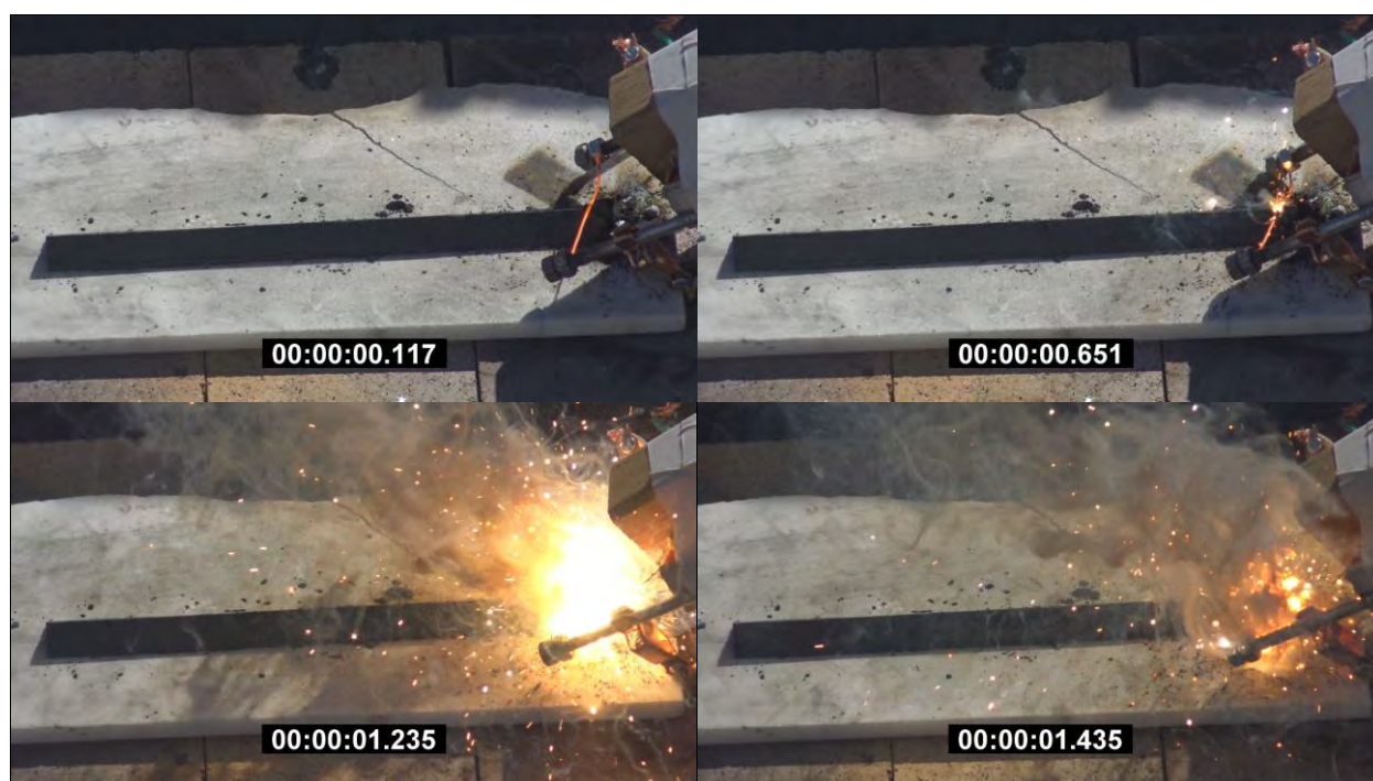
Photo 117: Readily Combustible Test Results - Hot Wire for Fine Al-CuO Thermite - Mix ID #4 (SMS mixed) with Ignition and Partial Propagation over 1.4 seconds
