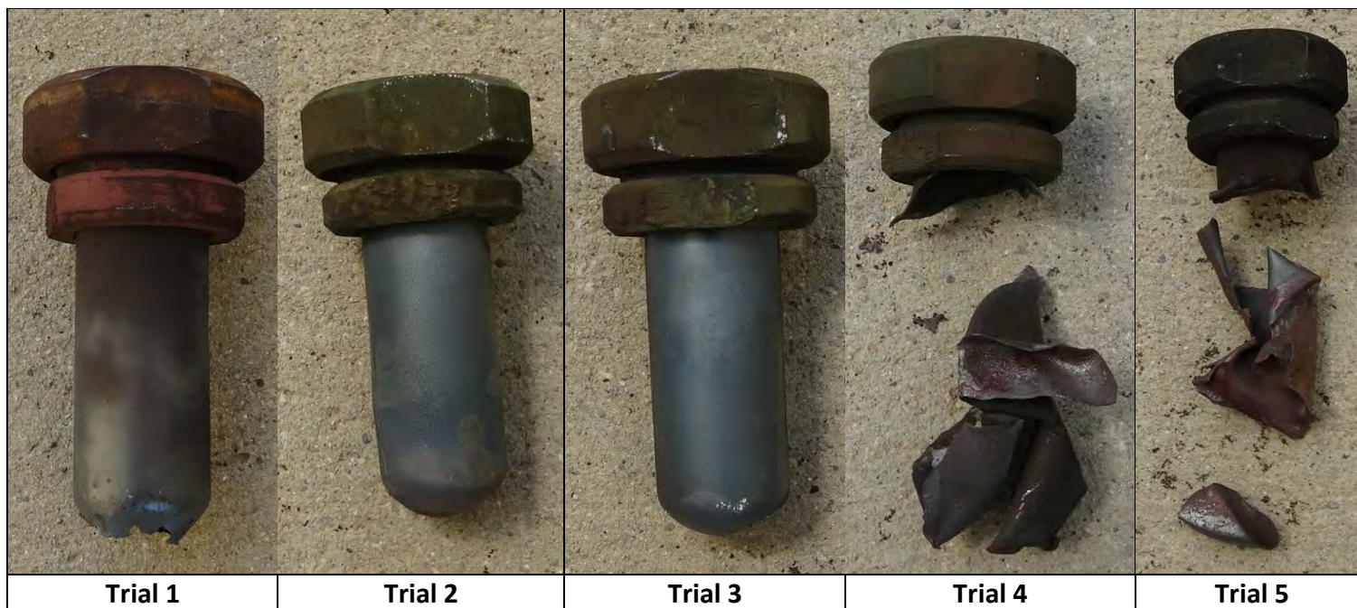
Photo A 6: LS #4-5-D30 Koenen Test Results
