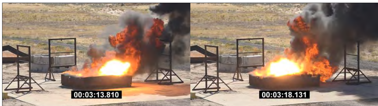
Photo 97: EIS External Fire Test Progression - Visible Reactions of Samples (typical)
