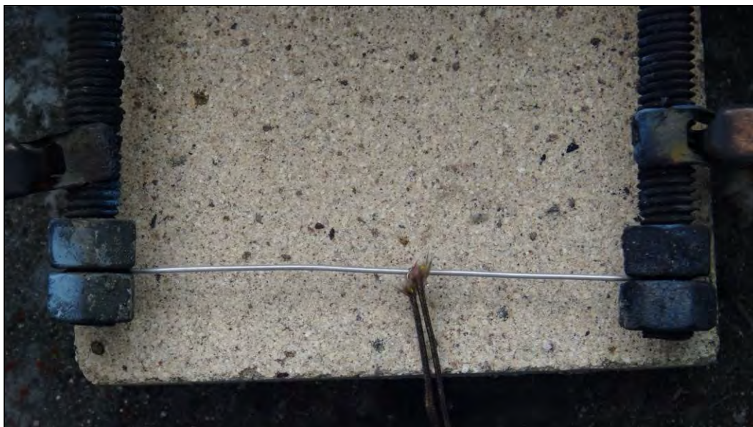
Photo 159: Hotwire Auto-ignition Temperature Apparatus with Dual Thermocouples
