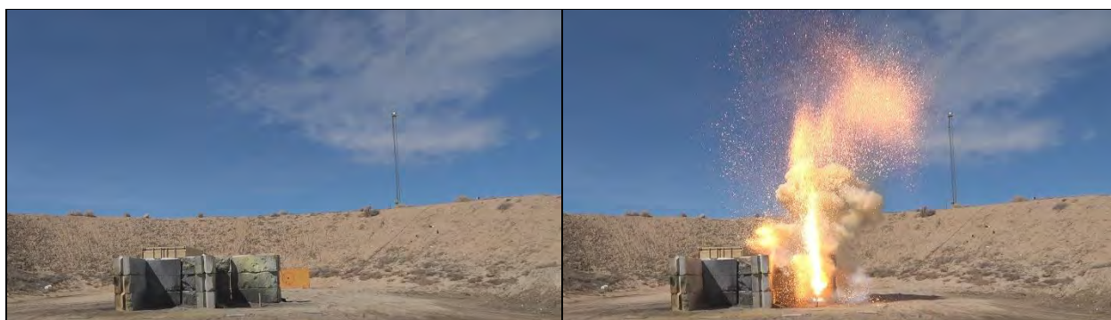
Photo 17: Internal Ignition Test Results (Burning) for SS #30 Al-NiO in the Thin Fiberboard Tube
