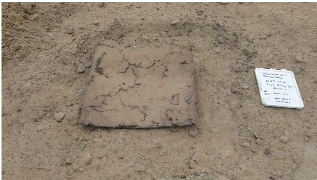
Photo 7: UN Series 6 (a) Single Package Test Results for Fine Al-MnO 2 Thermite – Large-Scale Mix ID #7 (SMS mixed)
