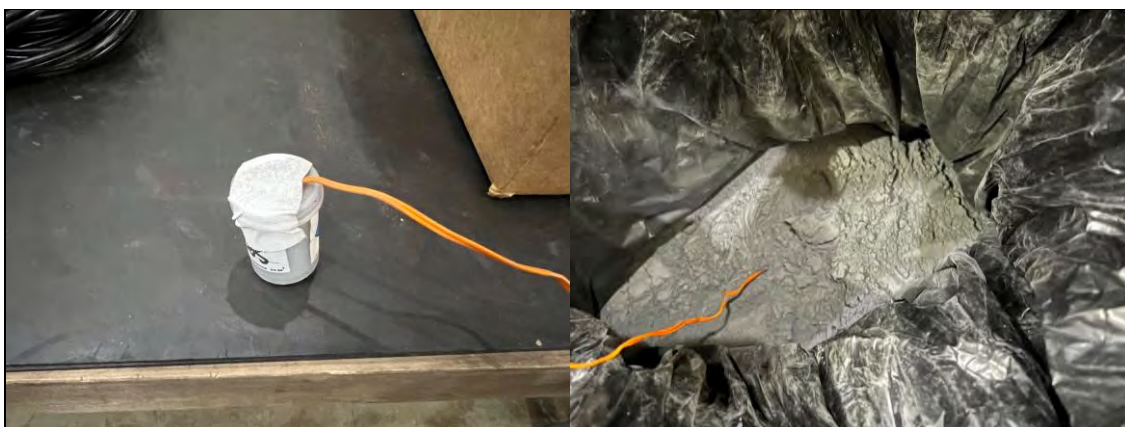
Photo 5: Preparation and Placement of Igniter - typical
