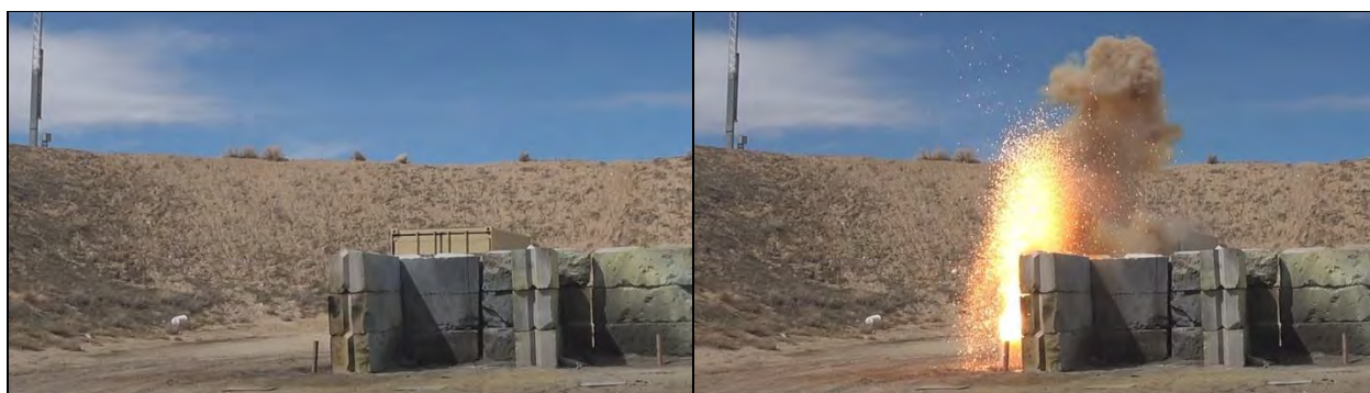
Photo 16: Internal Ignition Test Results (Burning) for SS #27 Al-Fe 3 O 4 in the Thin Fiberboard Tube
