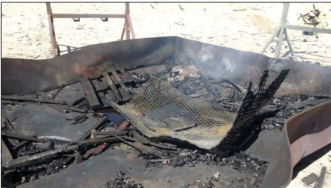
Photo 25: Post-Test Steel Grating in Burn Pan
