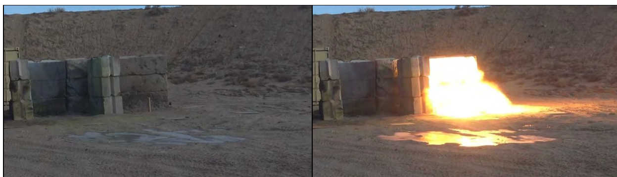
Photo 15: Internal Ignition Test Results (Explosion) for SS #24 Al-Bi 2 O 3 in the Thin Fiberboard Tube
