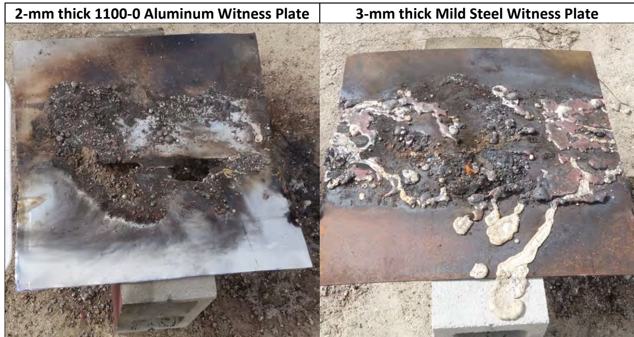
Photo 76: Suspended, Unconfined Package Test Results for Medium Al-CuO Thermite - Mix ID #5 (Commercial)
