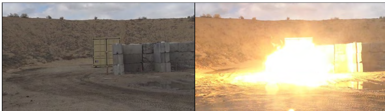
Photo 11: Internal Ignition Test Results (Explosion) for LS #7 Al-MnO 2 in the Thin Fiberboard Tube
