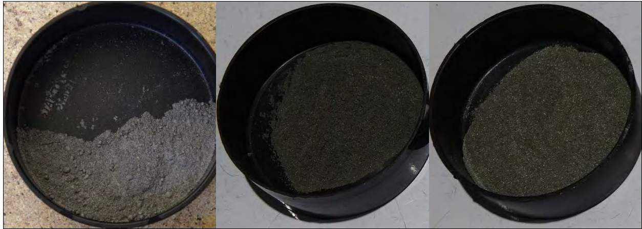
Photo 10: Scale-Scale Mix ID #4 Thermite with Fine Mg and MnO 2 as Fine (left), Medium (center), Coarse (right)
