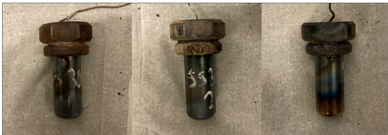
Photo 27: Koenen Test Results for SS #30 Al-NiO, Trials 1 - 3 (left to right)
