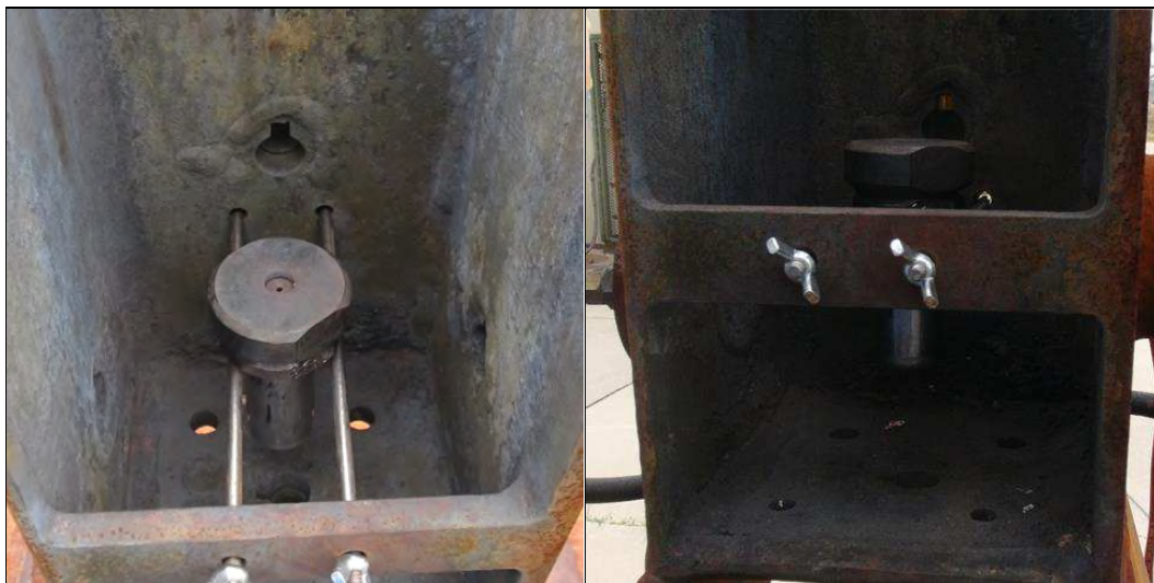
Photo 2: Koenen Tube Suspended in Heating and Protective Device
