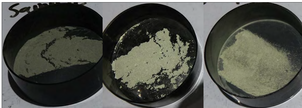
Photo 24: Small-Scale Mix ID #48 Thermite with Coarse Ti and \text{Bi}_2\text{O}_3 as Fine (left), Medium (center), Coarse (right)
