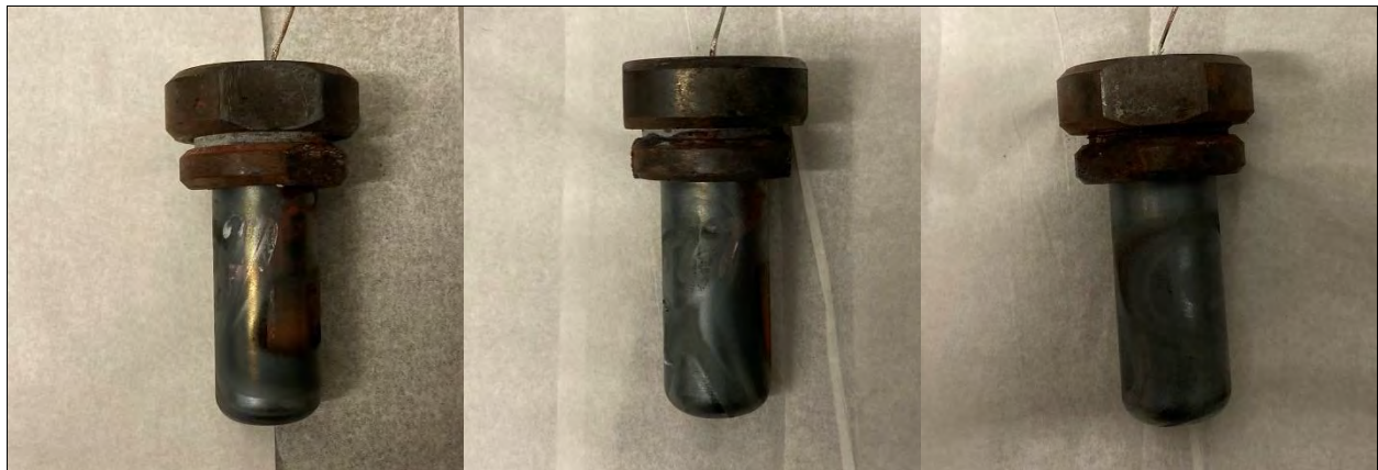
Photo 25: Koenen Test Results for SS #27 Al-Fe 3 O 4 , Trials 1 - 3 (left to right)
