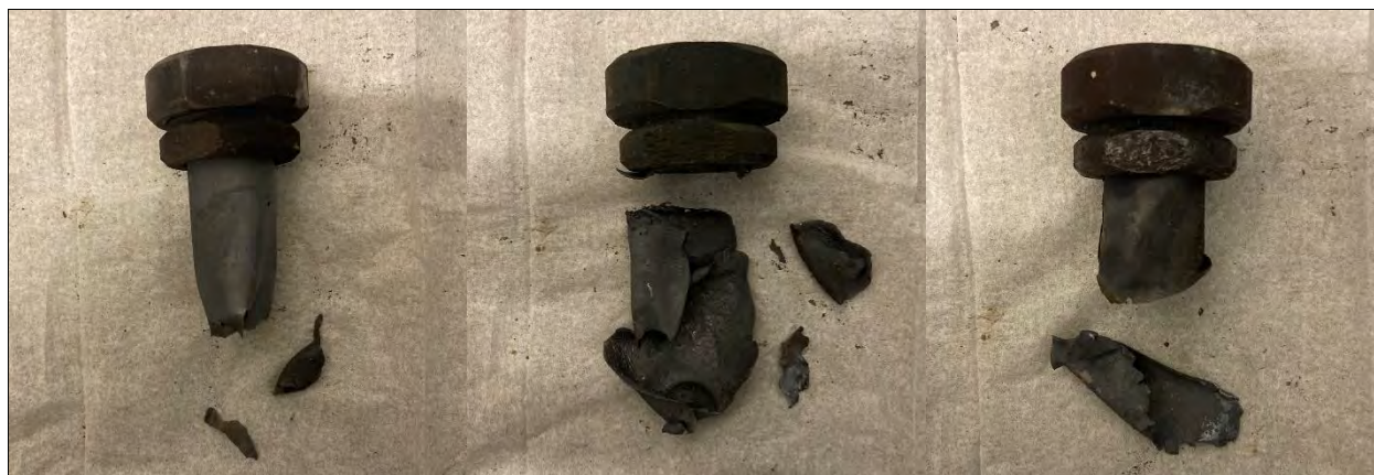
Photo 20: Koenen Test Results for LS #8 Mg&Al-MoO 3 -CuO, Trials 1 - 3 (left to right)
