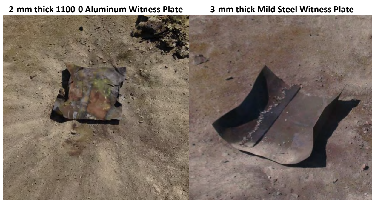
Photo 79: Suspended, Unconfined Package Test Results for Fine Mg&Al-MoO 3 -CuO Thermite - Mix ID #8 (SMS mixed)
