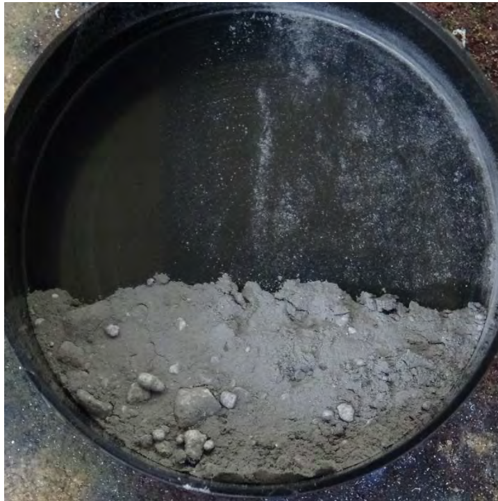
Photo 10: Fine Ti-B 2 O 3 Thermite – Small-Scale Mix ID #2B (SMS mixed)
