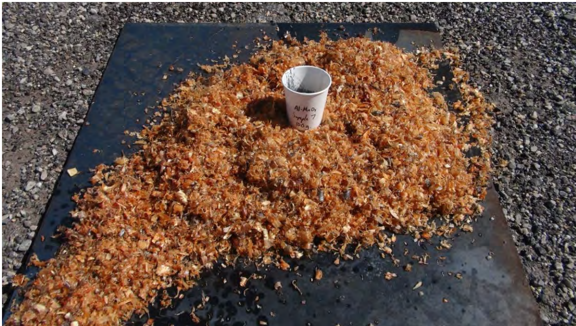
Photo61: Small-scale Burning Test Setup (typical)
