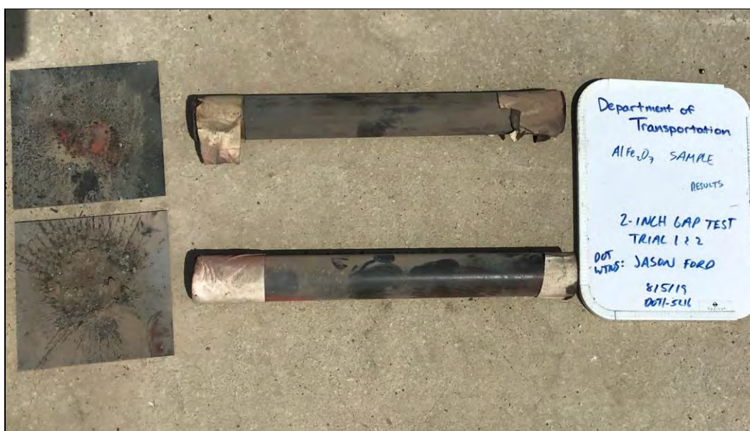
Photo 31: UN 2-in Gap Test Results for Fine Al-Fe 2 O 3 Thermite - Mix ID #1 (SMS mixed)
