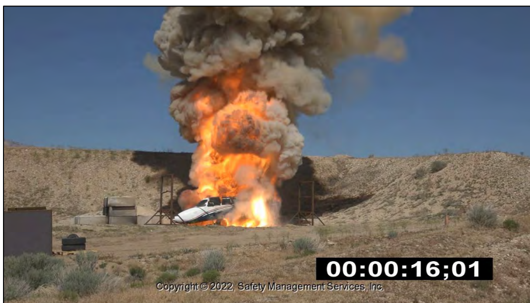
Photo 13: Peak of Reaction During the 1200-pound Stack Test in Airplane Fuselage
