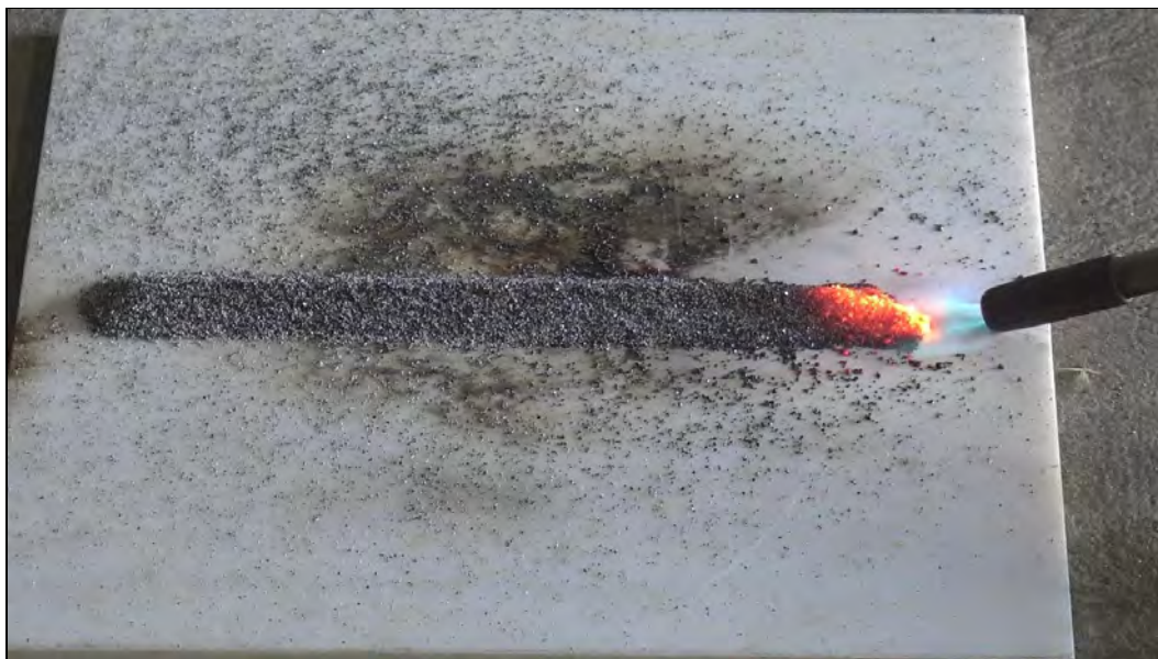
Photo 103: Readily Combustible Test Results - Gas Torch for Coarse \text{Al-Fe}_2\text{O}_3 Thermite A - Mix ID #2 (Commercial) with No Reaction in 5 minutes
