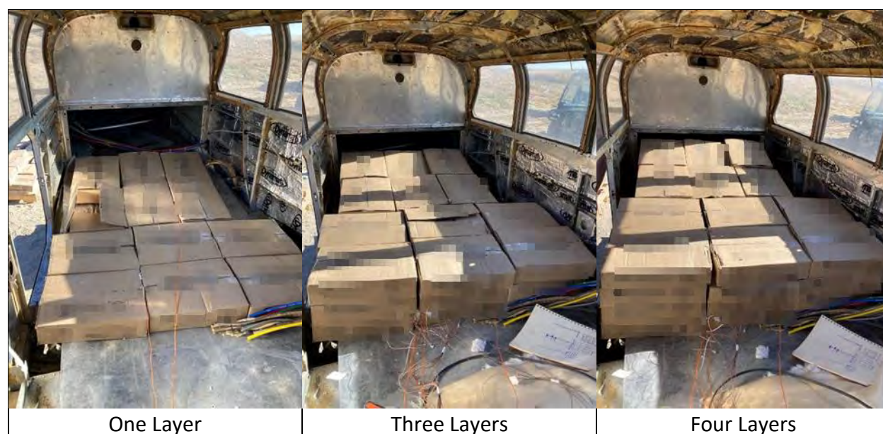
Photo 11: Loading Thermite into the Cargo Area of the Fuselage
