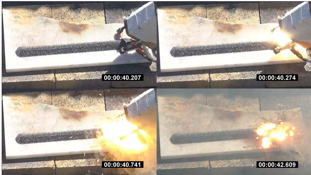
Photo 118: Readily Combustible Test Results - Hot Wire for Medium Al-CuO Thermite - Mix ID #5 (Commercial) with Ignition and Partial Propagation over 2.4 seconds
