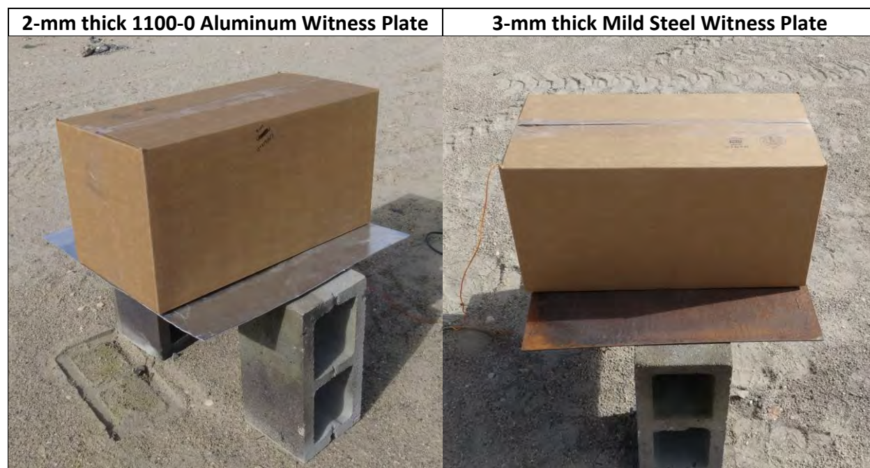
Photo 71: Suspended, Unconfined Single Package Test Setup - typical
