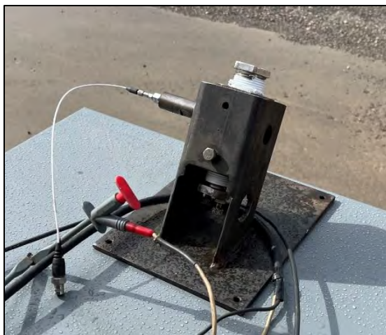
Photo 15: Time/Pressure Ignition Source and Test Setup - typical
