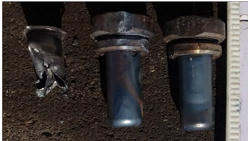
Photo 19: Koenen Test Results for LS #7 Al-MnO 2 , Trials 1 - 3 (left to right)
