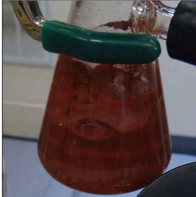
Photo 151: UN Test N.5 Test Results for Fine Al-Fe 2 O 3 Thermite - Mix ID #1 (SMS mixed)
