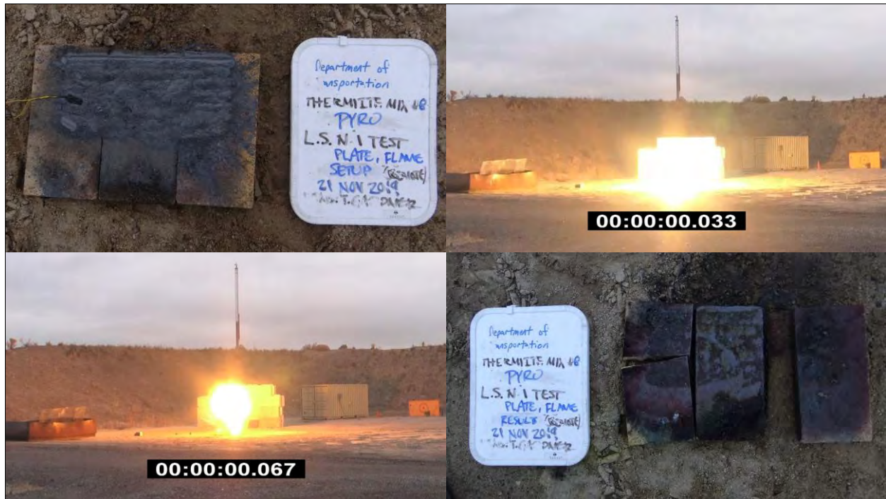
Photo 146: Large-Scale Readily Combustible Test Results - Pyrogen Match on Plate for Fine Mg&Al-MoO 3 -CuO Thermite - Mix ID #8 (SMS mixed) with Explosion
