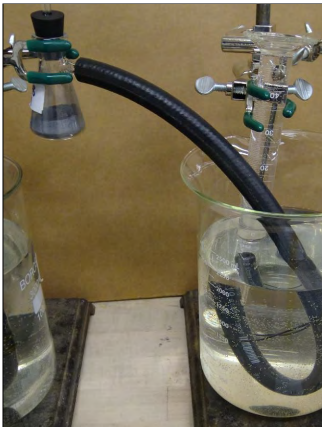
Photo 150: UN Test N.5 Test Setup (typical)
