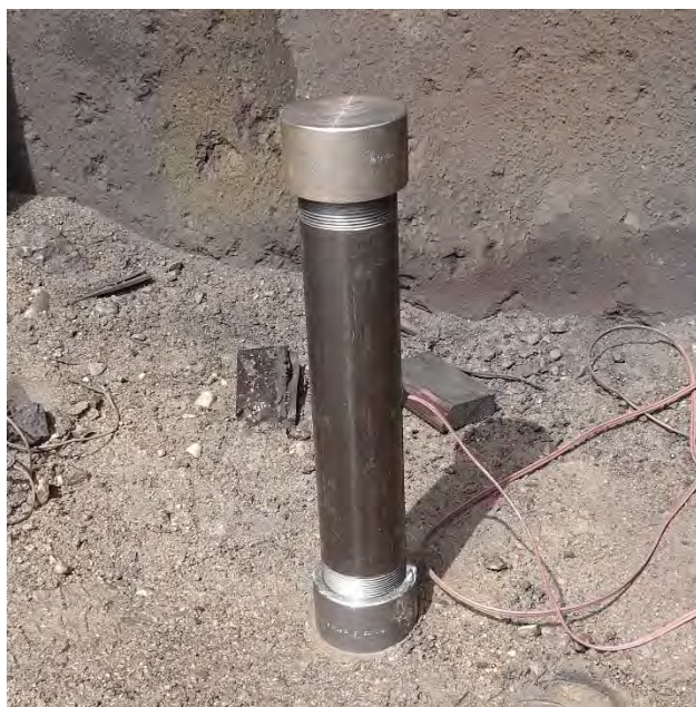
Photo 22: Internal Ignition Test Setup for the Thick-walled Steel Tube – Typical
