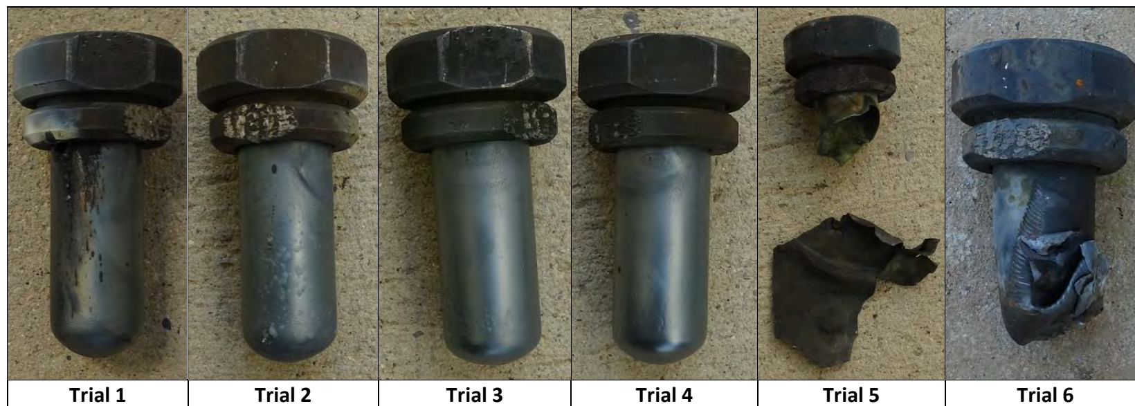
Photo A 2: LS #1-6-C30 Koenen Test Results
