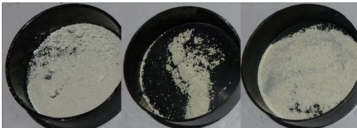
Photo 18: Small-Scale Mix ID #19 Thermite with Coarse Al and \text{SnO}_2 as Fine (left), Medium (center), Coarse (right)
