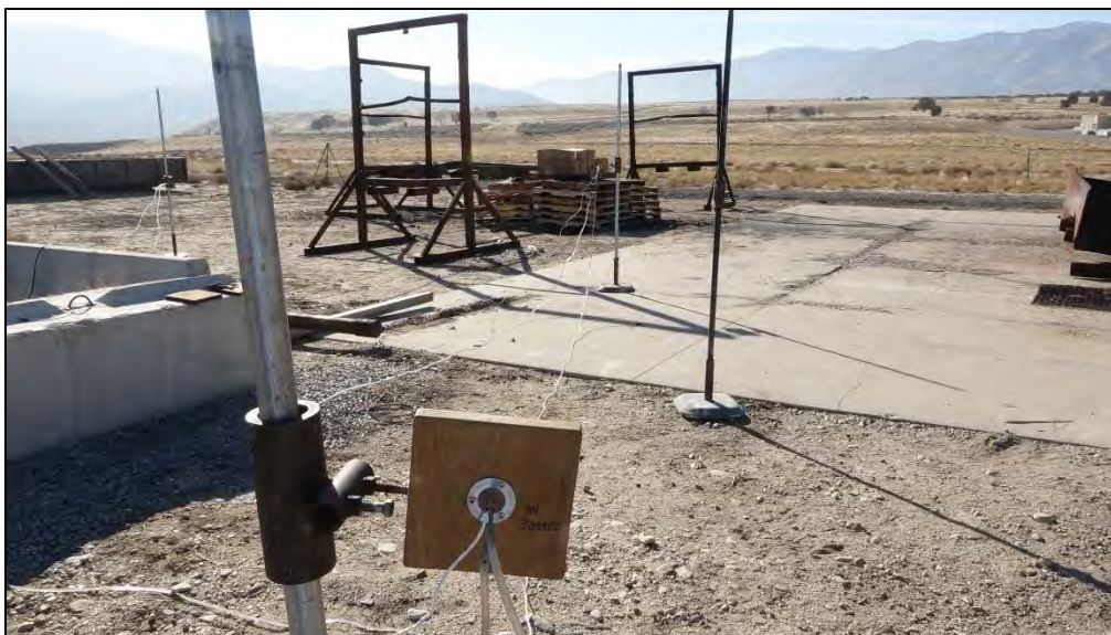
Photo 22: UN Series 6 (c) External Fire – Thermal Flux Instrumentation Setup for Line A - typical
