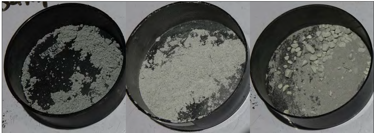
Photo 14: Small-Scale Mix ID #9 Thermite with Medium Al and \text{MoO}_3 as Fine (left), Medium (center), Coarse (right)
