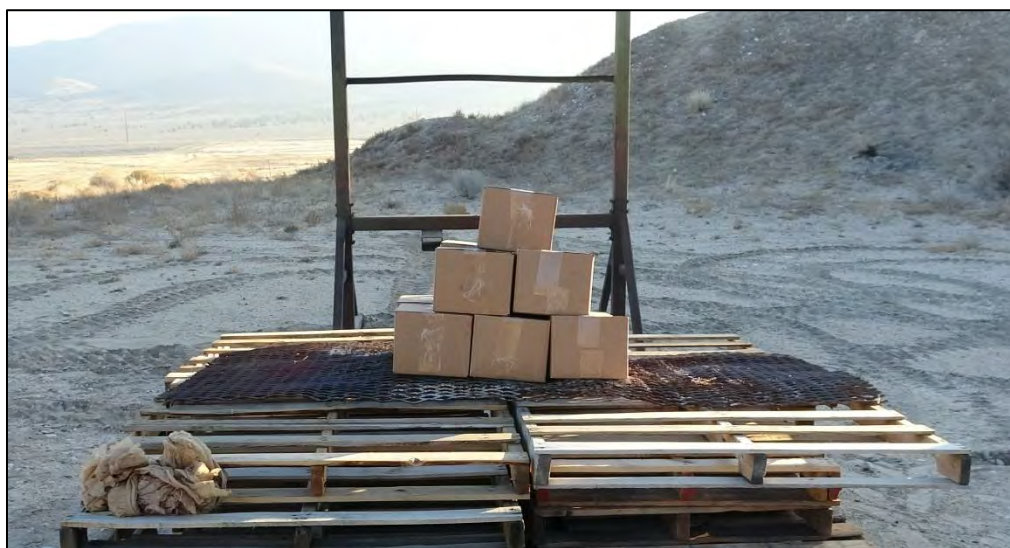
Photo 16: UN Series 6 (c) External Fire Test Setup for Fine \text{Al-Fe}_2\text{O}_3 Thermite – Large-Scale Mix ID #1 (SMS mixed)
