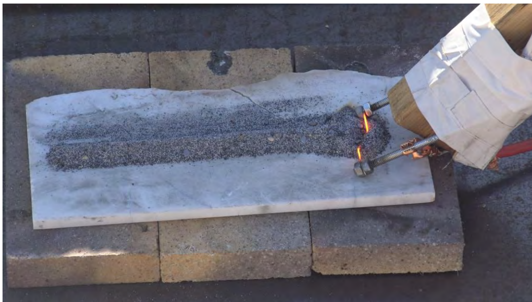
Photo 116: Readily Combustible Test Results - Hot Wire for Coarse Al-Fe 2 O 3 Thermite B - Mix ID #3 (Commercial) with No Reaction in 5 minutes
