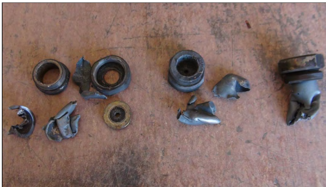
Photo 49: Koenen Test Results for Fine Mg&Al-MoO 3 -CuO Thermite - Mix ID #8 (SMS mixed)
