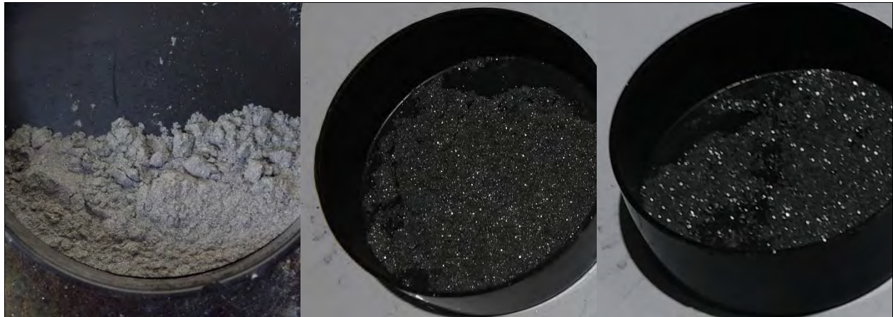
Photo 4: Large-Scale Mix ID #8 Thermite with Fine Mg & Al and \text{MoO}_3 & \text{CuO} as Fine (left), Medium (center), Coarse (right)
