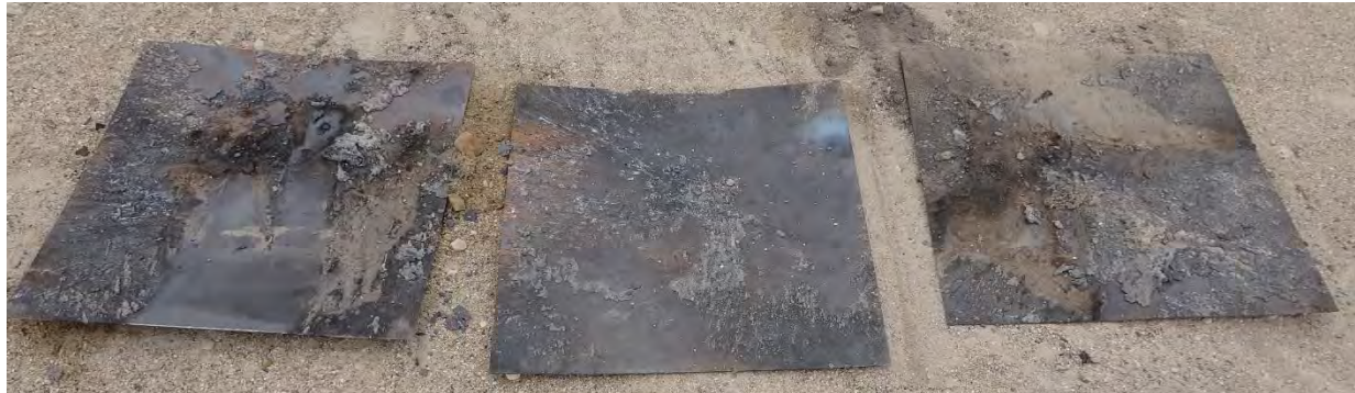
Photo 10: UN Series 6 (a) Single Package Test Results for Fine \text{Al-Fe}_2\text{O}_3 Thermite – Large-Scale Mix ID #1 (SMS mixed)
