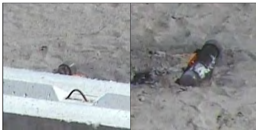
Photo 52: Internal Ignition Test Results for Coarse Al-Fe 2 O 3 Thermite A - Mix ID #2 (Commercial) - typical
