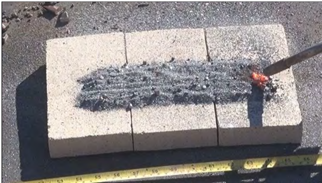
Photo 130: Large-Scale Readily Combustible Test Results - Gas Torch on Plate for Coarse Al-Fe 2 O 3 Thermite B - Mix ID #3 (Commercial) with No Reaction in 5 minutes
