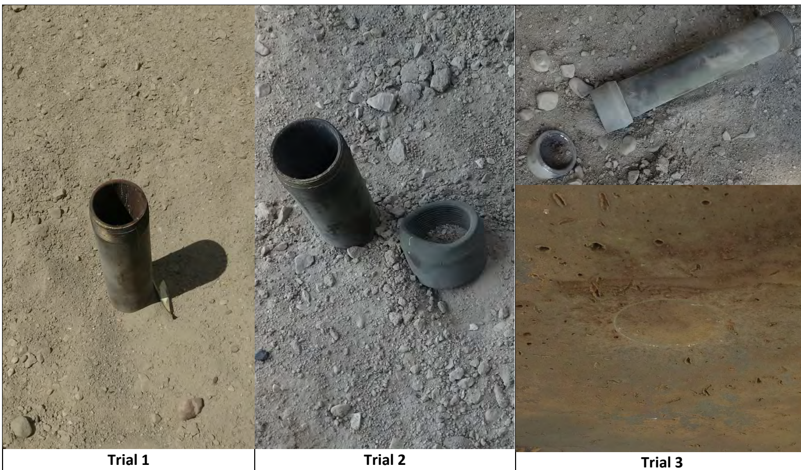
Photo C 3: LS #4-5-A10 Internal 1/2 (c) (ii) Internal Ignition Test Results
