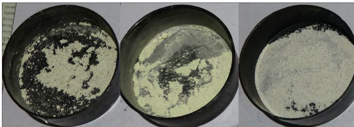
Photo 21: Small-Scale Mix ID #24 Thermite with Coarse Al and \text{Bi}_2\text{O}_3 as Fine (left), Medium (center), Coarse (right)
