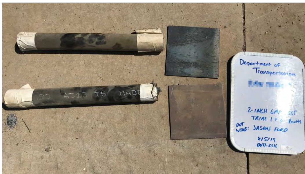
Photo 32: UN 2-in Gap Test Results for Coarse Al-Fe 2 O 3 Thermite A - Mix ID #2 (Commercial)
