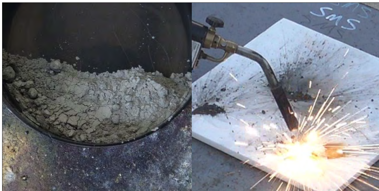
Photo 11: Fine Al-Ni 2 O 3 Thermite - Mix ID #6 (SMS mixed)
