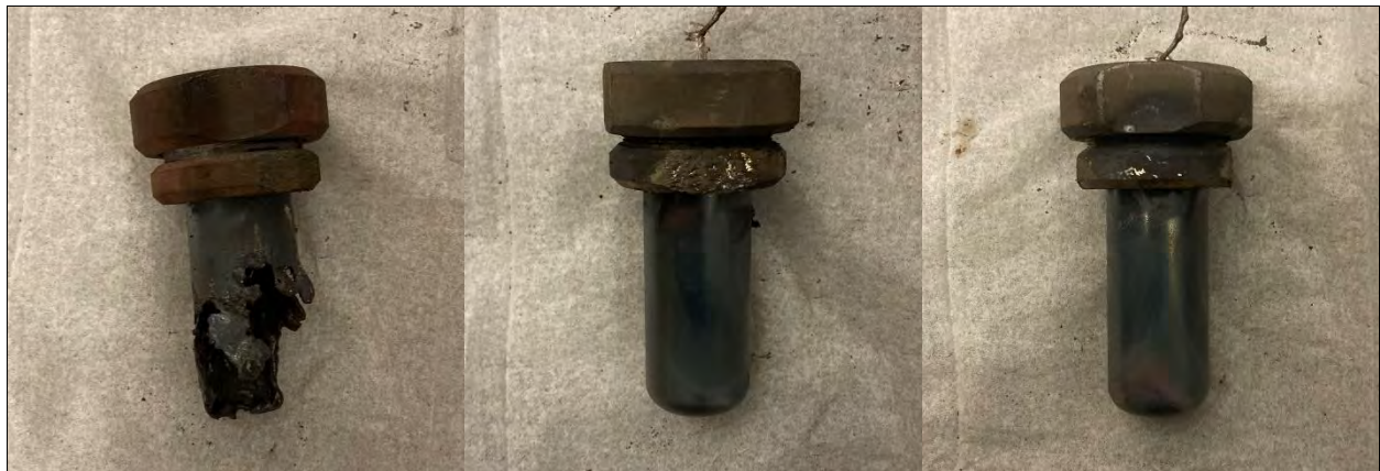
Photo 18: Koenen Test Results for LS #5 Al-CuO, Trials 1 - 3 (left to right)
