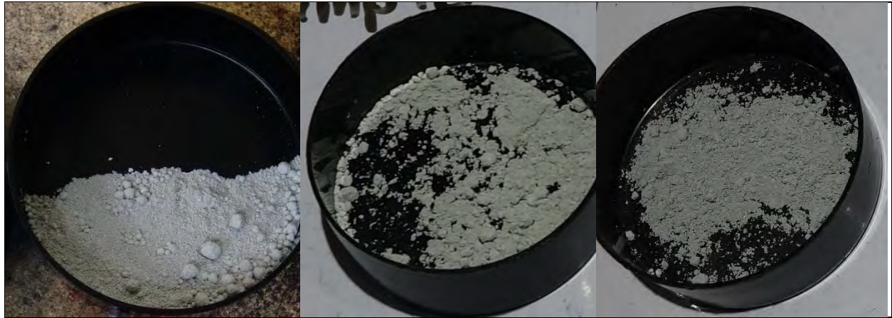
Photo 16: Small-Scale Mix ID #19 Thermite with Fine Al and SnO 2 as Fine (left), Medium (center), Coarse (right)
