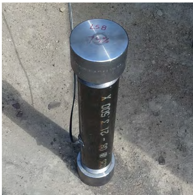
Photo 28: Internal Ignition Test Setup for the Thick-walled Steel Tube at 75% Fill – Typical
