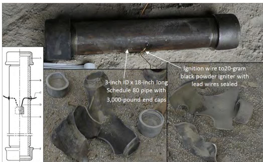
Figure 4: Typical Internal Ignition Test Set-up
