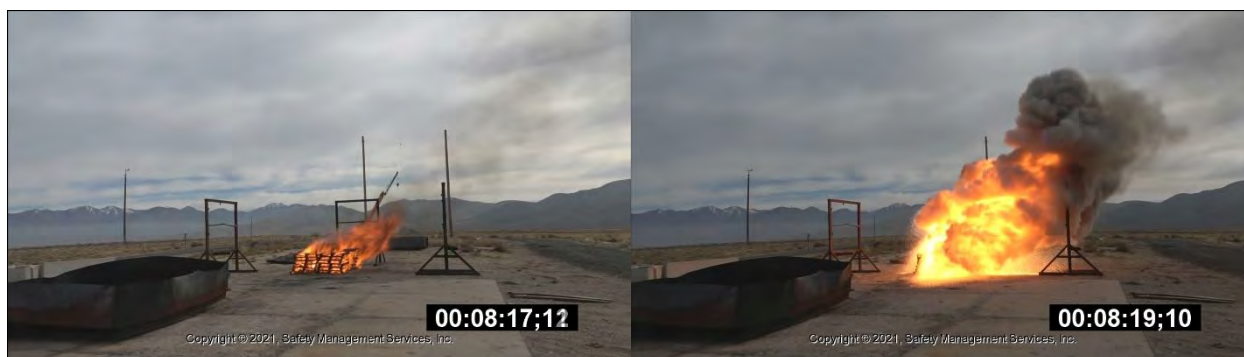
Photo 26: UN Series 6 (c) External Fire – Test Progression for Coarse Al-Fe 2 O 3 Thermite B – Large-Scale Mix ID #3 (Commercial)
