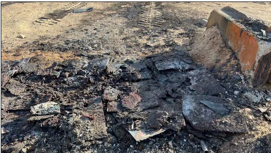
Photo 34: Intermodal Container Test Results - Damage to Witness Plates
