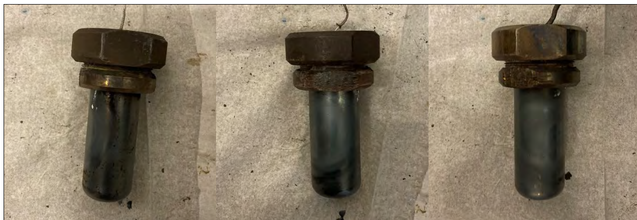
Photo 22: Koenen Test Results for SS #12 Al- \text{Co}_3\text{O}_4 , Trials 1 - 3 (left to right)
