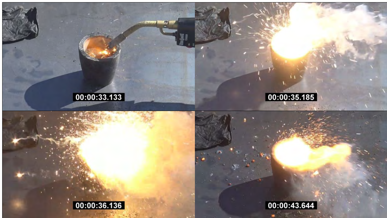
Photo 142: Large-Scale Readily Combustible Test Results - Gas Torch in Crucible for Fine \text{Al-Ni}_2\text{O}_3 Thermite - Mix ID #6 (SMS mixed) with Ignition and Full Consumption over 10.5 seconds
