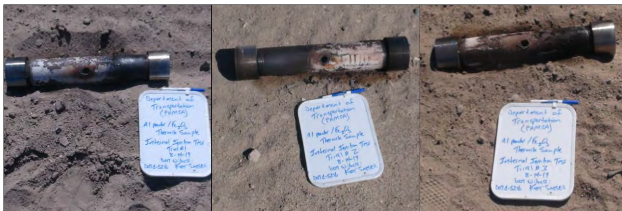
Photo 51: Internal Ignition Test Results for Fine Al-Fe 2 O 3 Thermite - Mix ID #1 (SMS mixed)
