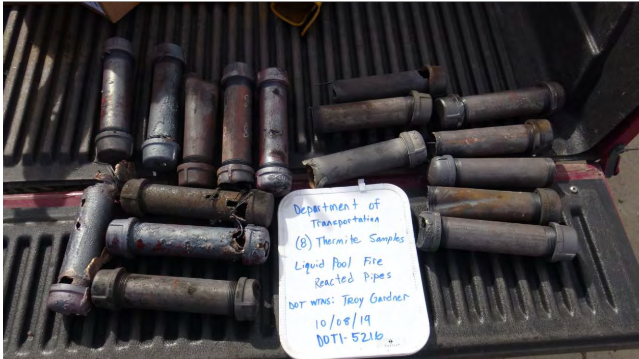
Photo 100: EIS External Fire Test Results - Reacted Pipes
