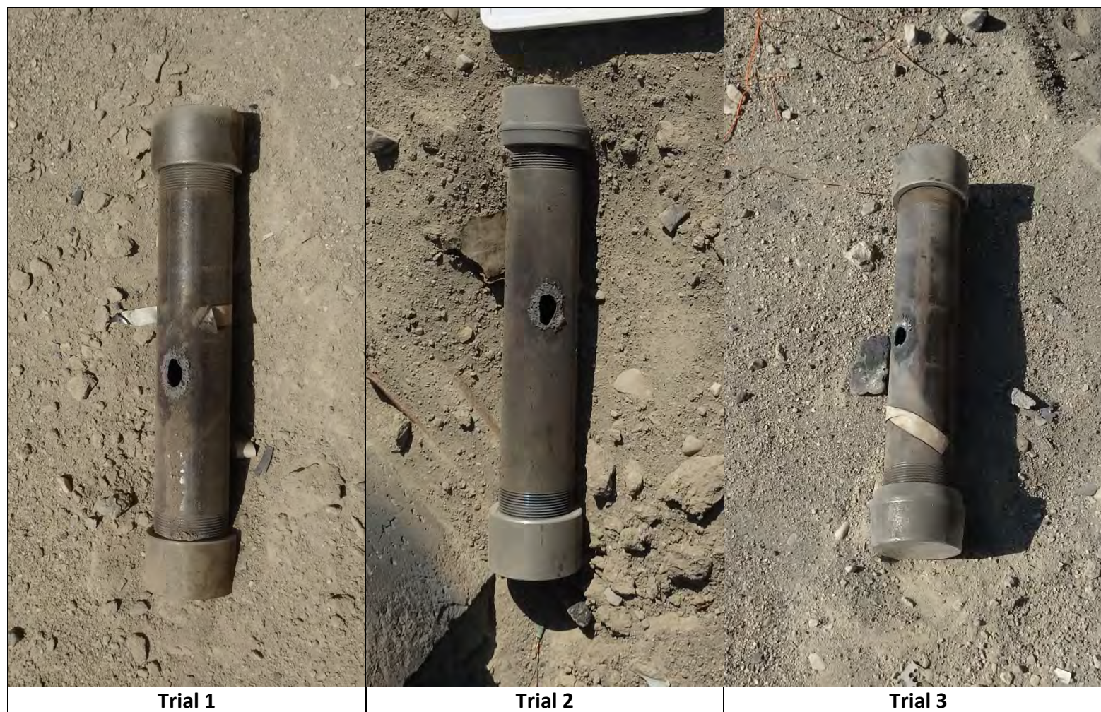
Photo C 1: LS #1-6-A30 Internal 1/2 (c) (ii) Internal Ignition Test Results
