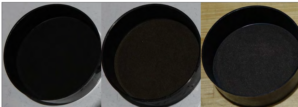
Photo 12: Scale-Scale Mix ID #4 Thermite with Coarse Mg and MnO 2 as Fine (left), Medium (center), Coarse (right)
