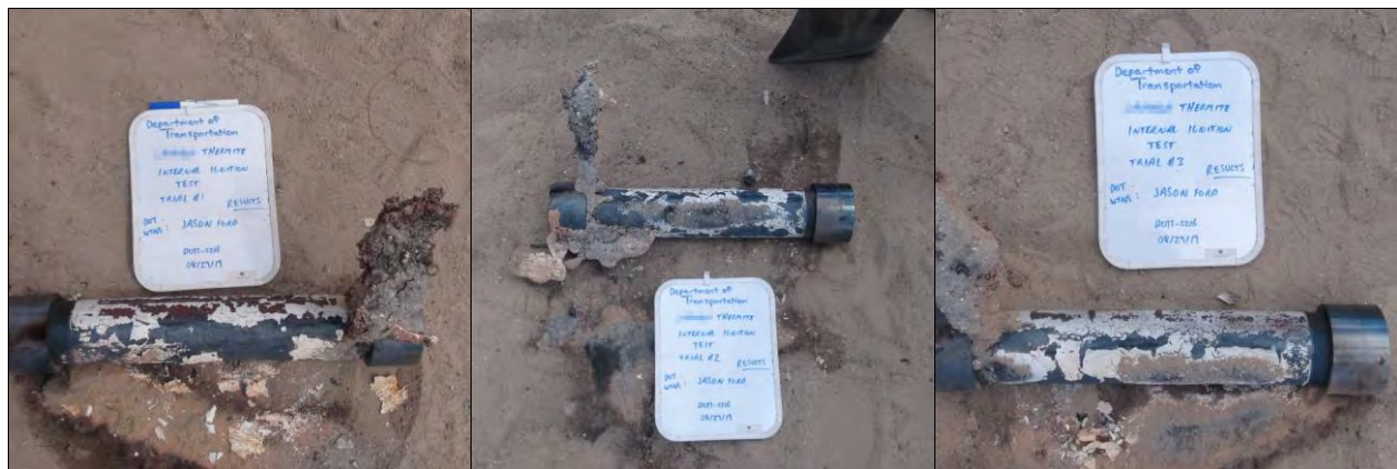
Photo 55: Internal Ignition Test Results for Medium Al-CuO Thermite - Mix ID #5 (Commercial)
