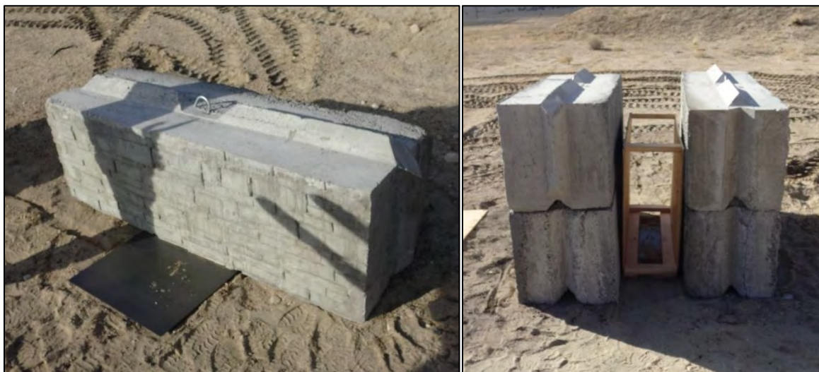
Photo 4: Placement of Witness plate, Concrete Blocks and Simulated Pallet
