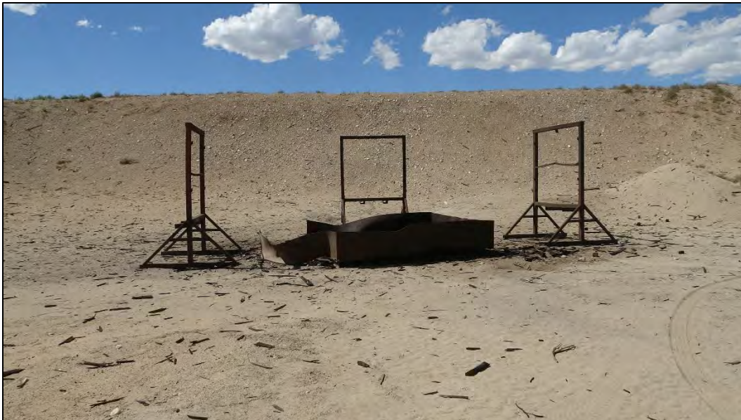
Photo 28: Wood Lattice Scattered by Explosion
