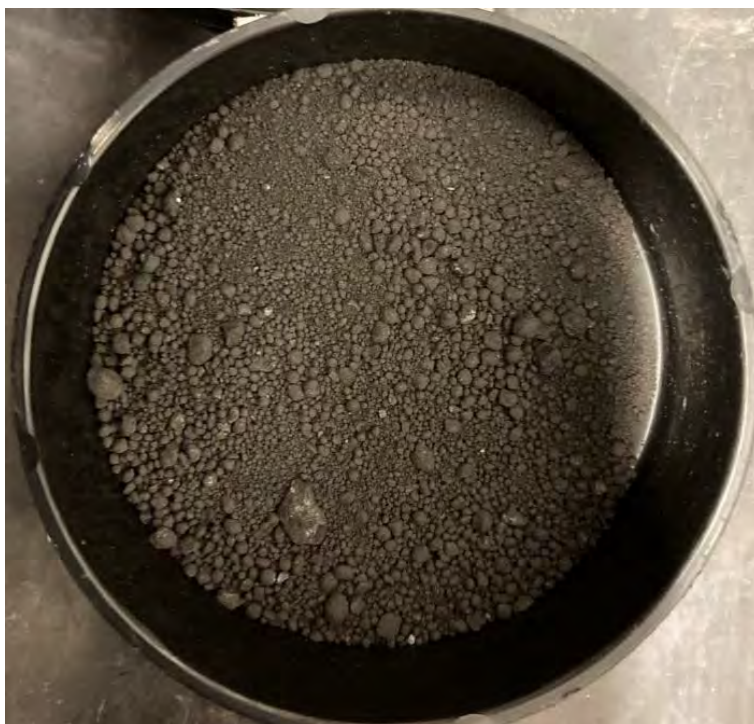
Photo 6: Fine Al-Fe 3 O 4 – Small-Scale Mix ID #27
