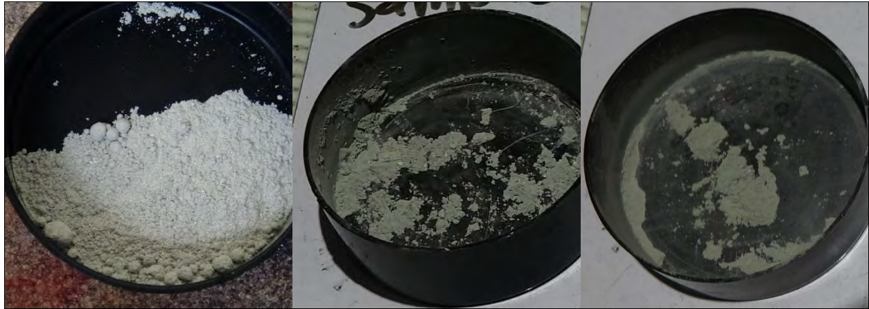
Photo 19: Small-Scale Mix ID #24 Thermite with Fine Al and \text{Bi}_2\text{O}_3 as Fine (left), Medium (center), Coarse (right)
