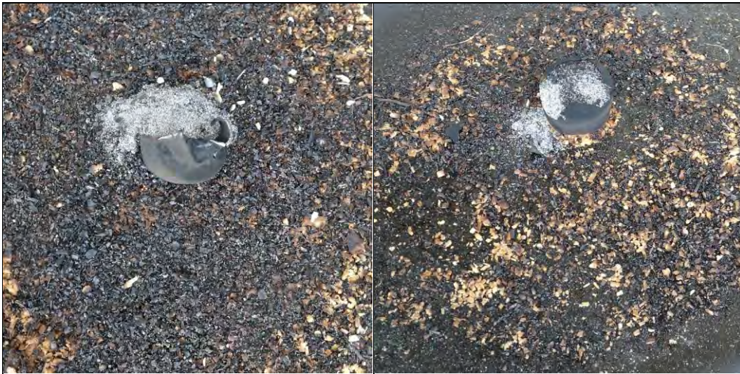
Photo 64: Small-scale Burning Test Results for Coarse Al-Fe 2 O 3 Thermite B - Mix ID #3 (Commercial)
