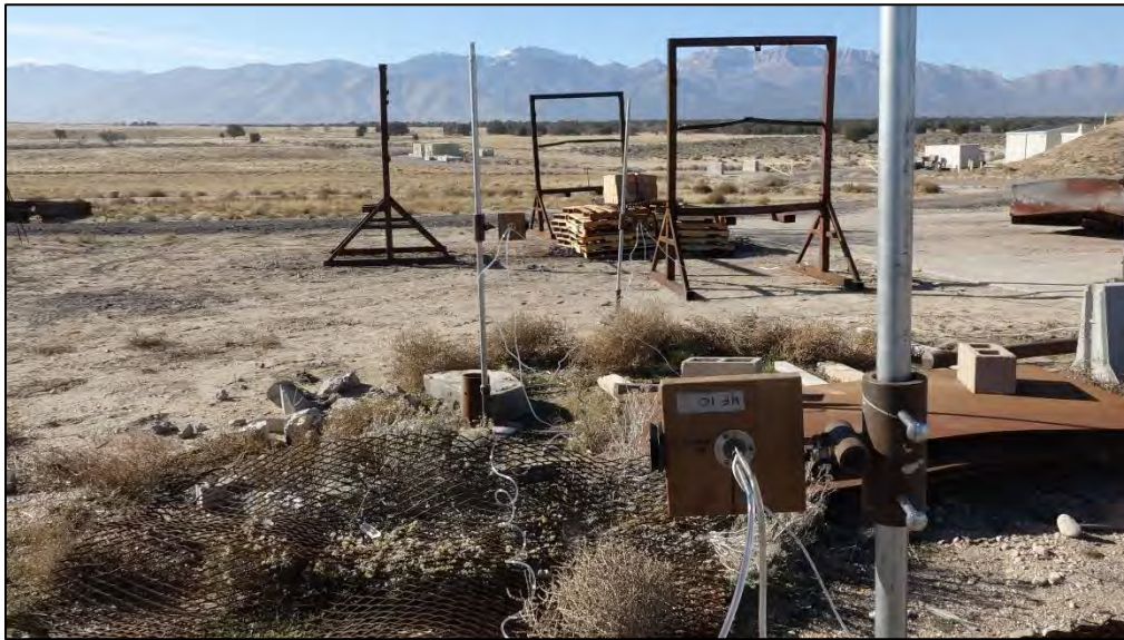
Photo 23: UN Series 6 (c) External Fire – Thermal Flux Instrumentation Setup for Line B - typical
