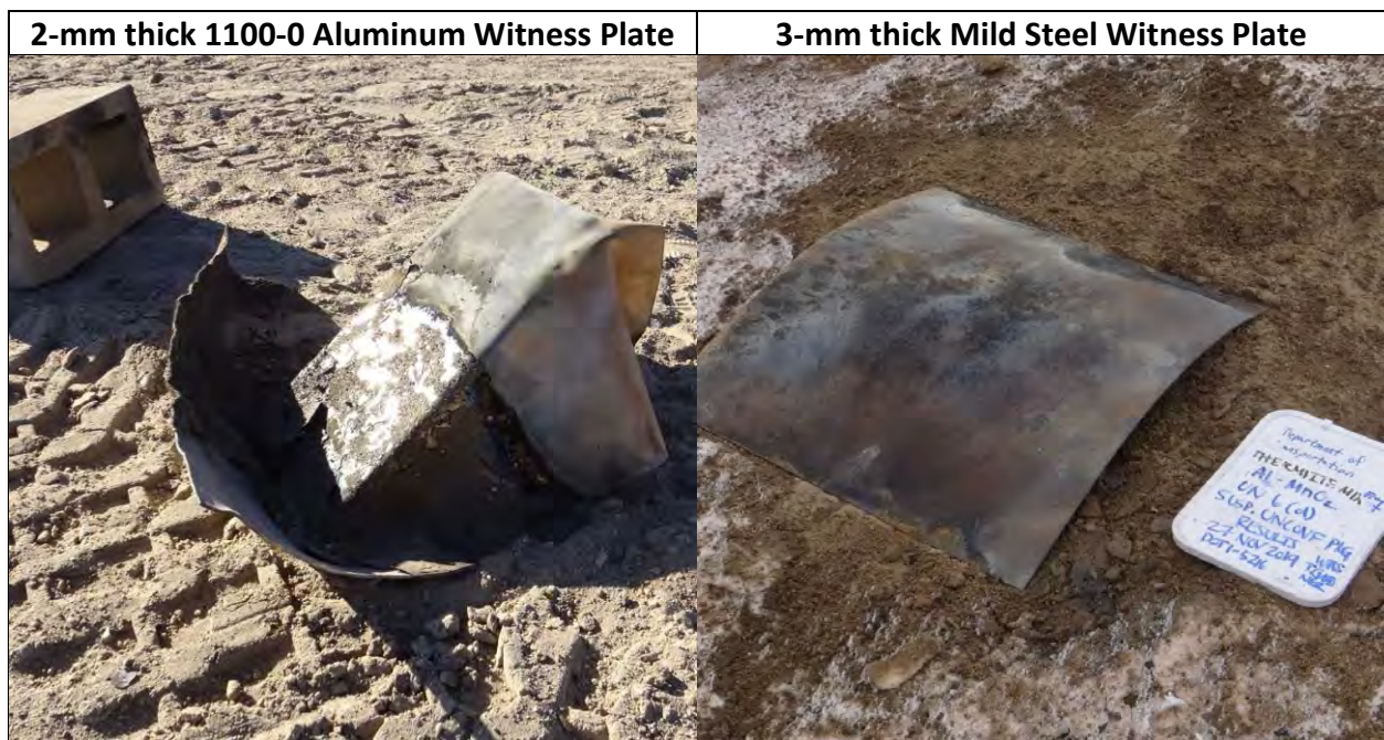
Photo 78: Suspended, Unconfined Package Test Results for Fine \text{Al-MnO}_2 Thermite - Mix ID #7 (SMS mixed)
