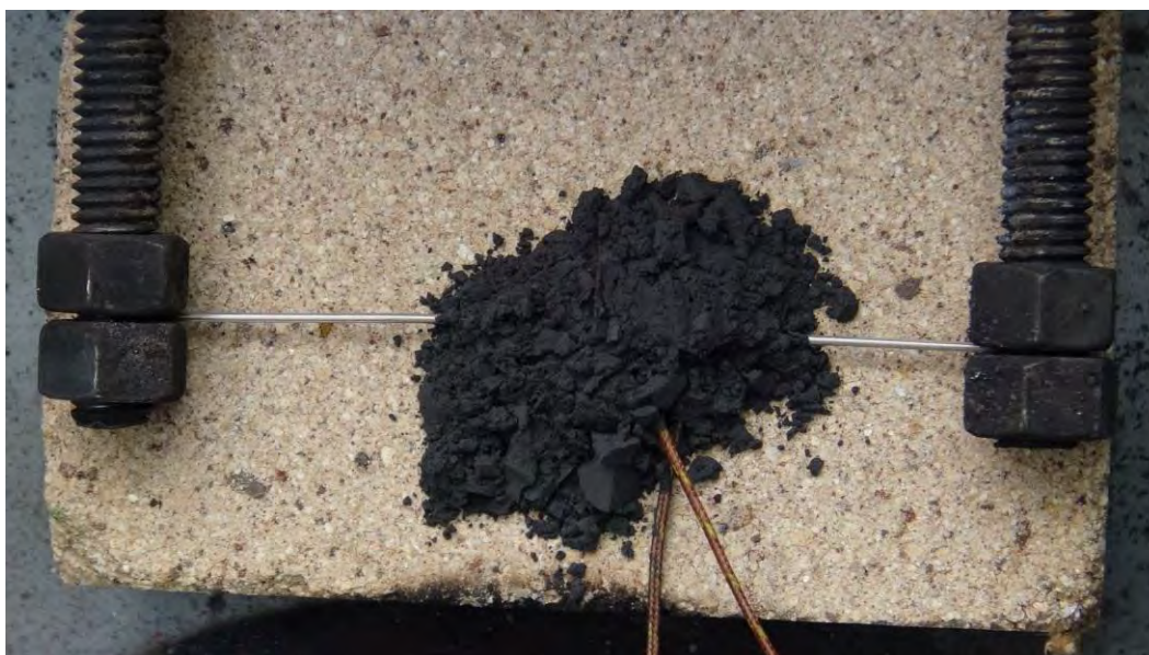
Photo 54: Test Sample Loaded onto Hotwire Auto-ignition Temperature Apparatus
