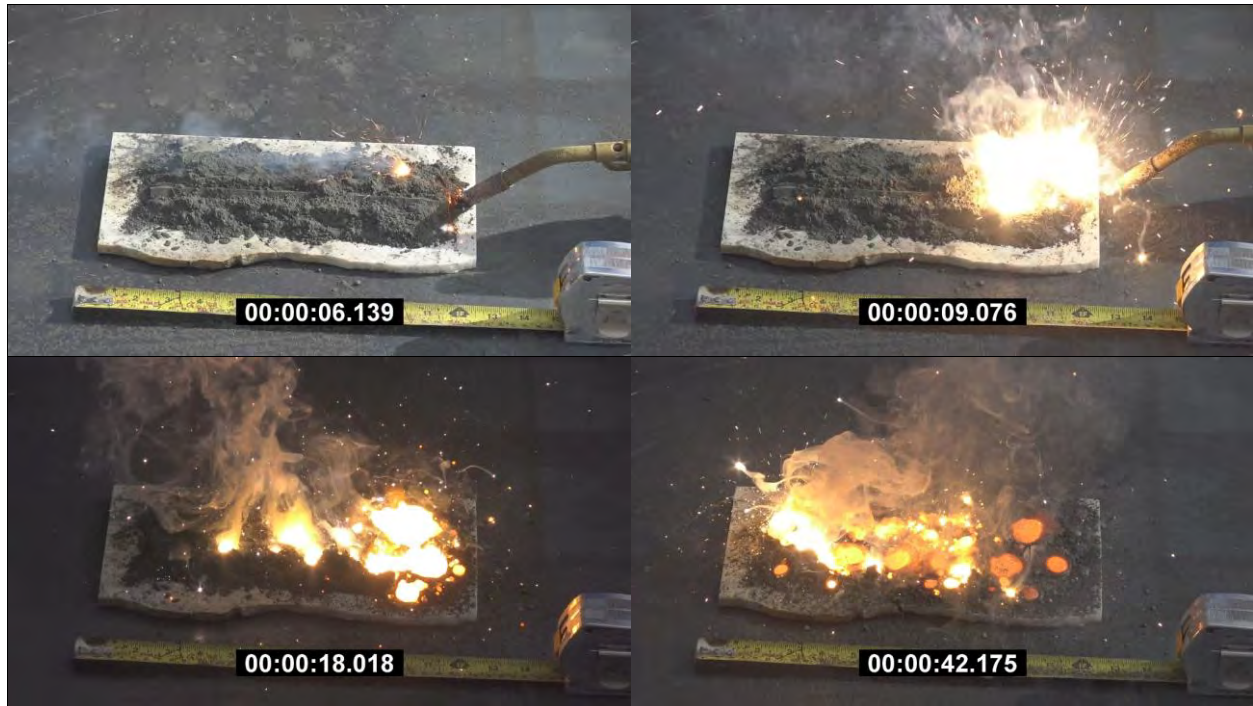
Photo 140: Large-Scale Readily Combustible Test Results - Gas Torch on Plate for Fine Al-Ni 2 O 3 Thermite - Mix ID #6 (SMS mixed) with Ignition and Full Propagation over 36 seconds
