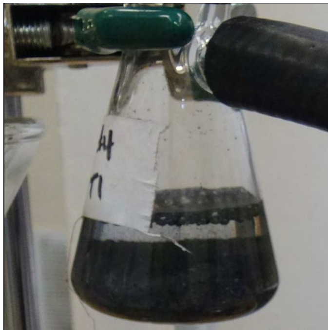
Photo 154: UN Test N.5 Test Results for Fine Al-CuO Thermite - Mix ID #4 (SMS mixed)
