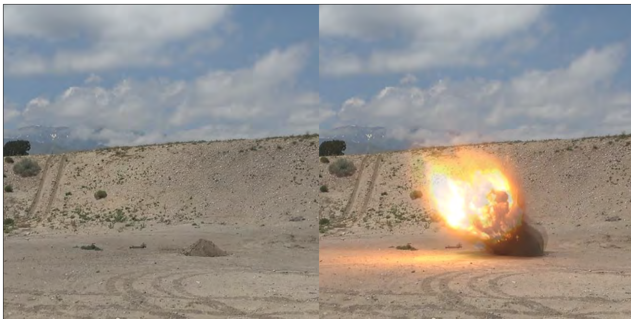
Photo 8: Explosion of Fine Mg&Al-MoO 3 -CuO Thermite – Large-Scale Mix ID #8 (SMS mixed) in the UN Series 6 (a) Single Package Test
