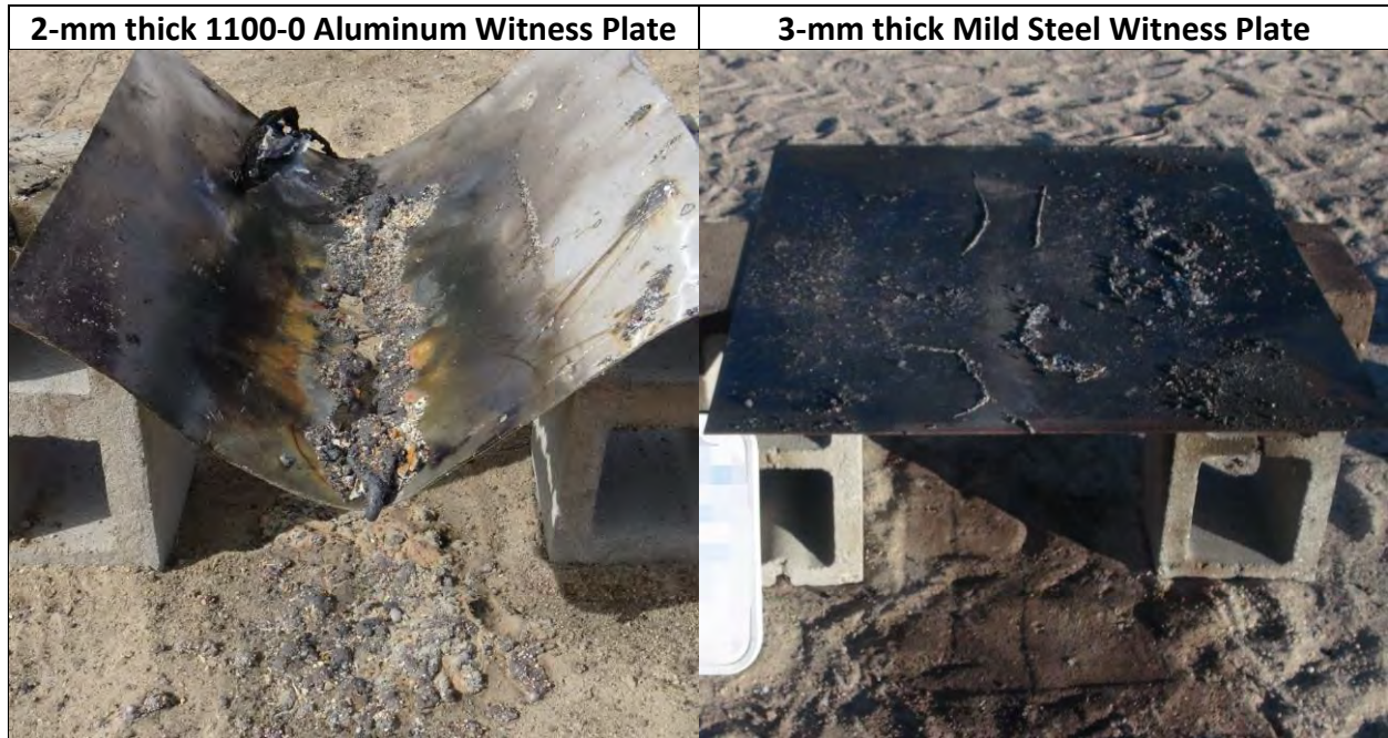
Photo 72: Suspended, Unconfined Package Test Results for Fine Al-Fe 2 O 3 Thermite - Mix ID #1 (SMS mixed)
