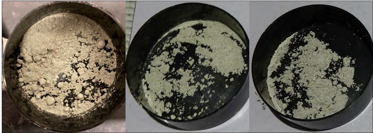
Photo 22: Small-Scale Mix ID #48 Thermite with Fine Ti and \text{Bi}_2\text{O}_3 as Fine (left), Medium (center), Coarse (right)
