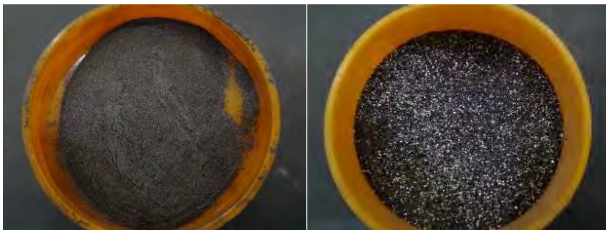
Photo 1: Examples of Thermite Fine Powder (left) and Coarse Powder (right)
