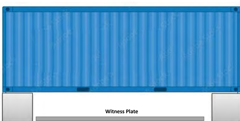
Figure 5: Test Configuration for the Intermodal Container
