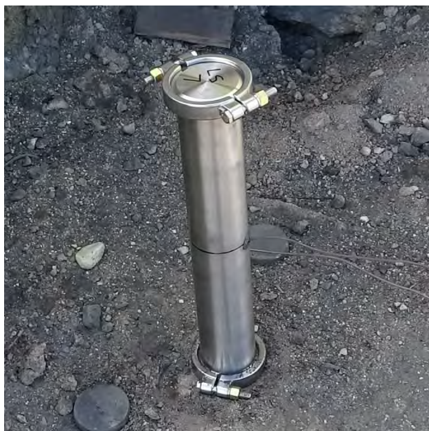
Photo 19: Internal Ignition Test Setup for the Thin-walled Steel Tube – Typical
