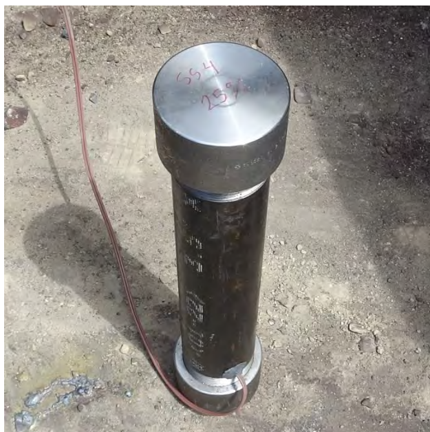
Photo 24: Internal Ignition Test Setup for the Thick-walled Steel Tube at 25% Fill – Typical
