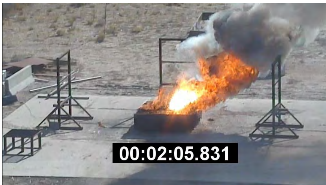
Photo 93: External Bonfire #4 Test Progression - Burning of Fine Al-Ni 2 O 3 Thermite - Mix ID #6 (SMS mixed)
