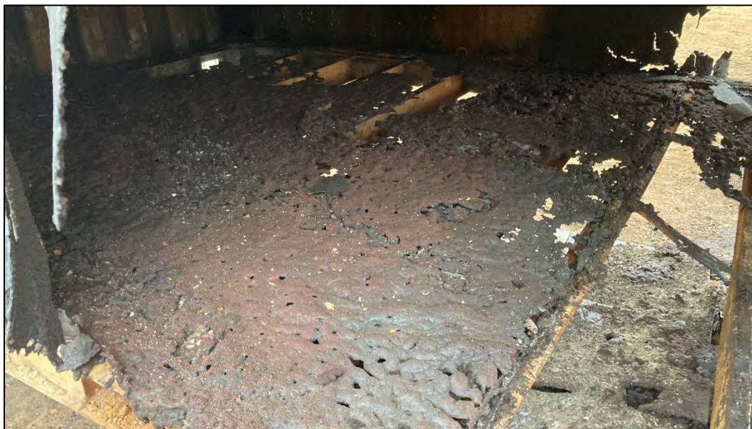
Photo 32: Intermodal Container Test Results - Perforated Container Floor
