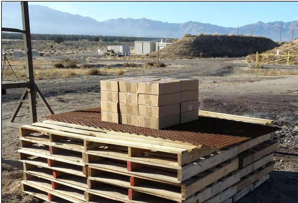
Photo 20: UN Series 6 (c) External Fire Test Setup for Medium Al-CuO Thermite – Large-Scale Mix ID #5 (Commercial)
