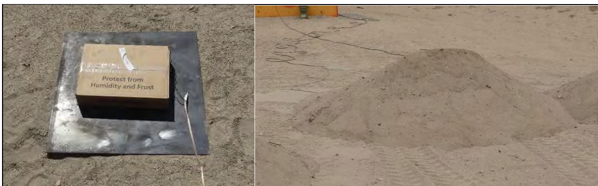
Photo 4: UN Series 6 (a) Single Package Test Setup - typical
