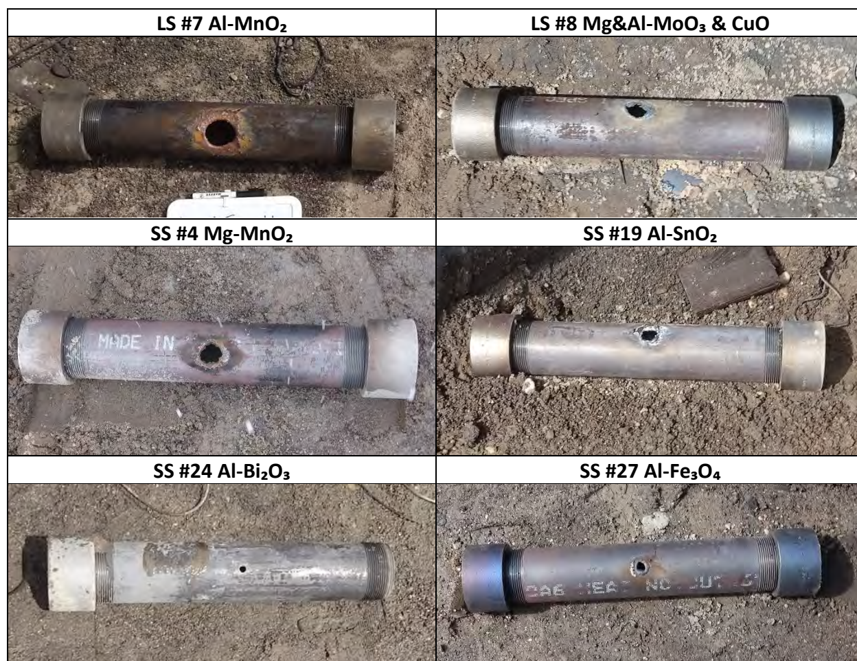
Photo 23: Internal Ignition Test Results for the Thick-walled Steel Tube at 100% Fill
