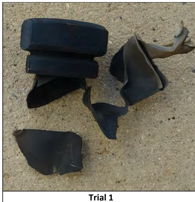
Photo A 1: LS #1-6-A30 Koenen Test Results
