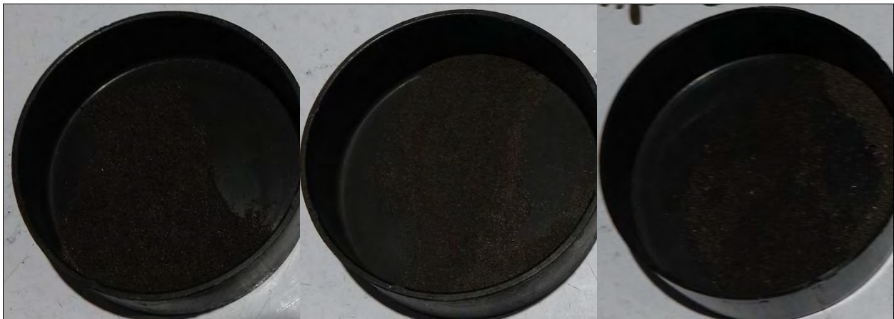
Photo 2: Large-Scale Mix ID #7 Thermite with Medium Al and \text{MnO}_2 as Fine (left), Medium (center), Coarse (right)
