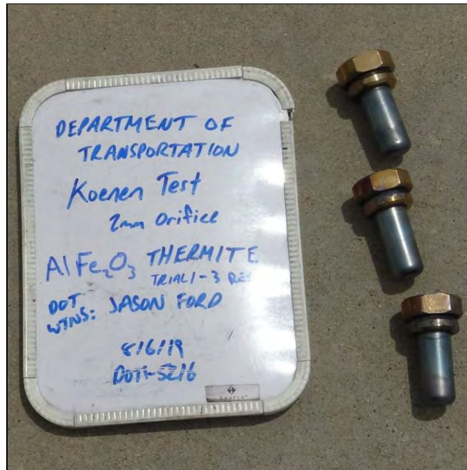
Photo 42: Koenen Test Results for Fine \text{Al-Fe}_2\text{O}_3 Thermite - Mix ID #1 (SMS mixed)
