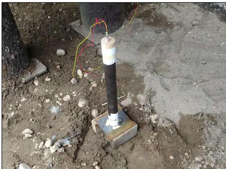
Photo 7: UN Series (a) Zero Gap Test Setup – typical
