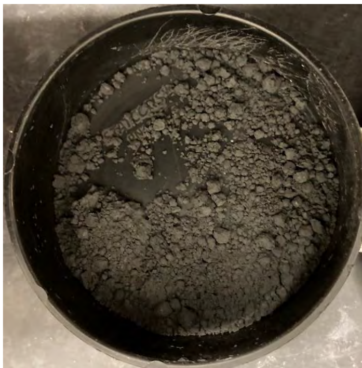
Photo 26: Fine Al-Mn 2 O 3 – Small-Scale Mix ID #28
