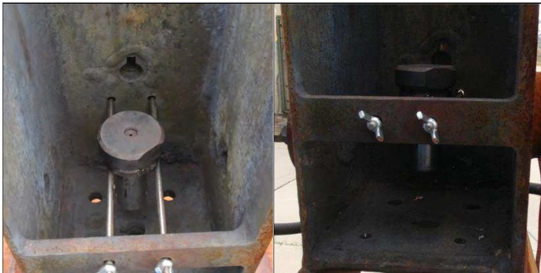
Photo 14: Koenen Tube Suspended in Heating and Protective Device
