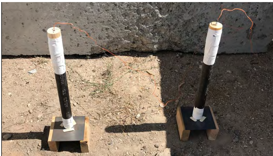
Photo 30: UN 2-inch Gap Setup (typical)
