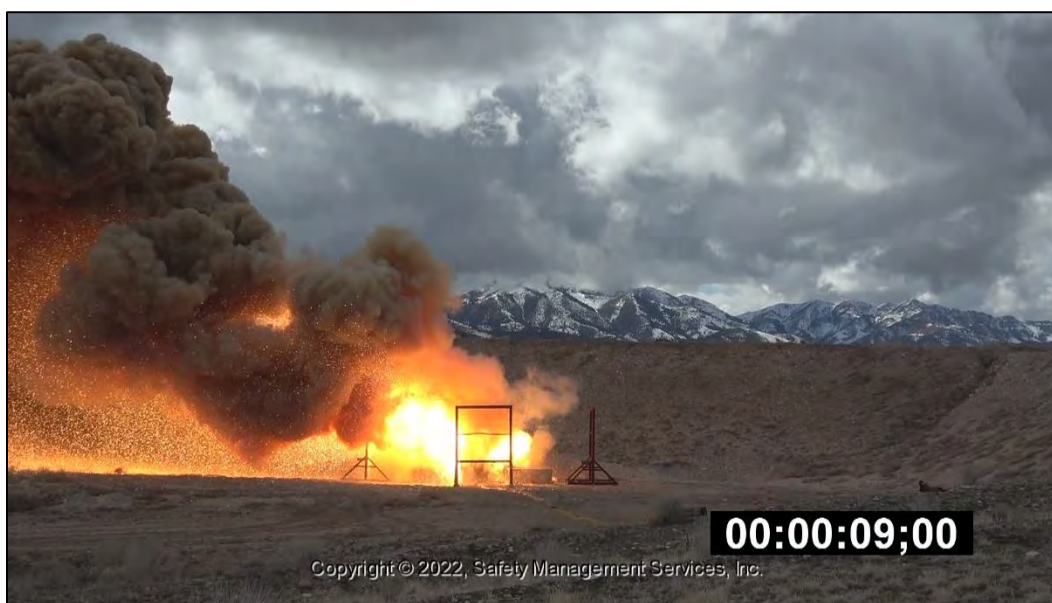
Photo 8: Peak of Reaction for the Modified 800-pound Stack Test
