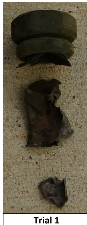
Photo A 5: LS #4-5-C30 Koenen Test Results
