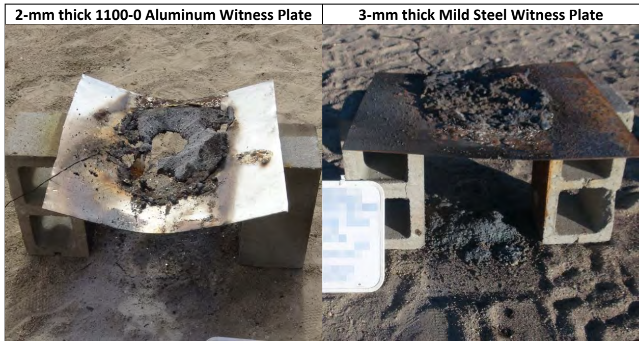
Photo 74: Suspended, Unconfined Package Test Results for Coarse Al-Fe 2 O 3 Thermite B - Mix ID #3 (Commercial)
