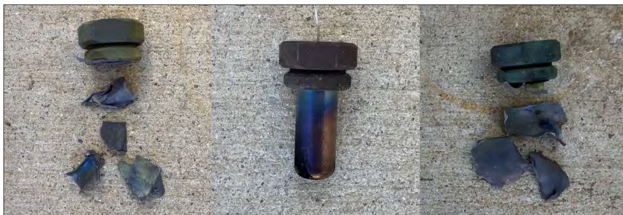
Photo 28: Koenen Test Results for SS #48 Ti-Bi 2 O 3 , Trials 1 - 3 (left to right)
