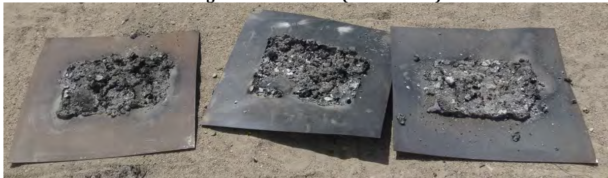
Photo 12: UN Series 6 (a) Single Package Test Results for Coarse \text{Al-Fe}_2\text{O}_3 Thermite B – Large-Scale Mix ID #3 (Commercial)
