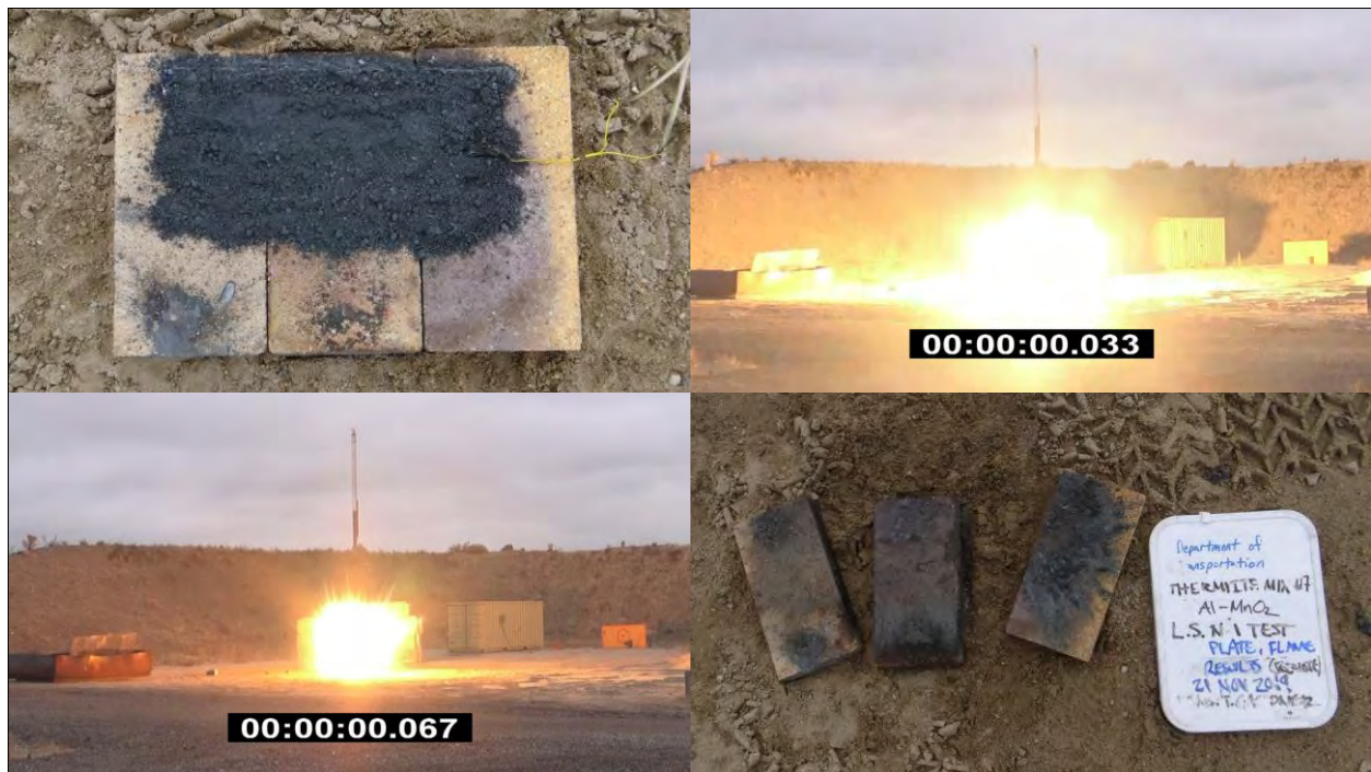
Photo 143: Large-Scale Readily Combustible Test Results - Pyrogen Match on Plate for Fine \text{Al-MnO}_2 Thermite - Mix ID #7 (SMS mixed) with Explosion
