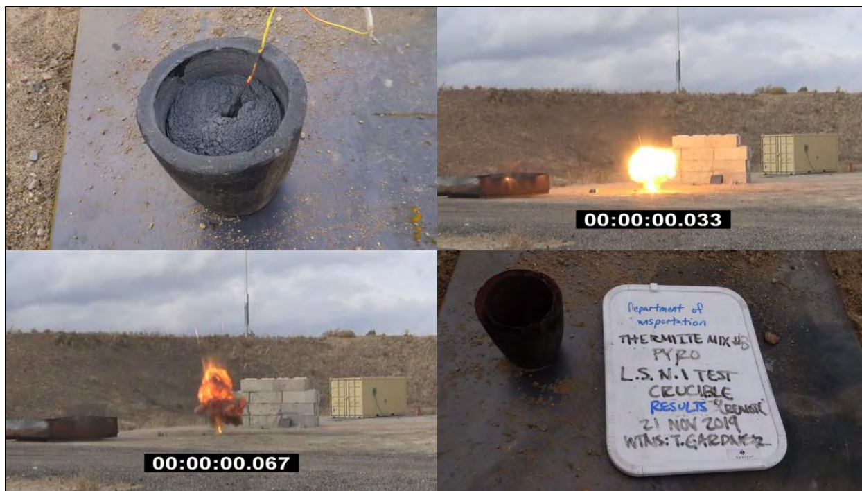
Photo 148: Large-Scale Readily Combustible Test Results - Pyrogen Match in Top of Crucible for Fine Mg&Al-MoO 3 -CuO Thermite - Mix ID #8 (SMS mixed) with Explosion
