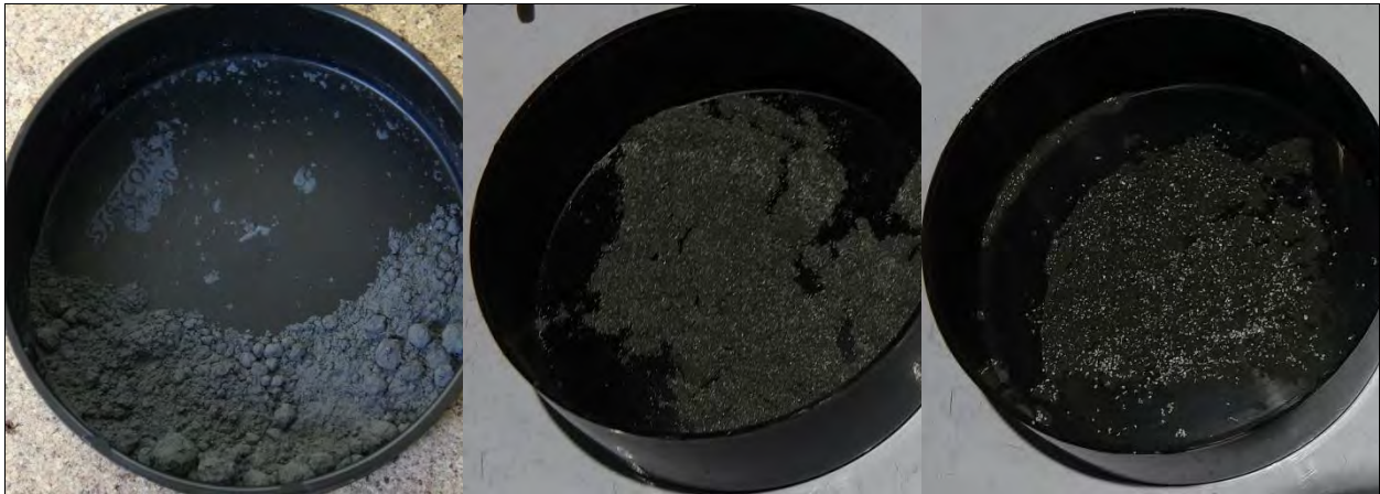
Photo 1: Large-Scale Mix ID #7 Thermite with Fine Al and \text{MnO}_2 as Fine (left), Medium (center), Coarse (right)
