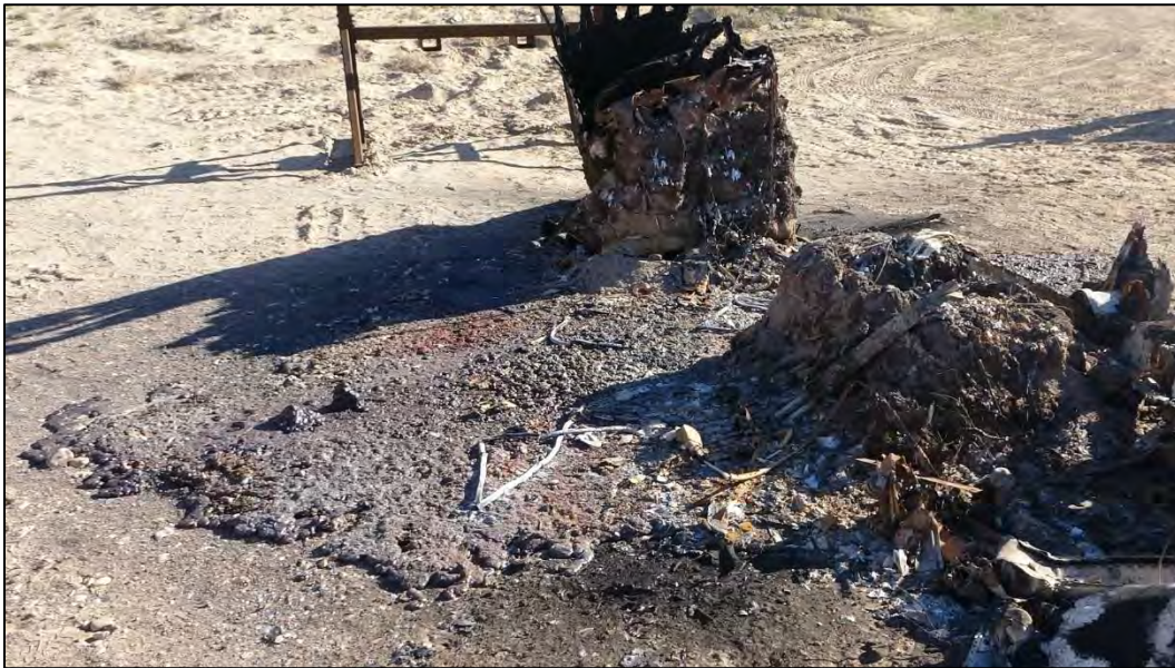
Photo 16: Solidified Pool of Thermite Slag (Fe and \text{Al}_2\text{O}_3 ) from the 1200-lb Stack Test
