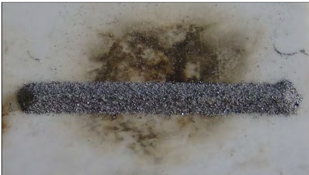
Photo 101: Readily Combustible Solids Test Setup (typical)
