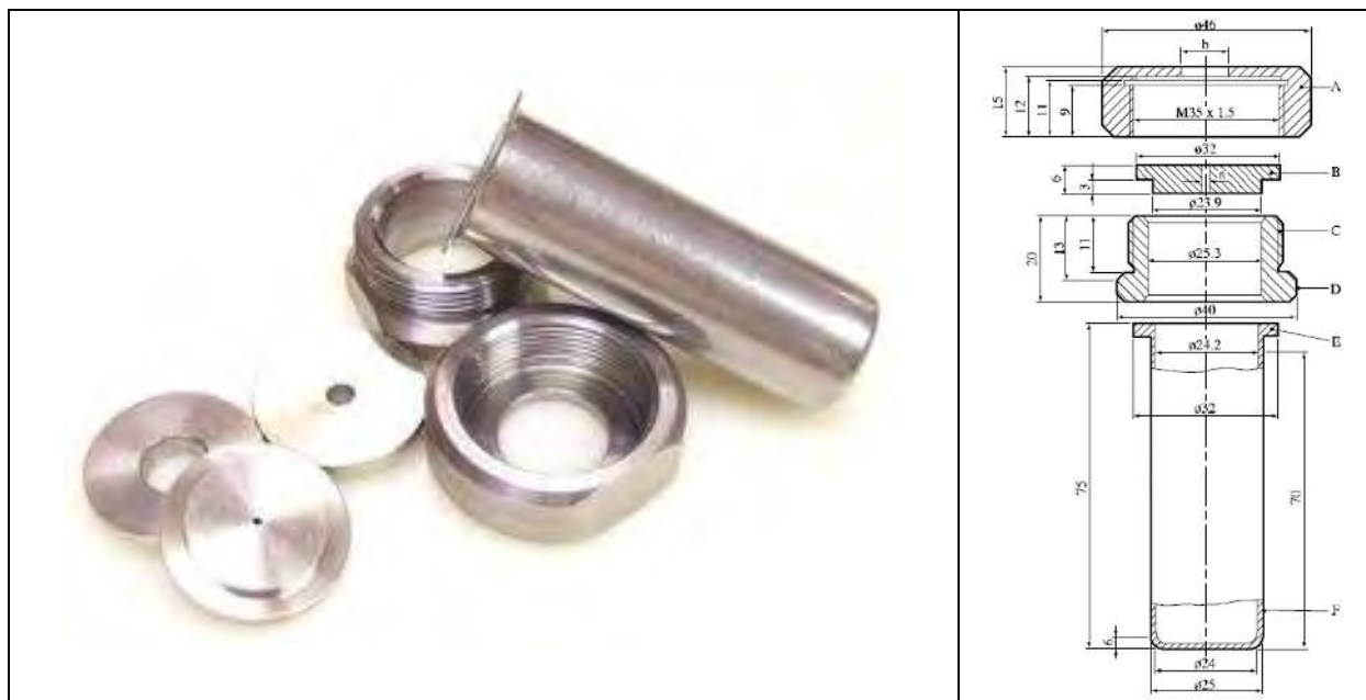
Photo 1: Koenen Tube, Orifice Plates, and Reusable Closing Device
