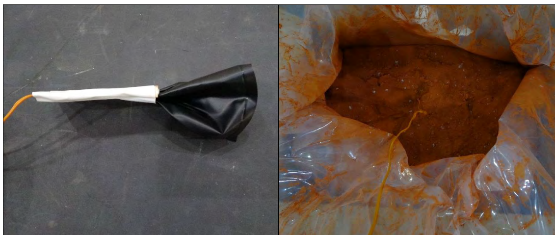
Photo 19: Placement of Thermite Starter Mix Bag Igniter - typical
