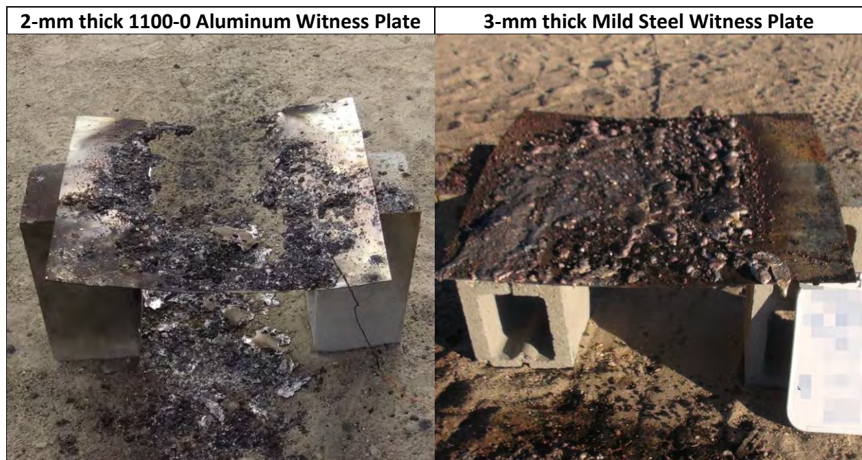
Photo 75: Suspended, Unconfined Package Test Results for Fine Al-CuO Thermite - Mix ID #4 (SMS mixed)
