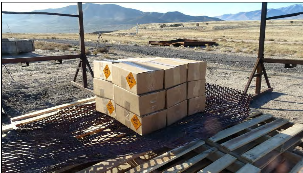
Photo 19: UN Series 6 (c) External Fire Test Setup for Fine Al-CuO Thermite – Large-Scale Mix ID #4 (SMS mixed)
