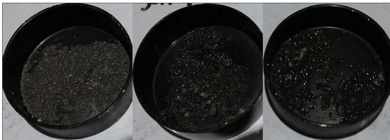
Photo 6: Large-Scale Mix ID #8 Thermite with Coarse Mg & Al and MoO 3 & CuO as Fine (left), Medium (center), Coarse (right)
