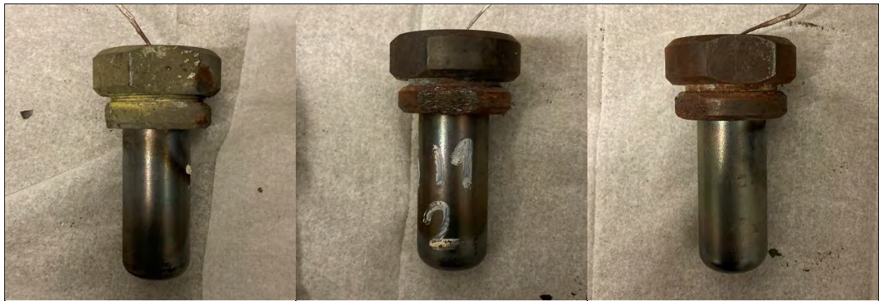
Photo 23: Koenen Test Results for SS #19 Al-SnO 2 , Trials 1 - 3 (left to right)
