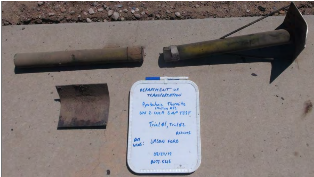
Photo 38: UN 2-in Gap Test Results for Fine Mg&Al-MoO 3 -CuO Thermite - Mix ID #8 (SMS mixed)
