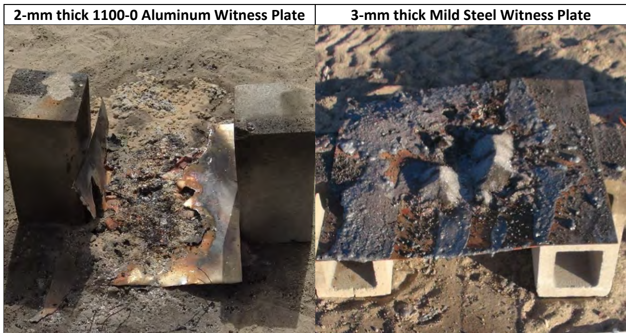
Photo 73: Suspended, Unconfined Package Test Results for Coarse Al-Fe 2 O 3 Thermite A - Mix ID #2 (Commercial)
