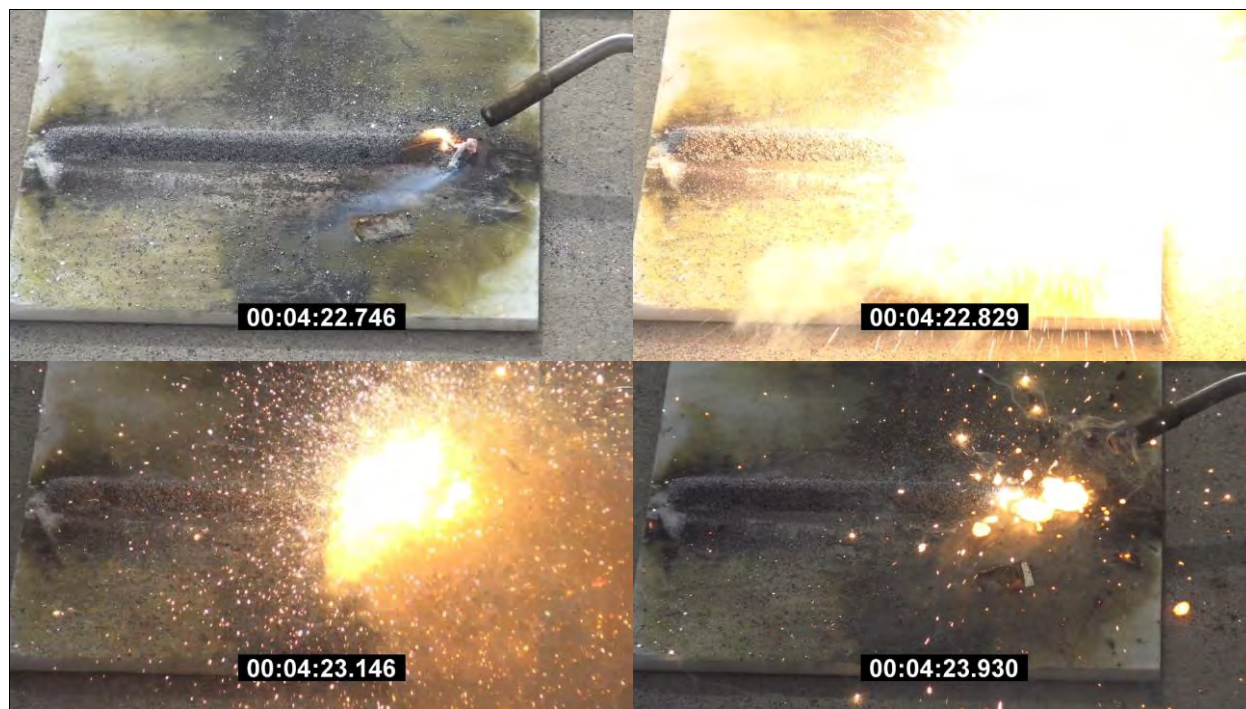
Photo 104: Readily Combustible Test Results - Gas Torch & Magnesium Strip for Coarse \text{Al-Fe}_2\text{O}_3 Thermite A - Mix ID #2 (Commercial) with Ignition without Propagation
