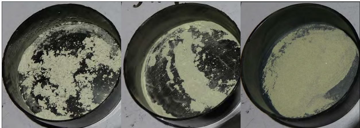
Photo 20: Small-Scale Mix ID #24 Thermite with Medium Al and \text{Bi}_2\text{O}_3 as Fine (left), Medium (center), Coarse (right)
