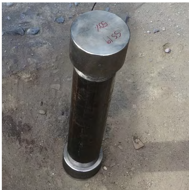
Photo 26: Internal Ignition Test Setup for the Thick-walled Steel Tube at 50% Fill – Typical
