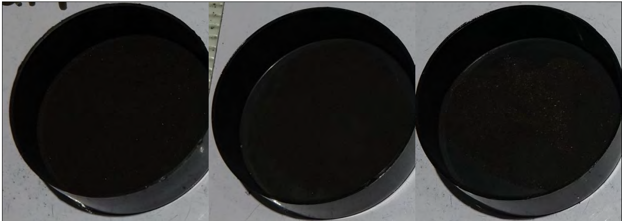
Photo 9: Small-Scale Mix ID #3B Thermite with Coarse Ti and MnO 2 as Fine (left), Medium (center), Coarse (right)
