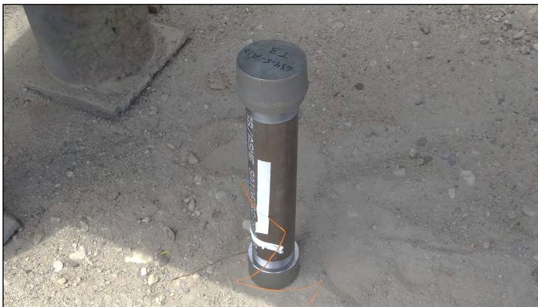
Photo 16: UN Series 1/2 (c) (ii) Internal Ignition Test Setup – typical
