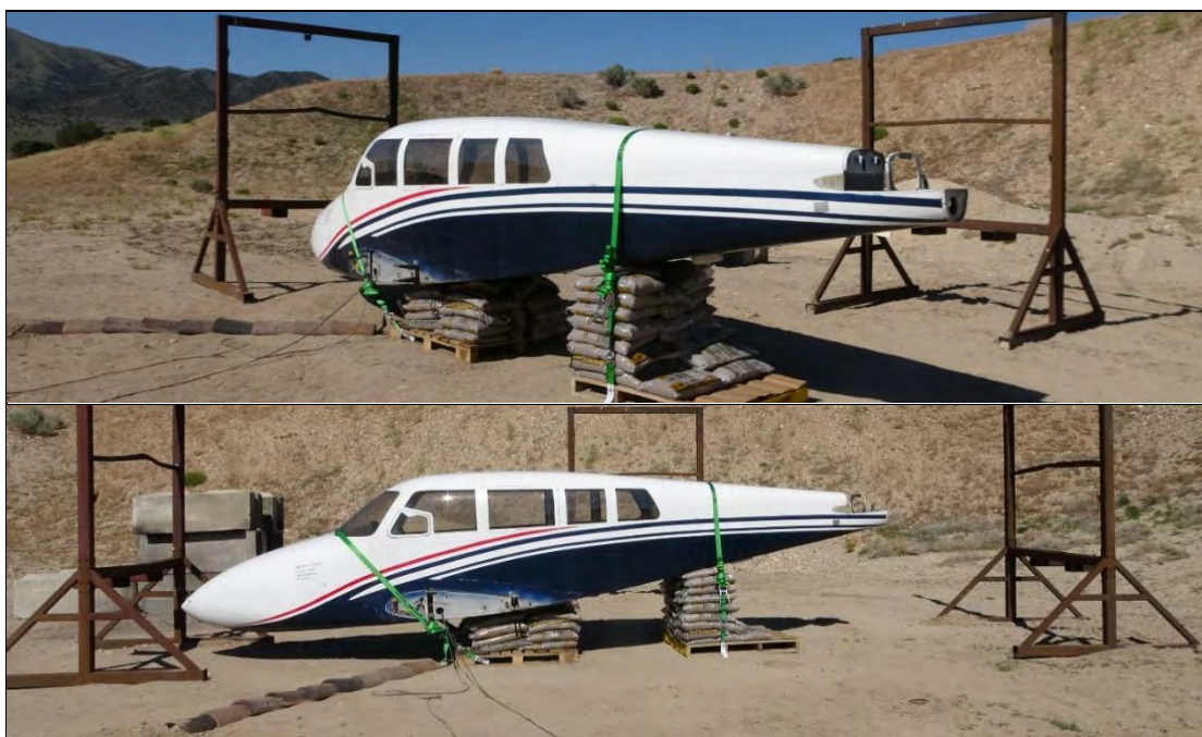
Photo 12: Final Test Setup for the Airplane Fuselage
