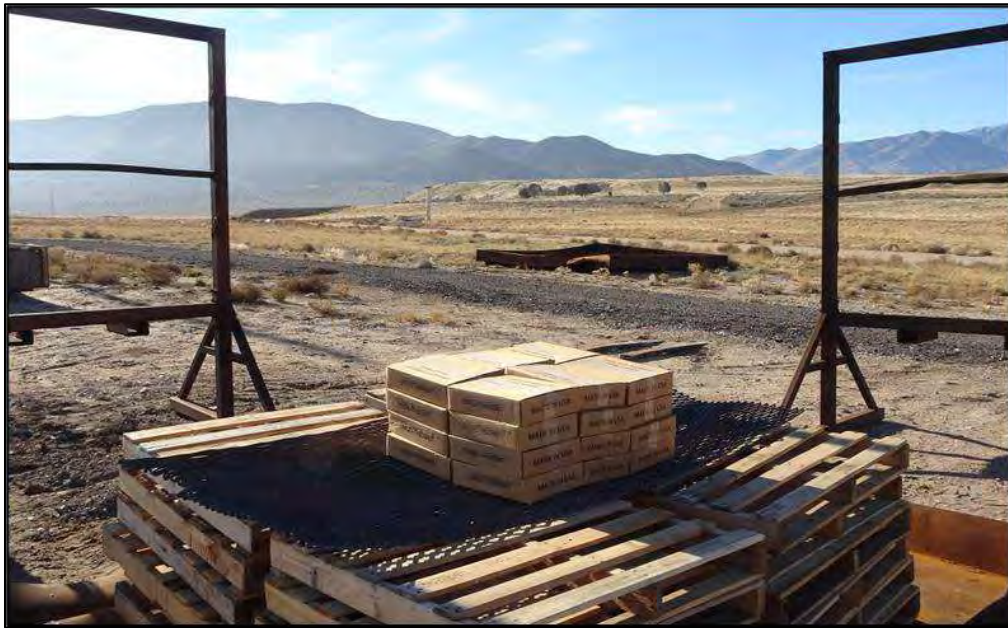
Photo 18: UN Series 6 (c) External Fire Test Setup for Coarse Al-Fe 2 O 3 Thermite B – Large-Scale Mix ID #3 (Commercial)
