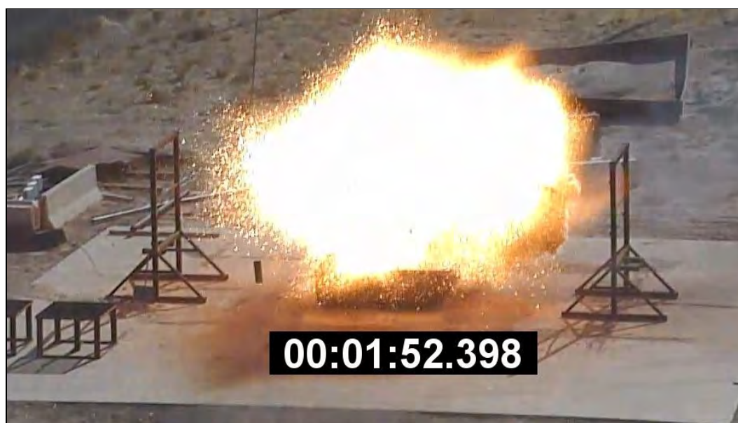
Photo 92: External Bonfire #4 Test Progression - Burning of Fine Al-Fe 2 O 3 Thermite - Mix ID #1 (SMS mixed)
