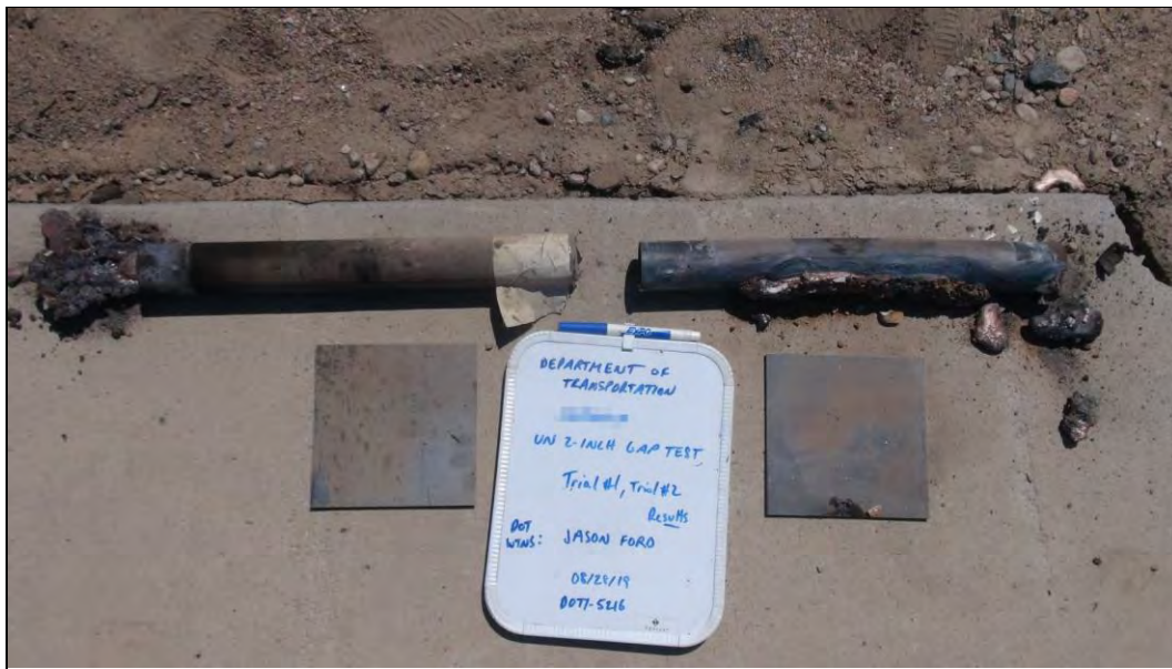
Photo 35: UN 2-in Gap Test Results for Medium Al-CuO Thermite - Mix ID #5 (Commercial)
