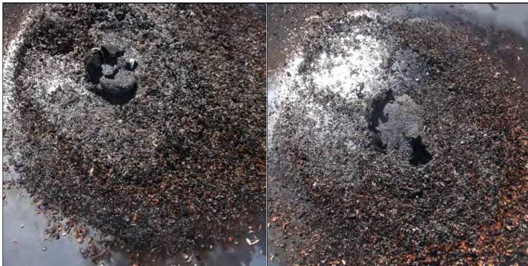
Photo 66: Small-scale Burning Test Results for Medium Al-CuO Thermite - Mix ID #5 (Commercial)
