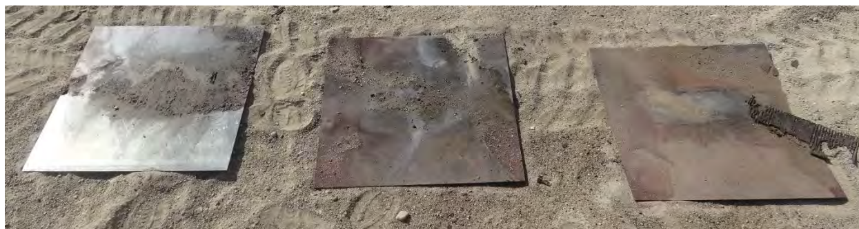
Photo 13: UN Series 6 (a) Single Package Test Results for Fine Al-CuO Thermite – Large-Scale Mix ID #4 (SMS mixed)
