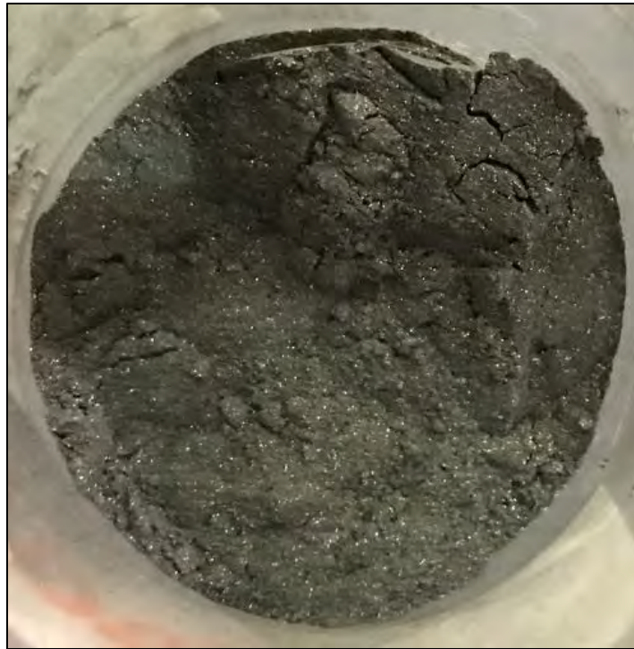
Photo 53: Fine Mg&Al-MoO 3 -CuO – Small-Scale Mix ID #56
