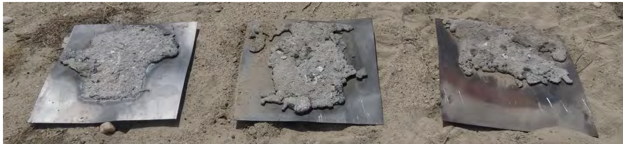
Photo 11: UN Series 6 (a) Single Package Test Results for Coarse \text{Al-Fe}_2\text{O}_3 Thermite A – Large-Scale Mix ID #2 (Commercial)
