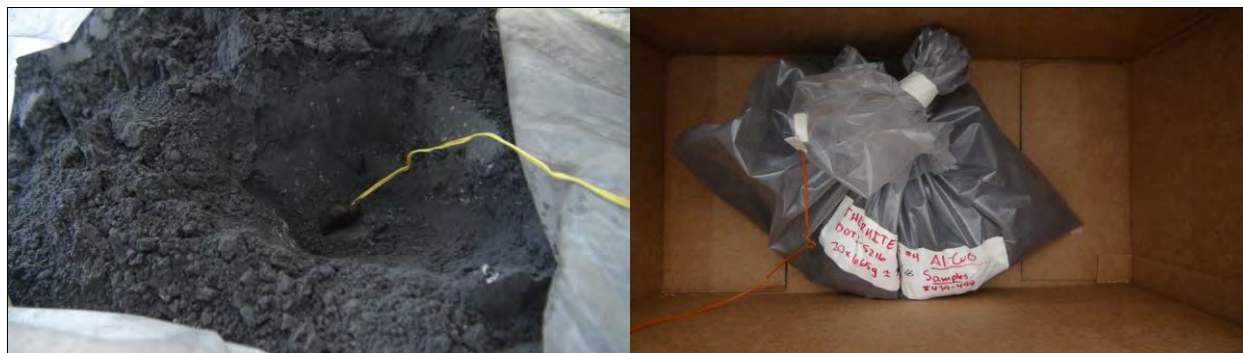
Photo 70: Unconfined Single Package Test Setup for Fine Al-CuO Thermite - Mix ID #4 (SMS mixed) - typical
