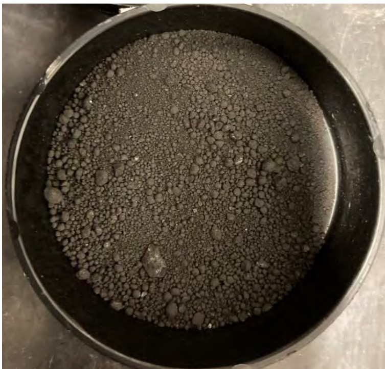
Photo 25: Fine Al-Fe 3 O 4 – Small-Scale Mix ID #27
