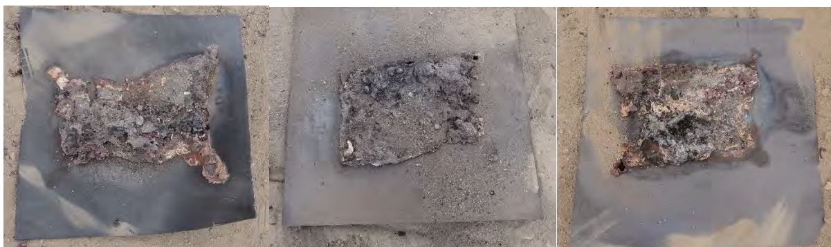
Photo 14: UN Series 6 (a) Single Package Test Results for Medium Al-CuO Thermite – Large-Scale Mix ID #5 (Commercial)
