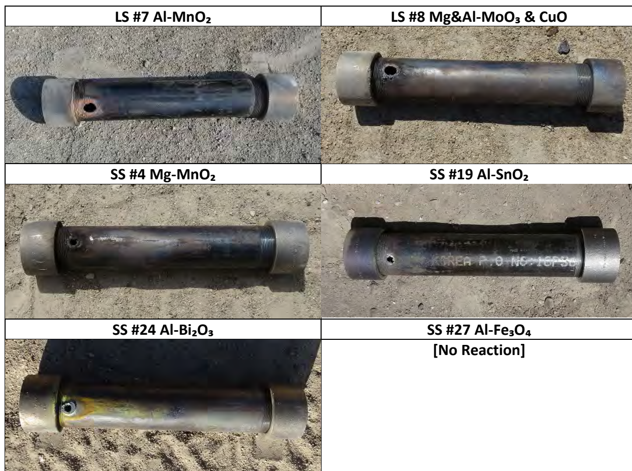
Photo 25: Internal Ignition Test Results for the Thick-walled Steel Tube at 25% Fill
