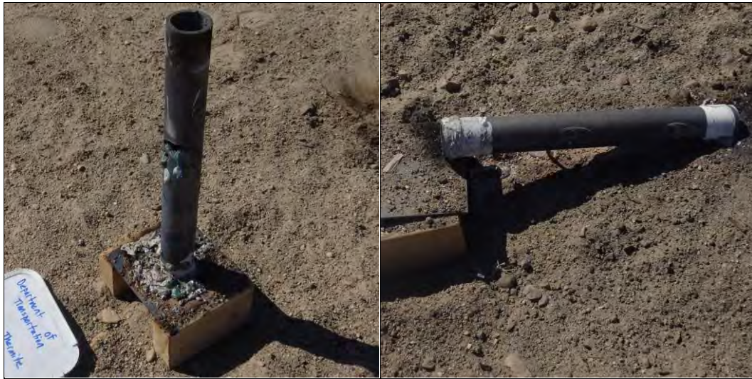
Photo 36: UN 2-in Gap Test Results for Fine Al-Ni 2 O 3 Thermite - Mix ID #6 (SMS mixed)
