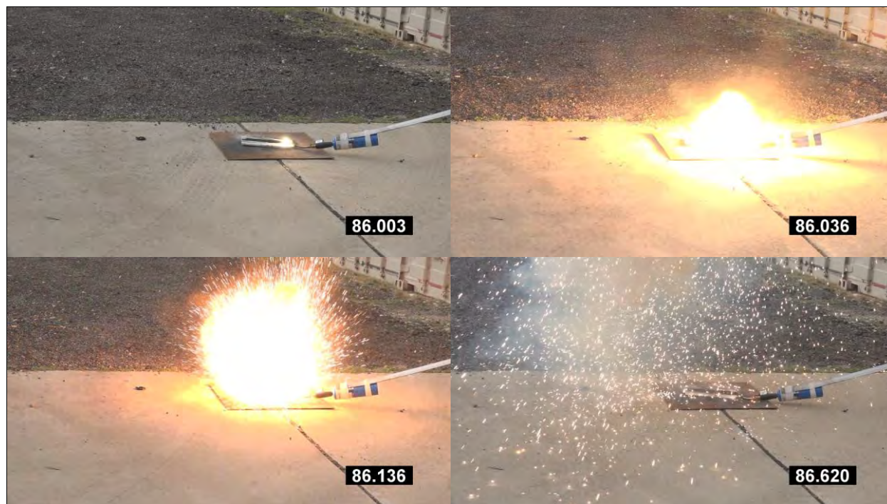
Photo 111: Readily Combustible Test Results - Gas Torch for Fine Al-MnO 2 Thermite - Mix ID #7 (SMS mixed) with Ignition and Explosion
