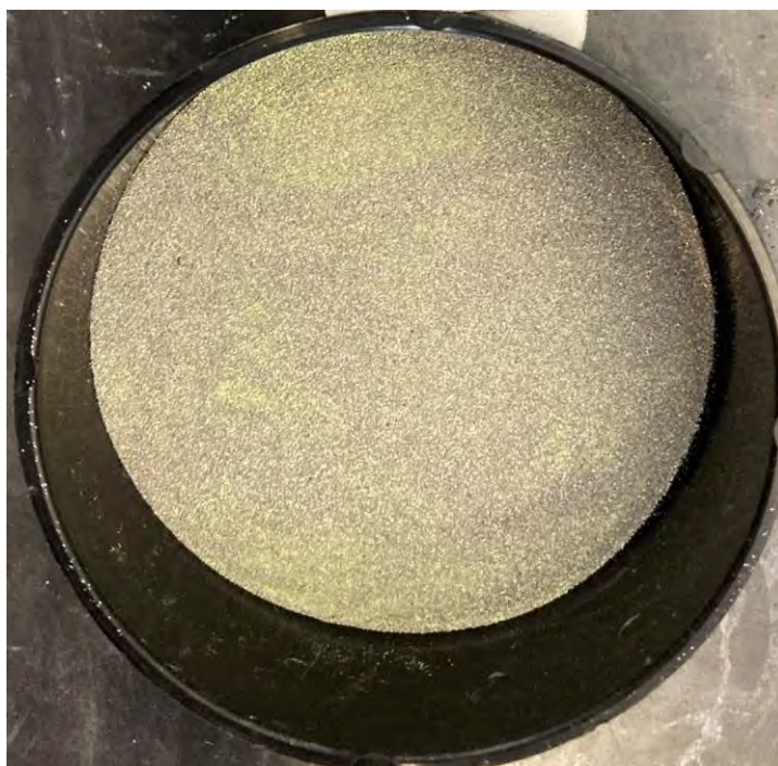
Photo 42: Fine Mg-WO 3 – Small-Scale Mix ID #45
