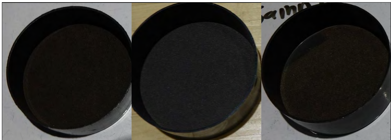
Photo 11: Scale-Scale Mix ID #4 Thermite with Medium Mg and MnO 2 as Fine (left), Medium (center), Coarse (right)
