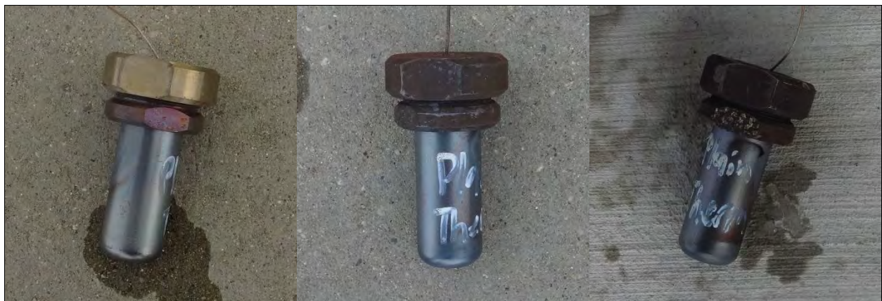
Photo 16: Koenen Test Results for LS #2 Al-Fe 2 O 3 , Trials 1 - 3 (left to right)
