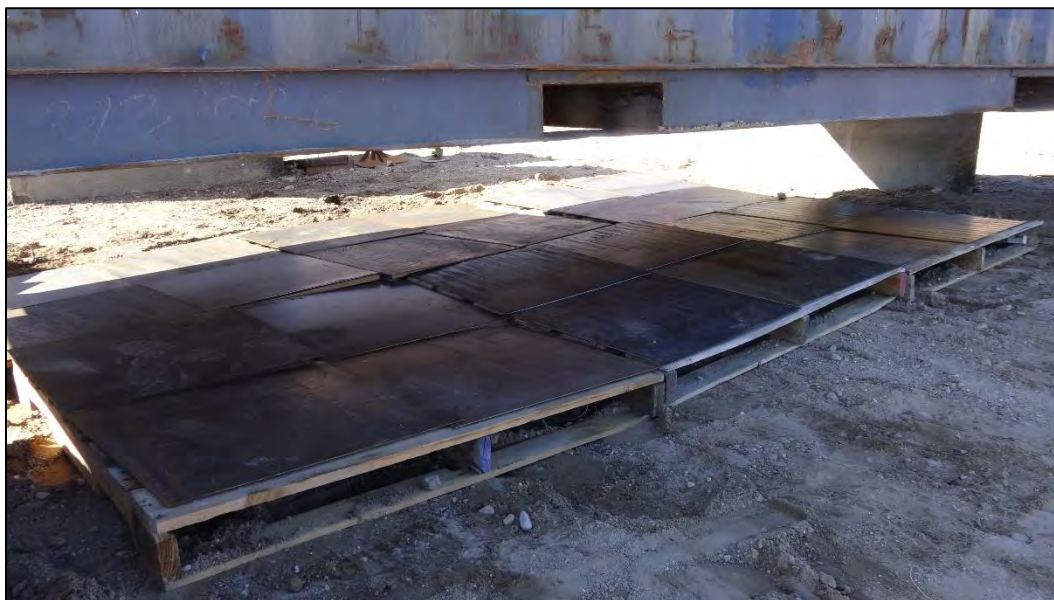
Photo 26: Grid of Steel Witness Plates Underneath the Shipping Container
