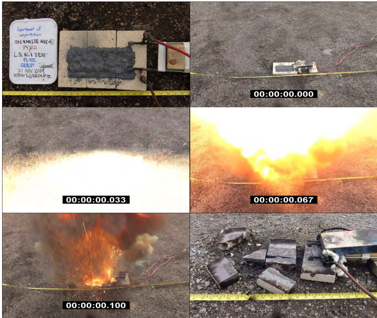
Photo 147: Large-Scale Readily Combustible Test Results - Hot Wire on Plate for Fine Mg&Al-MoO 3 -CuO Thermite - Mix ID #8 (SMS mixed) with Explosion
