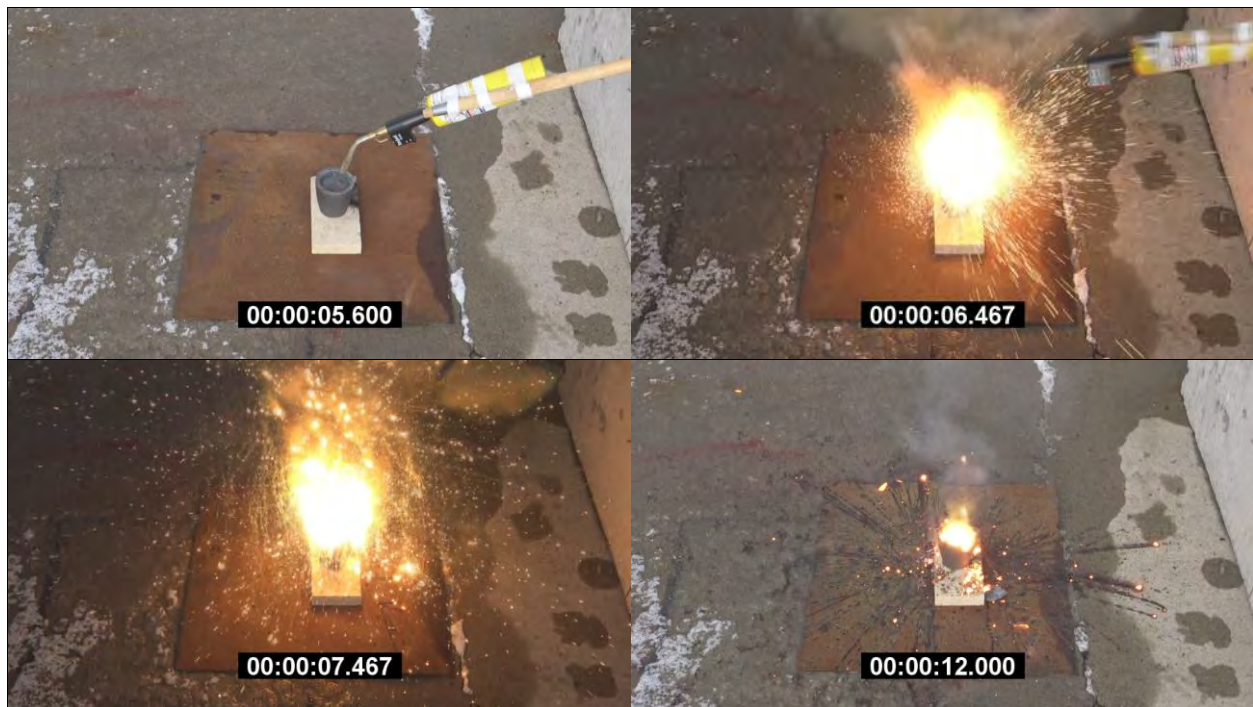
Photo 139: Large-Scale Readily Combustible Test Results - Gas Torch (aided by a thermite starting powder) in Crucible for Medium Al-CuO Thermite - Mix ID #5 (Commercial) with Ignition and Full Propagation over 6.4 seconds
