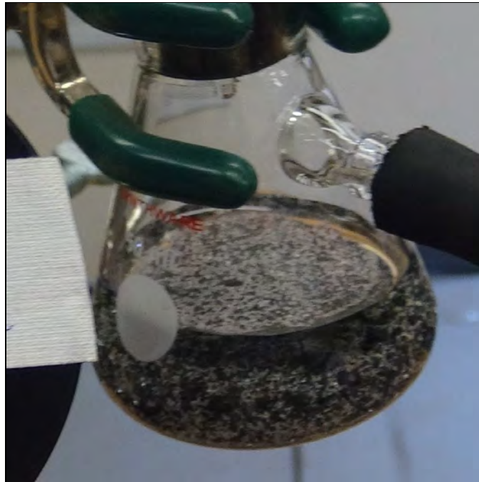
Photo 153: UN Test N.5 Test Results for Coarse Al-Fe 2 O 3 Thermite B - Mix ID #3 (Commercial)
