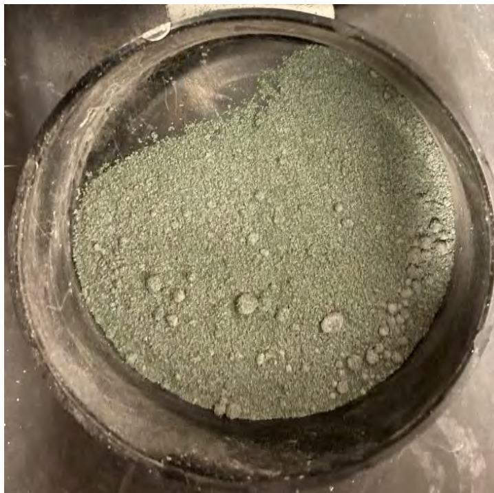
Photo 12: Fine Al-MnO – Small-Scale Mix ID #29
