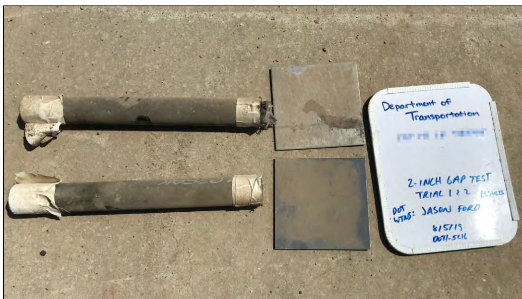
Photo 33: UN 2-in Gap Test Results for Coarse Al-Fe 2 O 3 Thermite B - Mix ID #3 (Commercial)
