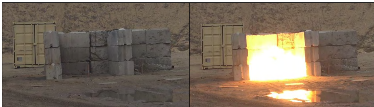
Photo 18: Internal Ignition Test Results (Explosion) for SS #48 Ti-Bi 2 O 3 in the Thin Fiberboard Tube
