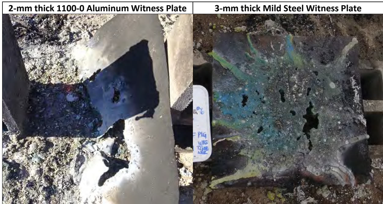
Photo 77: Suspended, Unconfined Package Test Results for Fine \text{Al-Ni}_2\text{O}_3 Thermite - Mix ID #6 (SMS mixed)
