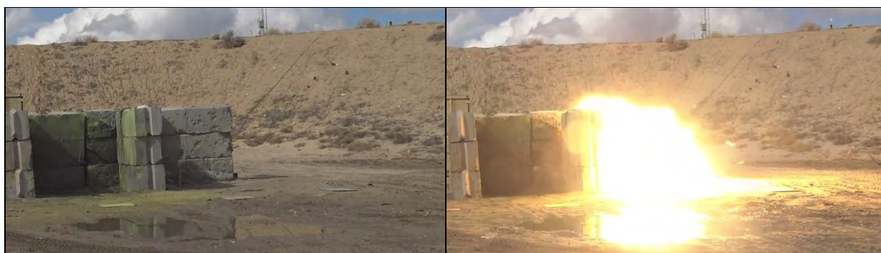
Photo 13: Internal Ignition Test Results (Explosion) for SS #4 Mg-MnO 2 in the Thin Fiberboard Tube
