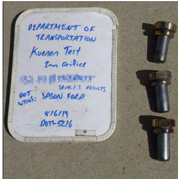
Photo 44: Koenen Test Results for Coarse Al-Fe 2 O 3 Thermite B - Mix ID #3 (Commercial)
