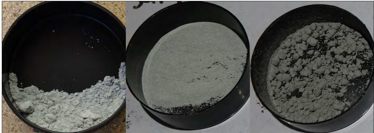
Photo 13: Small-Scale Mix ID #9 Thermite with Fine Al and \text{MoO}_3 as Fine (left), Medium (center), Coarse (right)
