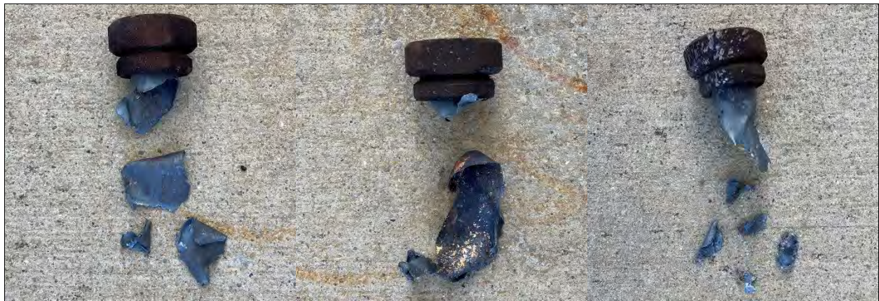
Photo 17: Koenen Test Results for LS #4 Al-CuO, Trials 1 - 3 (left to right)
