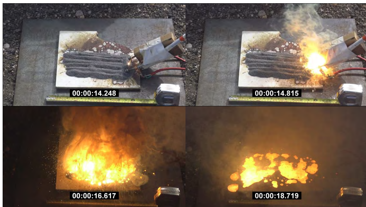
Photo 138: Large-Scale Readily Combustible Test Results - Hot Wire on Plate for Medium Al-CuO Thermite - Mix ID #5 (Commercial) with Ignition and Full Propagation over 2.4 seconds
