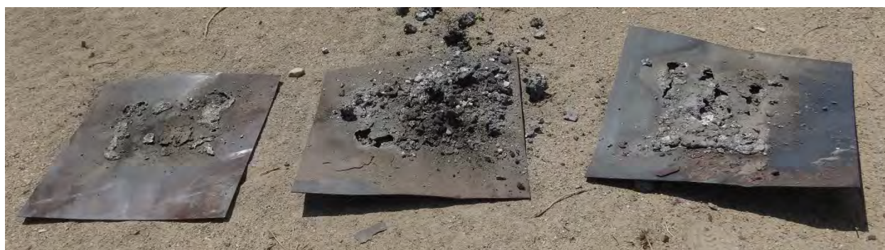
Photo 15: UN Series 6 (a) Single Package Test Results for Fine Al-Ni 2 O 3 Thermite – Large-Scale Mix ID #6 (SMS mixed)
