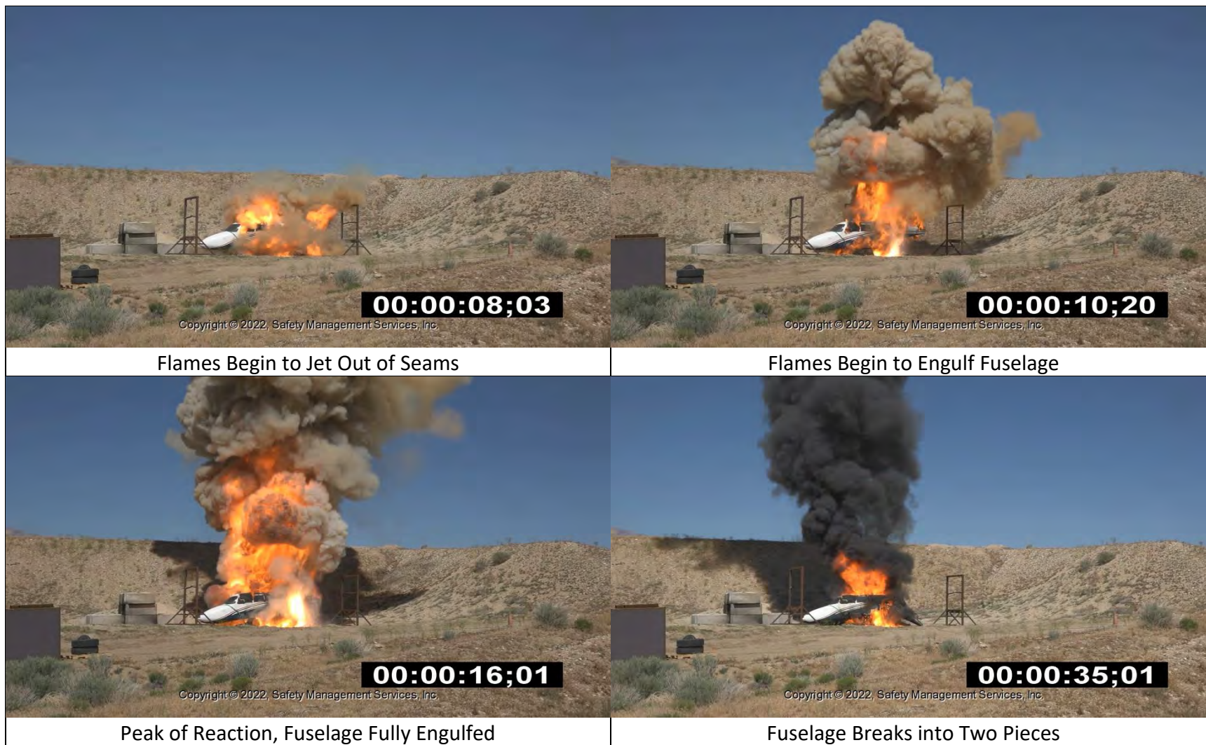
Photo A2: Reaction Progression for the 1200-lb Stack Test in an Airplane Fuselage
