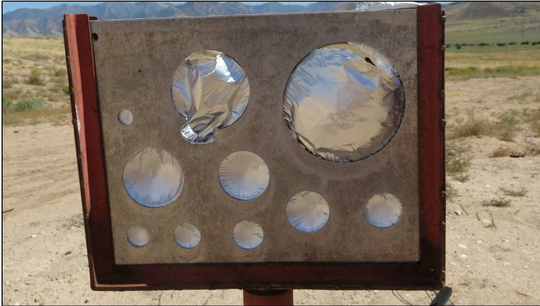
Photo 27: Bikini Gages Ruptured by the Blast of LS #4-5-C30 (two largest holes)
