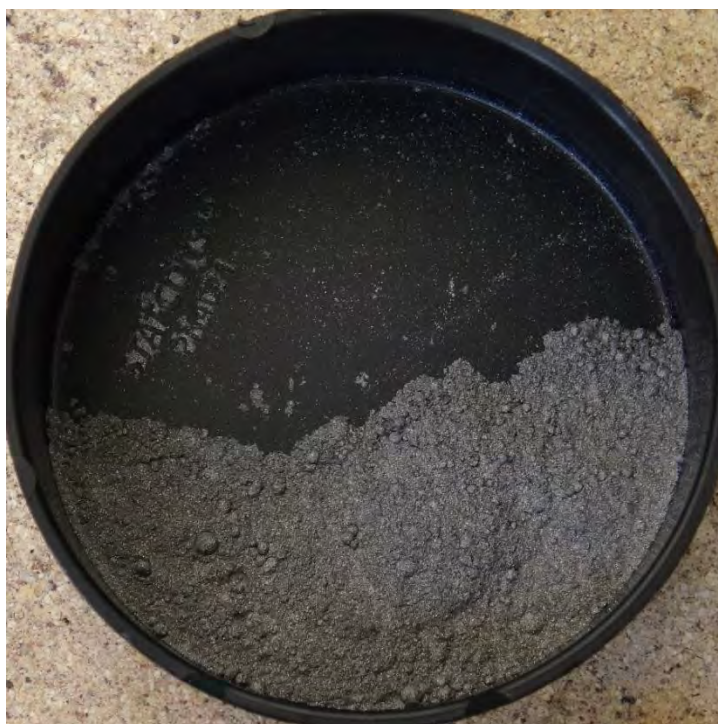
Photo 3: Fine Mg-MnO 2 Thermite – Small-Scale Mix ID #4 (SMS mixed)
