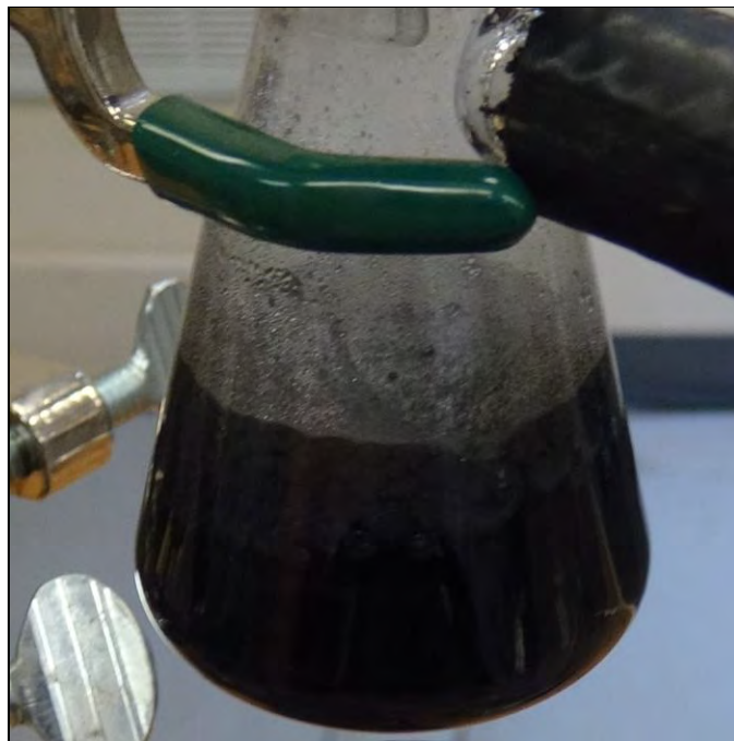
Photo 158: UN Test N.5 Test Results for Fine Mg&Al-MoO 3 -CuO Thermite - Mix ID #8 (SMS mixed)
