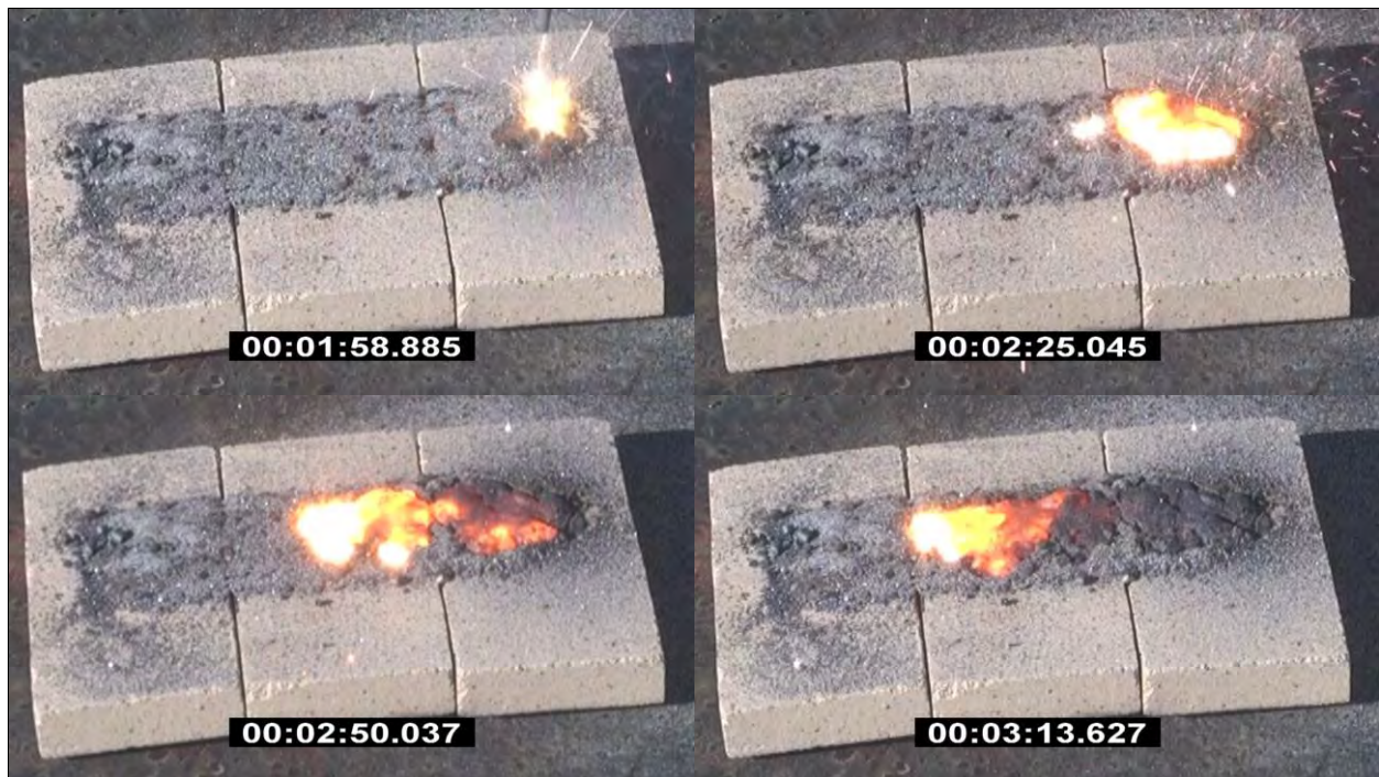
Photo 132: Large-Scale Readily Combustible Test Results - Acetylene Torch on Plate for Coarse Al-Fe 2 O 3 Thermite B - Mix ID #3 (Commercial) with Ignition and Partial Consumption over 75 seconds
