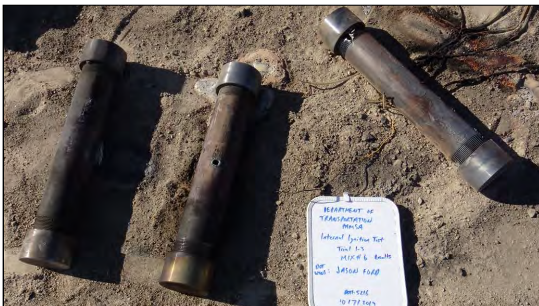
Photo 56: Internal Ignition Test Results for Fine Al-Ni 2 O 3 Thermite - Mix ID #6 (SMS mixed)
