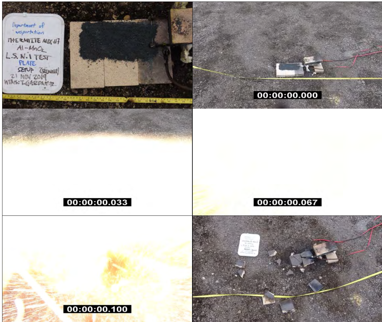
Photo 144: Large-Scale Readily Combustible Test Results - Hot Wire on Plate for Fine Al-MnO 2 Thermite - Mix ID #7 (SMS mixed) with Explosion
