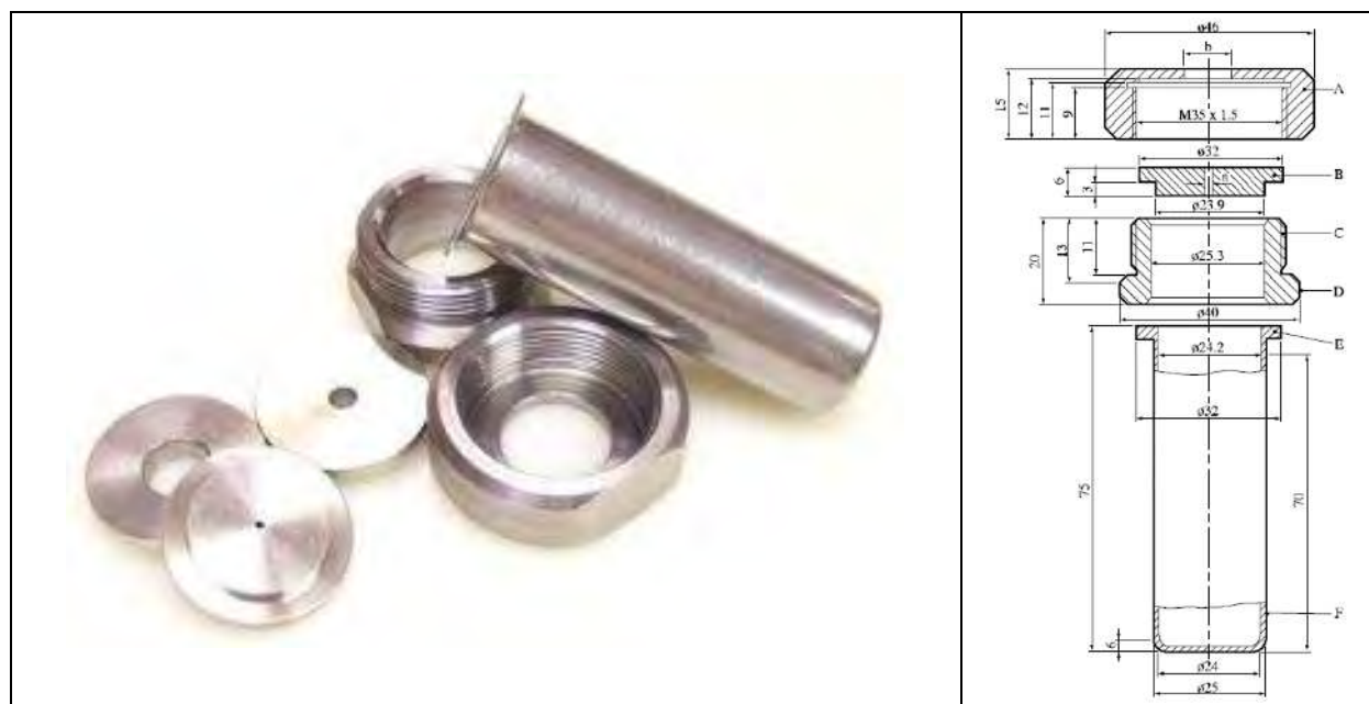
Figure 1: Koenen Tube, Orifices, Plate, and Reusable Closing Device
