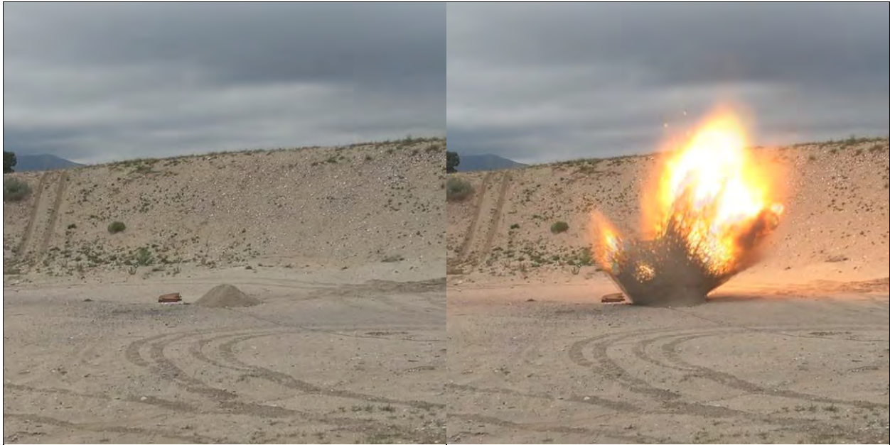
Photo 6: Explosion of Fine Al-MnO 2 Thermite – Large-Scale Mix ID #7 (SMS mixed) in the UN Series 6 (a) Single Package Test
