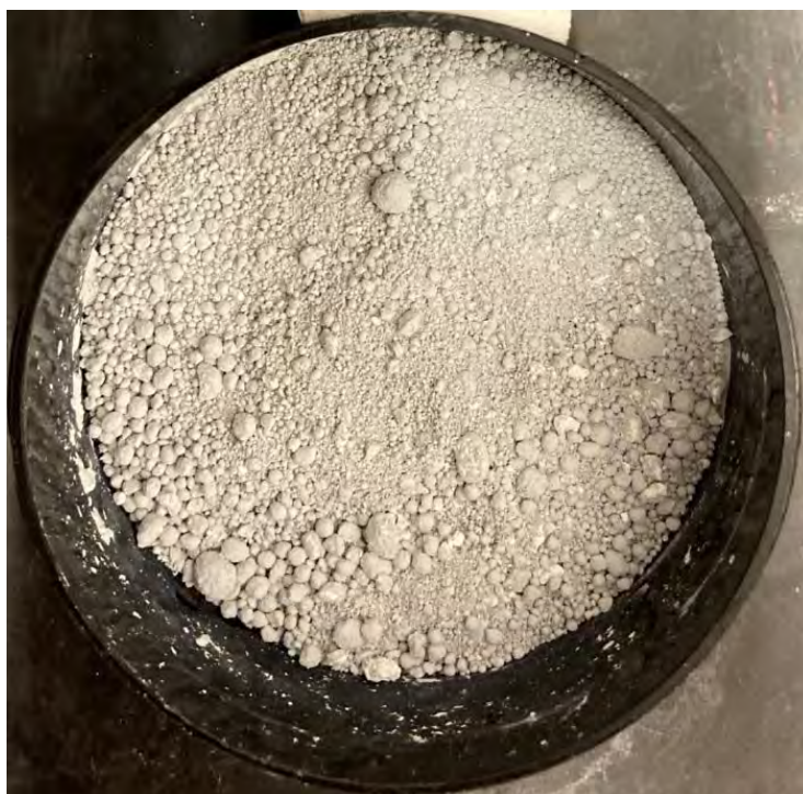
Photo 32: Fine Al-ZnO – Small-Scale Mix ID #34
