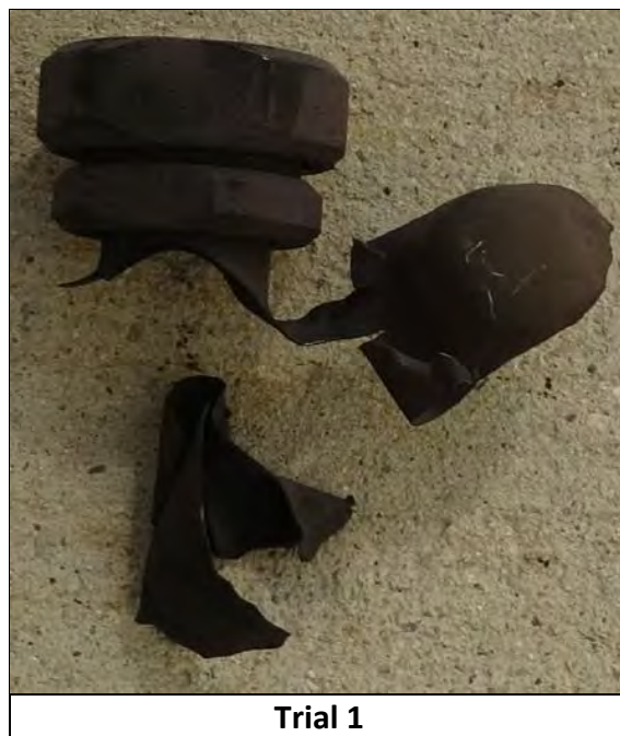
Photo A 4: LS #4-5-A30 Koenen Test Results
