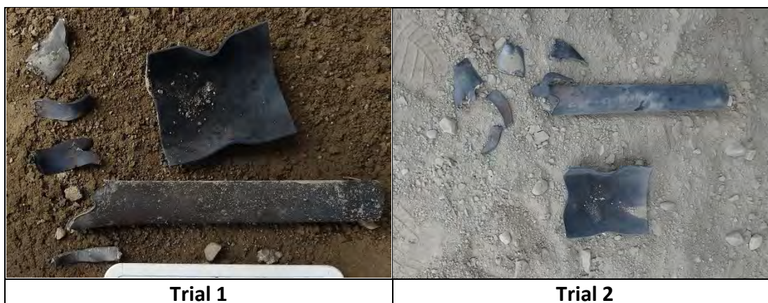
Photo 8: Large-Scale #1-6-A30 UN 1 (a) Zero Gap Test Results
