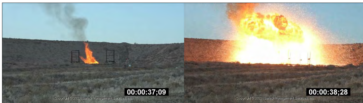
Photo 24: UN Series 6 (c) External Fire – Test Progression for Fine Al-Fe 2 O 3 Thermite – Large-Scale Mix ID #1 (SMS mixed)
