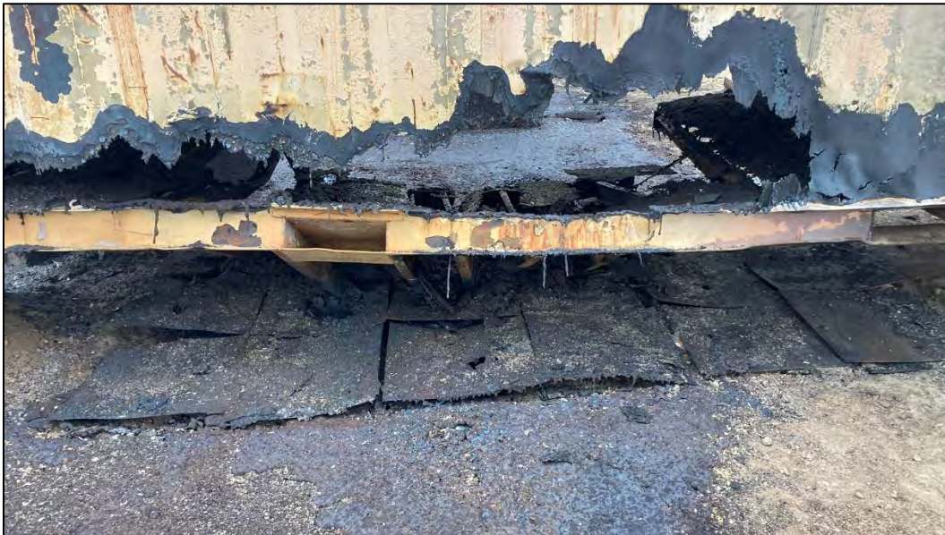
Photo 33: Intermodal Container Test Results - Damaged Siding and Witness Plates
