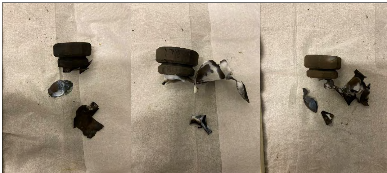
Photo 21: Koenen Test Results for SS #4 Mg-MnO 2 , Trials 1 - 3 (left to right)
