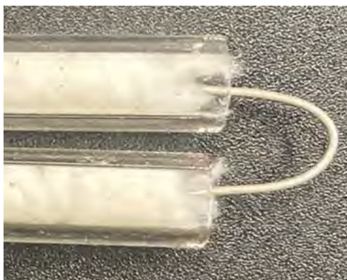
Photo 9: Insulated Nichrome Hotwire Igniter – Typical
