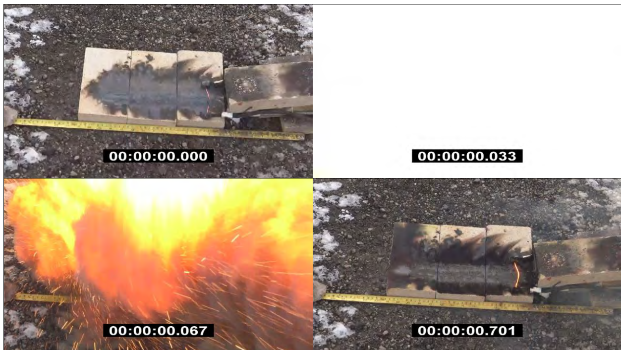
Photo 121: Readily Combustible Test Results - Hot Wire for Fine Mg&Al-MoO 3 -CuO Thermite - Mix ID #8 (SMS mixed) with Explosion
