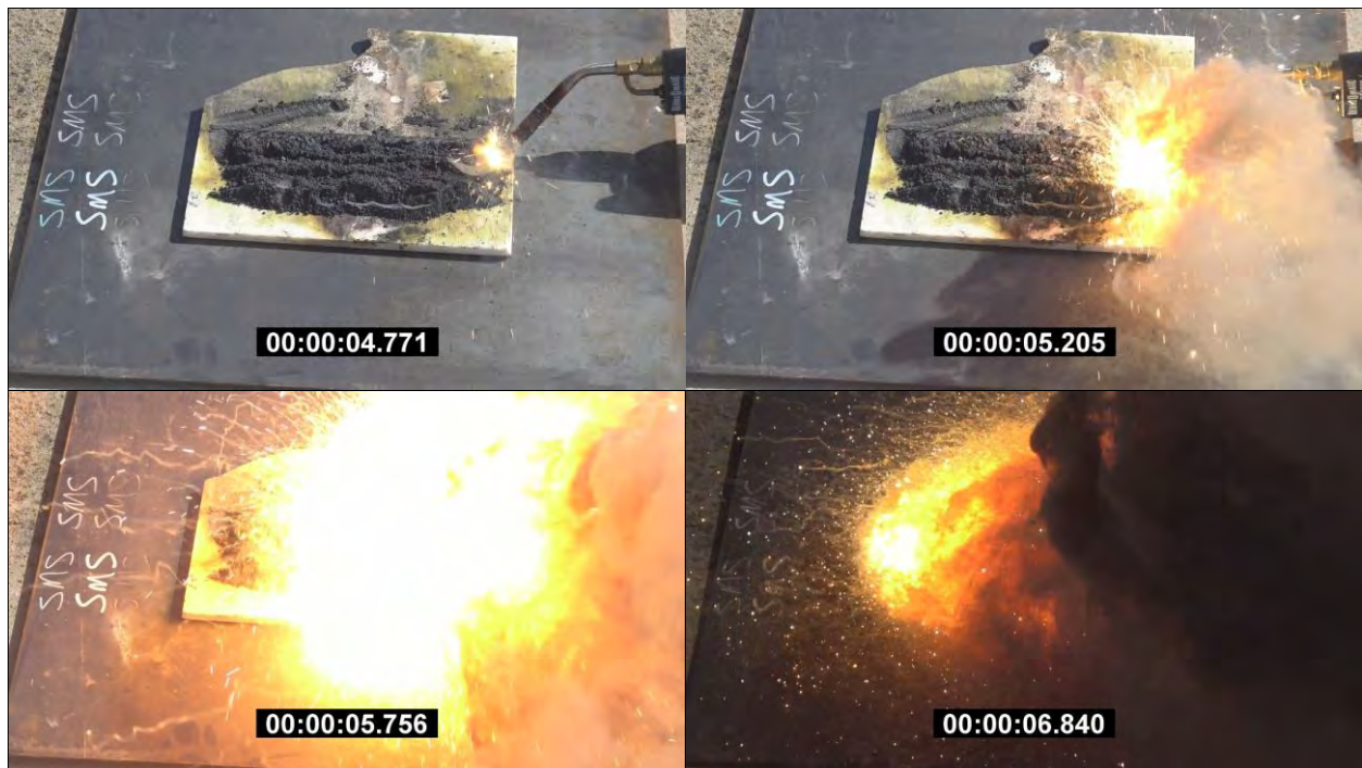
Photo 134: Large-Scale Readily Combustible Test Results - Gas Torch on Plate for Fine Al-CuO Thermite - Mix ID #4 (SMS mixed) with Ignition and Full Consumption over 2.1 seconds
