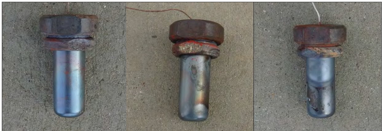
Photo 15: Koenen Test Results for LS #1 Al-Fe 2 O 3 , Trials 1 - 3 (left to right)
