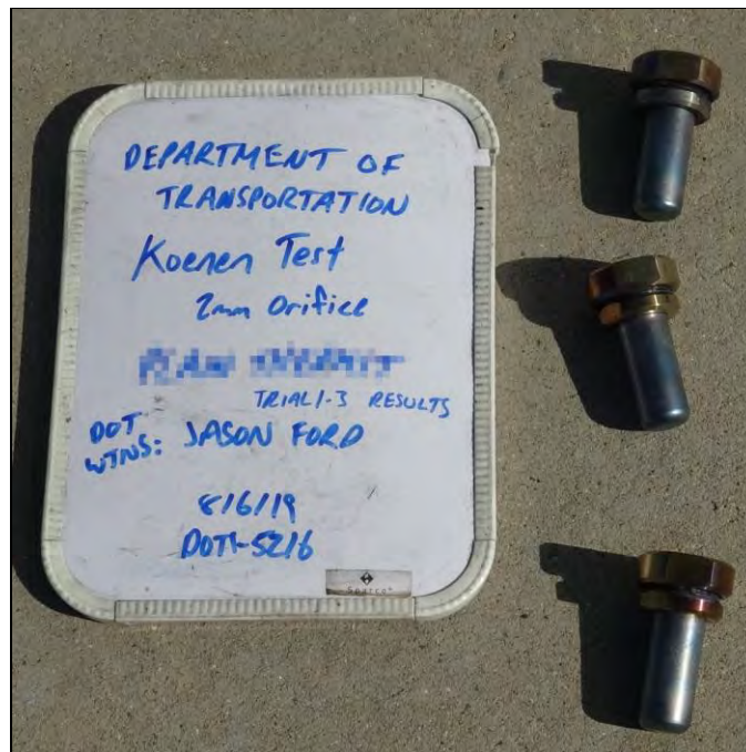
Photo 43: Koenen Test Results for Coarse \text{Al-Fe}_2\text{O}_3 Thermite A - Mix ID #2 (Commercial)
