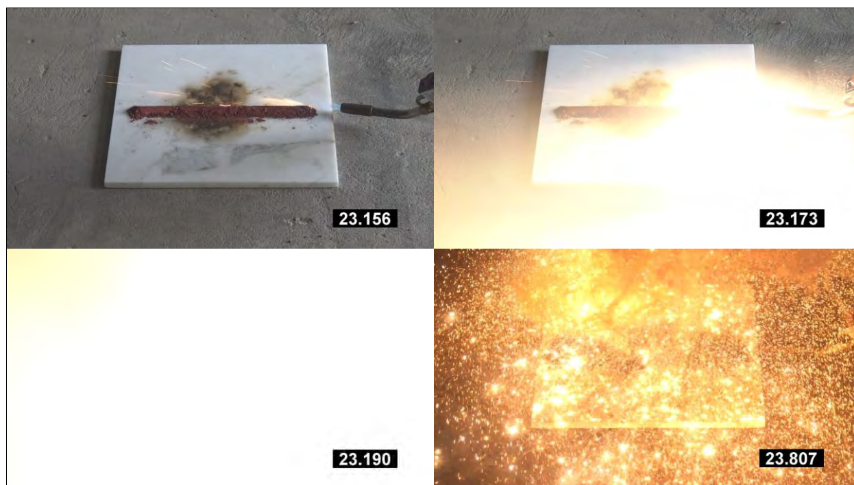
Photo 102: Readily Combustible Test Results - Gas Torch for Fine Al-Fe 2 O 3 Thermite - Mix ID #1 (SMS mixed) with Ignition and Rapid Burning
