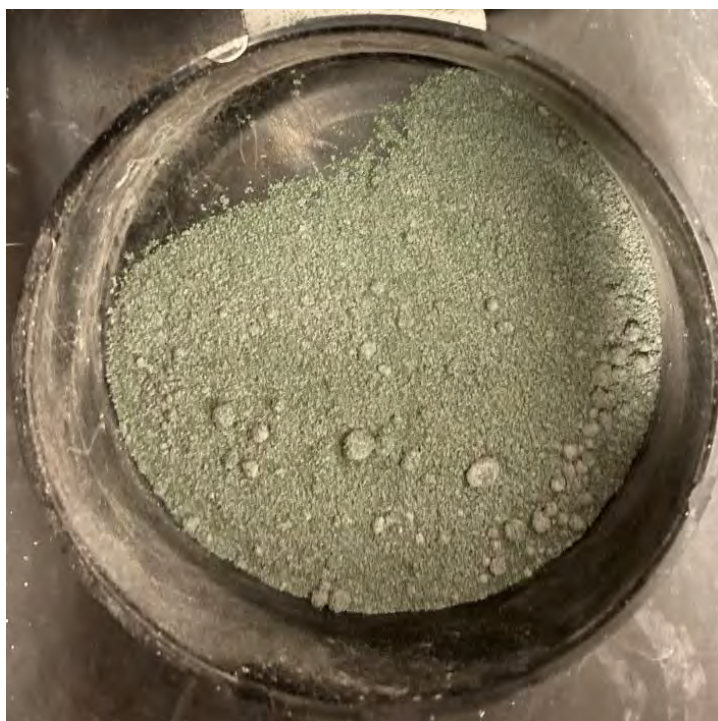
Photo 27: Fine Al-MnO – Small-Scale Mix ID #29
