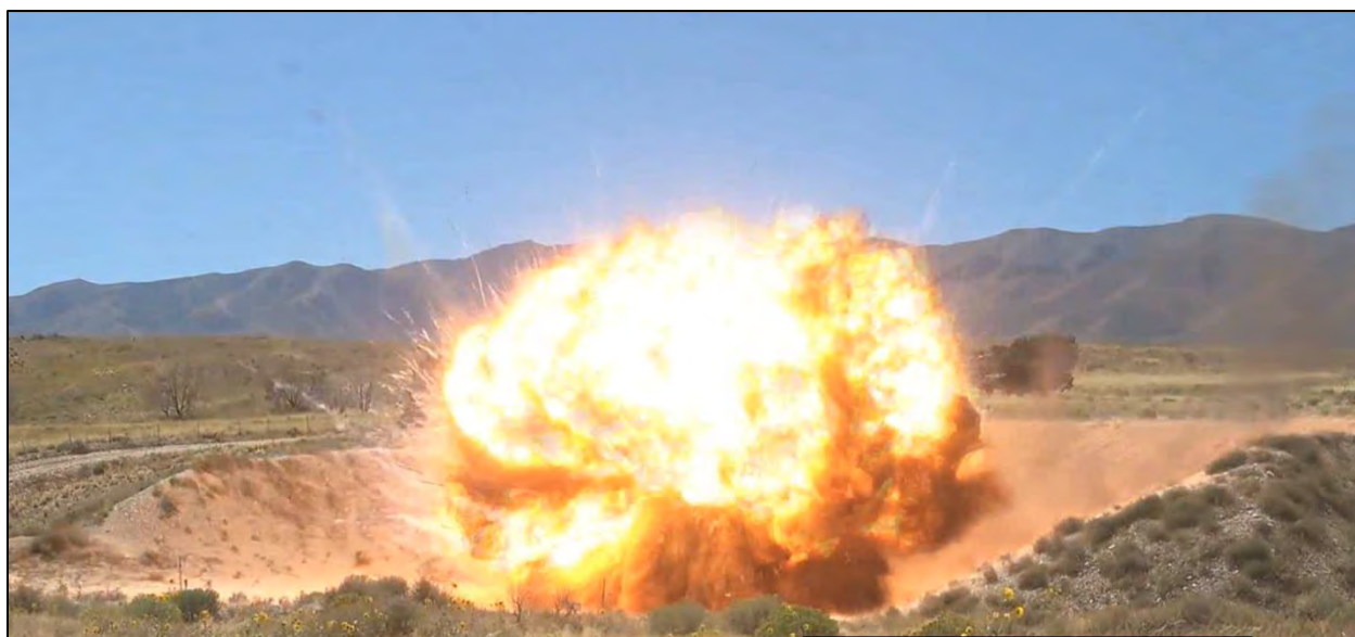
Photo 26: LS #4-5-C30 UN Series 6 (c) External Fire Reaction
