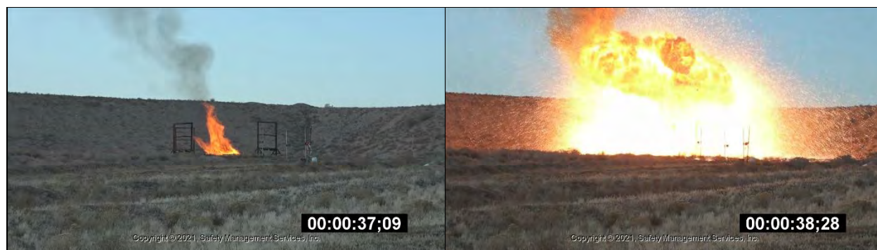
Photo 1: Task 4, UN Series 6 (c) External Fire – Test Progression for Fine \text{Al-Fe}_2\text{O}_3 Thermite – Large-Scale Mix ID #1 (SMS mixed)
