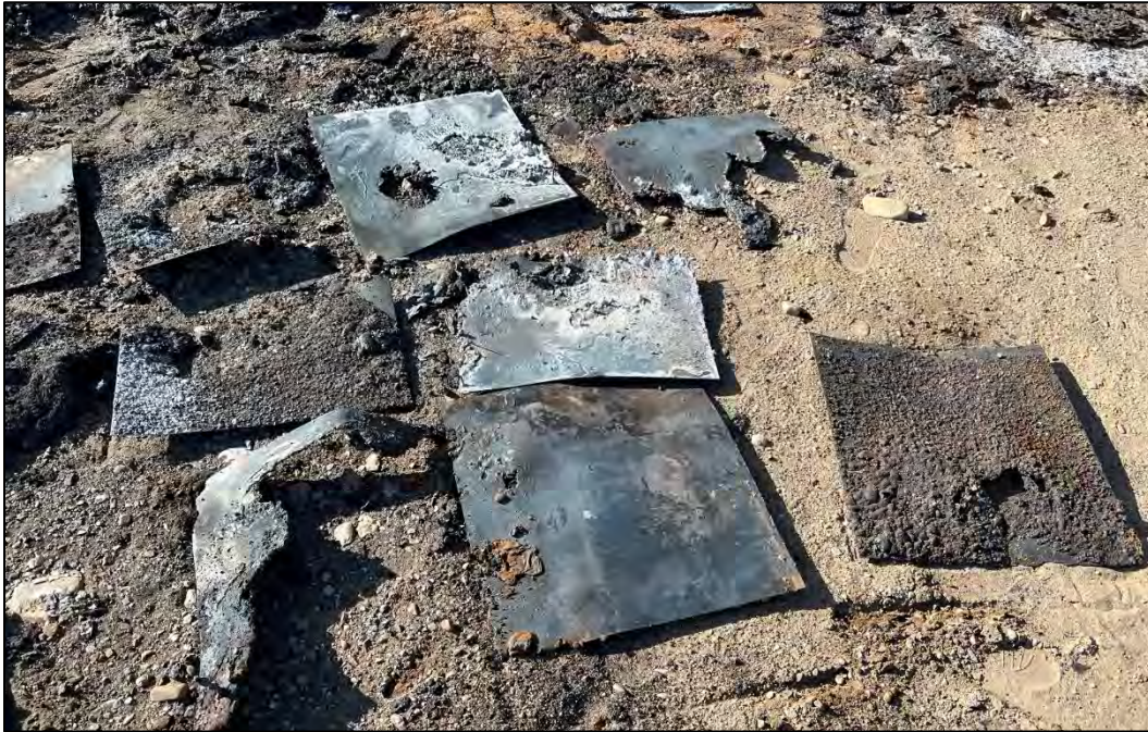
Photo 35: Intermodal Container Test Results - Damaged Witness Plates (typical)
