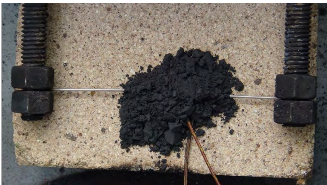
Photo 160: Test Sample Loaded onto Hotwire Auto-ignition Temperature Apparatus
