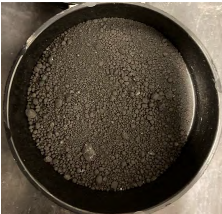
Photo 11: Fine Al-Fe 3 O 4 – Small-Scale Mix ID #27
