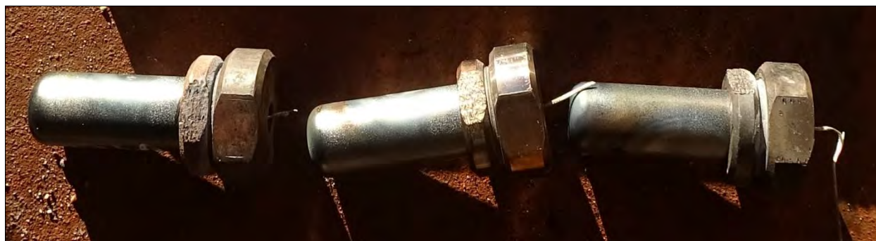
Photo 26: Koenen Test Results for SS #29 Al-MnO, Trials 1 - 3 (left to right)
