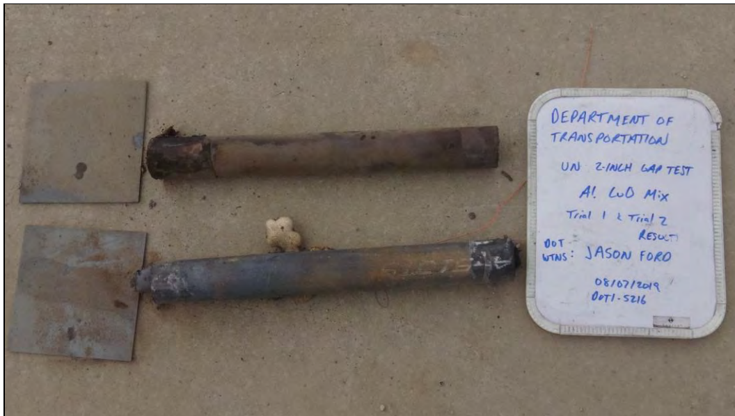
Photo 34: UN 2-in Gap Test Results for Fine Al-CuO Thermite - Mix ID #4 (SMS mixed)
