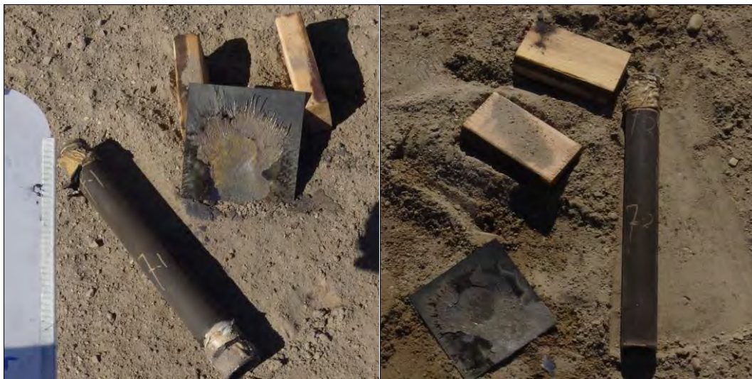
Photo 37: UN 2-in Gap Test Results for Fine Al-MnO 2 Thermite - Mix ID #7 (SMS mixed)
