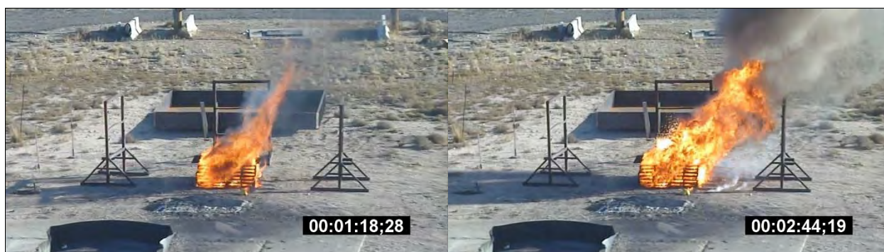
Photo 28: UN Series 6 (c) External Fire – Test Progression for Medium Al-CuO Thermite – Large-Scale Mix ID #5 (Commercial)
