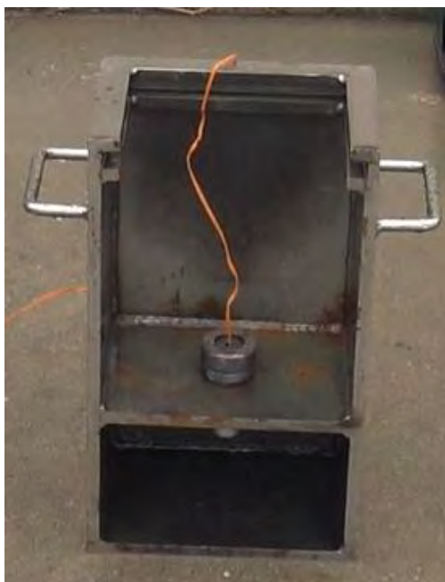
Figure 4: The Bursting Tube Ranking Test Setup
