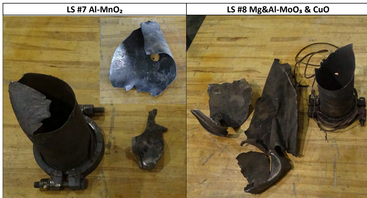
Photo 20: Internal Ignition Test Results (Explosion) for the Thin-walled Steel Tube
