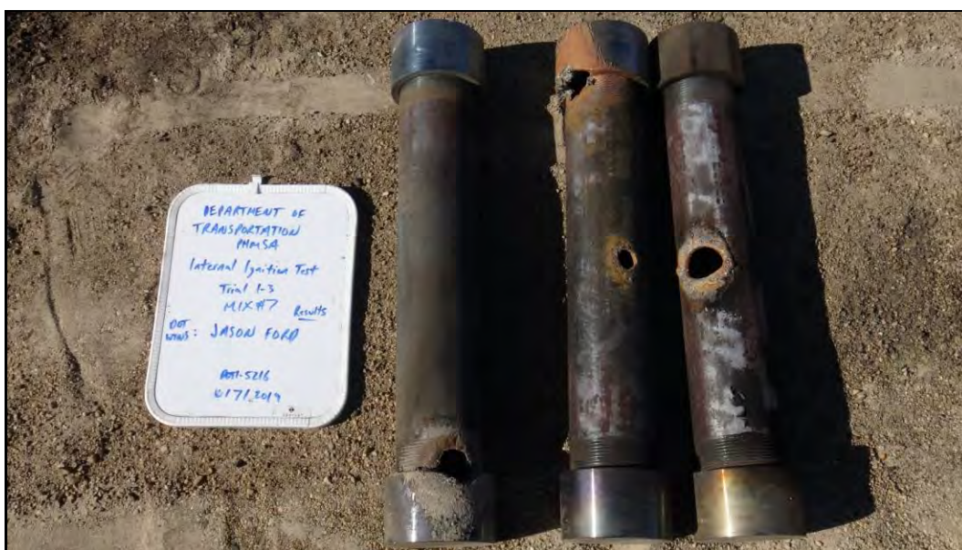
Photo 57: Internal Ignition Test Results for Fine Al-MnO 2 Thermite - Mix ID #7 (SMS mixed)
