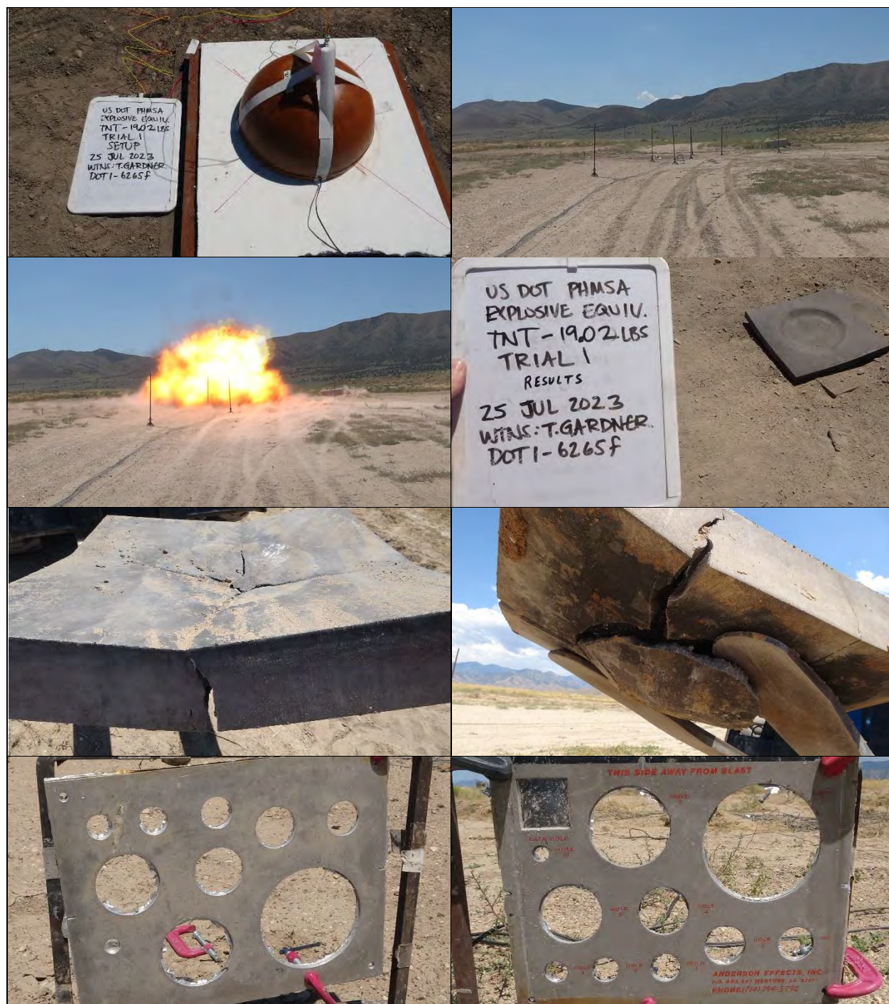
Photo 38: Test Setup and Results for Trial 1 of Cast TNT
