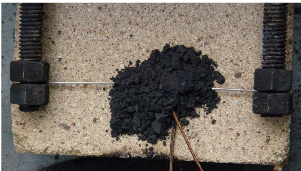
Photo 25: Test Sample Loaded onto Hotwire Auto-ignition Temperature Apparatus
