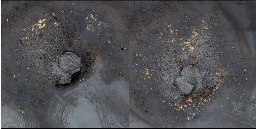
Photo 63: Small-scale Burning Test Results for Coarse Al-Fe 2 O 3 Thermite A - Mix ID #2 (Commercial)
