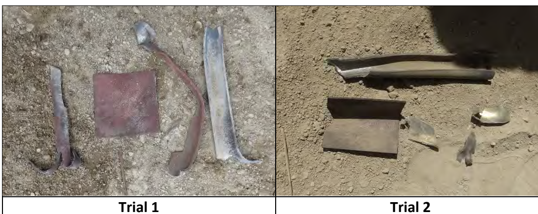
Photo 13: Large-Scale #4-5-D30 UN 1 (a) Zero Gap Test Results
