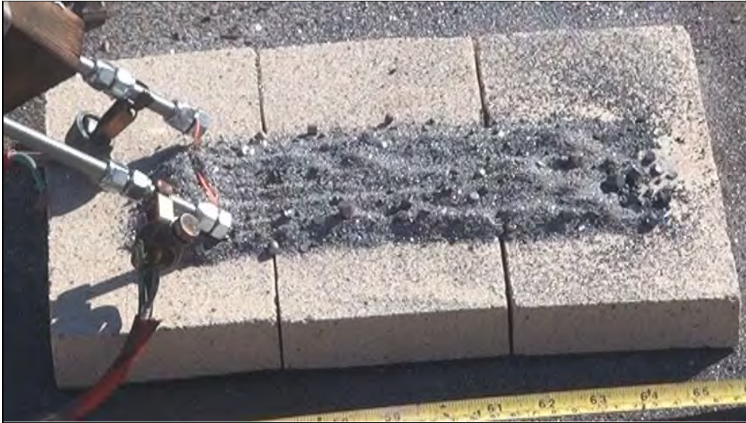
Photo 131: Large-Scale Readily Combustible Test Results - Hot Wire on Plate for Coarse Al-Fe 2 O 3 Thermite B - Mix ID #3 (Commercial) with No Reaction in 5 minutes
