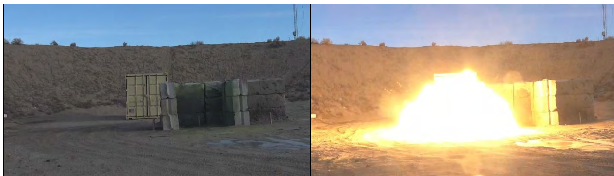
Photo 12: Internal Ignition Test Results (Explosion) for LS #8 Mg&Al-MoO 3 & CuO in the Thin Fiberboard Tube
