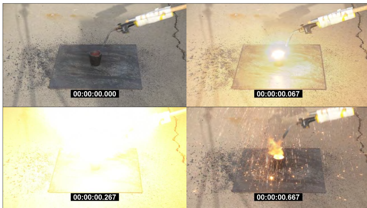
Photo 125: Large-Scale Readily Combustible Test Results - Gas Torch in Crucible for Fine Al-Fe 2 O 3 Thermite - Mix ID #1 (SMS mixed) with Ignition and Full Consumption over 0.5 seconds
