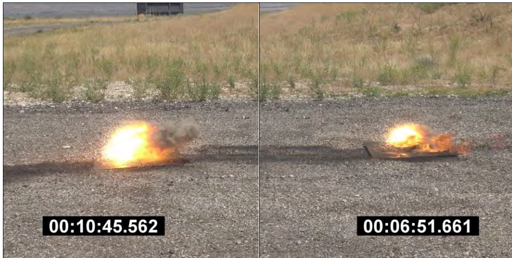
Photo 65: Small-scale Burning Test Results for Fine Al-CuO Thermite - Mix ID #4 (SMS mixed)
