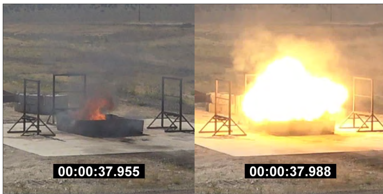
Photo 90: External Bonfire #2 Test Progression - Explosion of Fine \text{Mg\&Al-MoO}_3\text{-CuO} Thermite - Mix ID #8 (SMS mixed)
