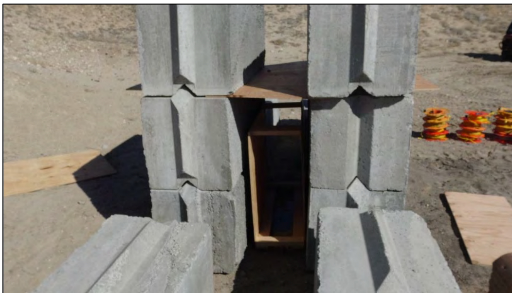
Photo 5: Secured Plywood Covering the Top of the Modified Stack Test Structure
