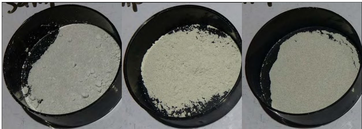
Photo 17: Small-Scale Mix ID #19 Thermite with Medium Al and SnO 2 as Fine (left), Medium (center), Coarse (right)
