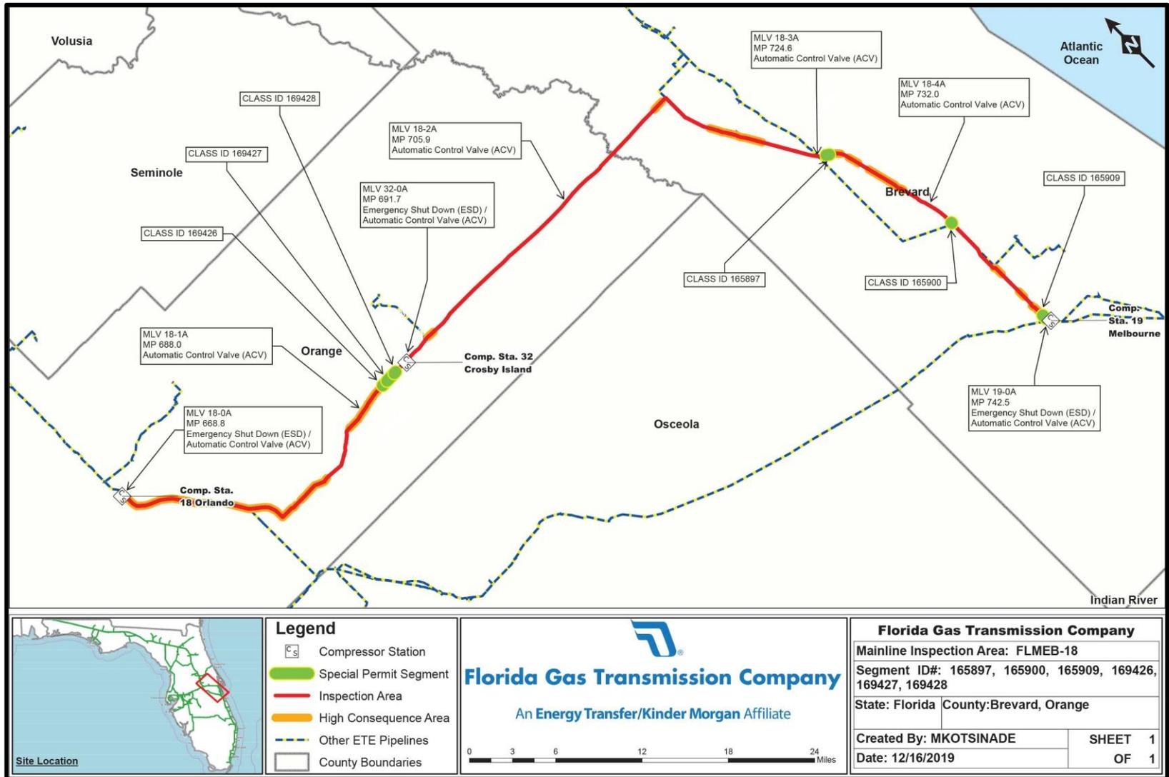
Attachment B-3 - FGT Route Map - Special Permit Segments and Special Permit Inspection Area
