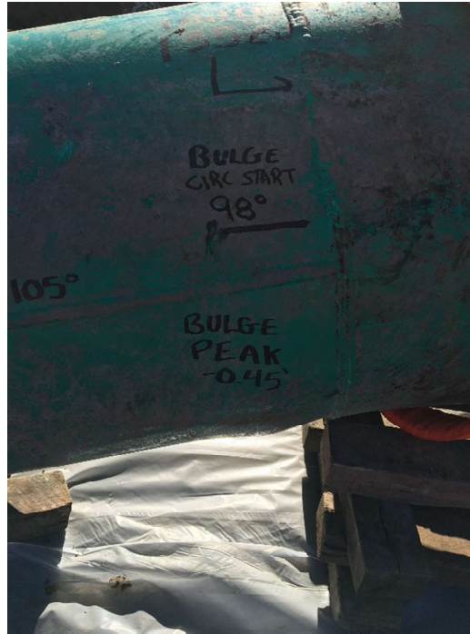
Figure 5: Photo of Bulge Upstream of Elbow
