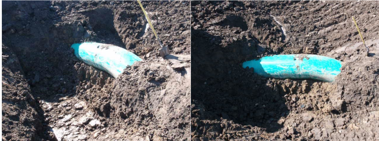
Figure 72. Photos Showing Soil Support Beneath TAG 98 (March 1, 2013)
