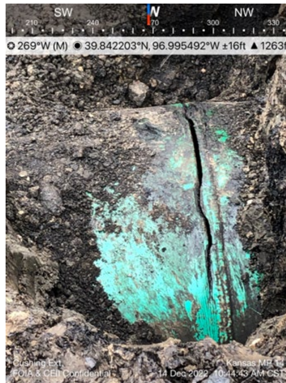
Figure 6. Excavated Failure Feature Showing Girth Weld Crack – December 14, 2022
