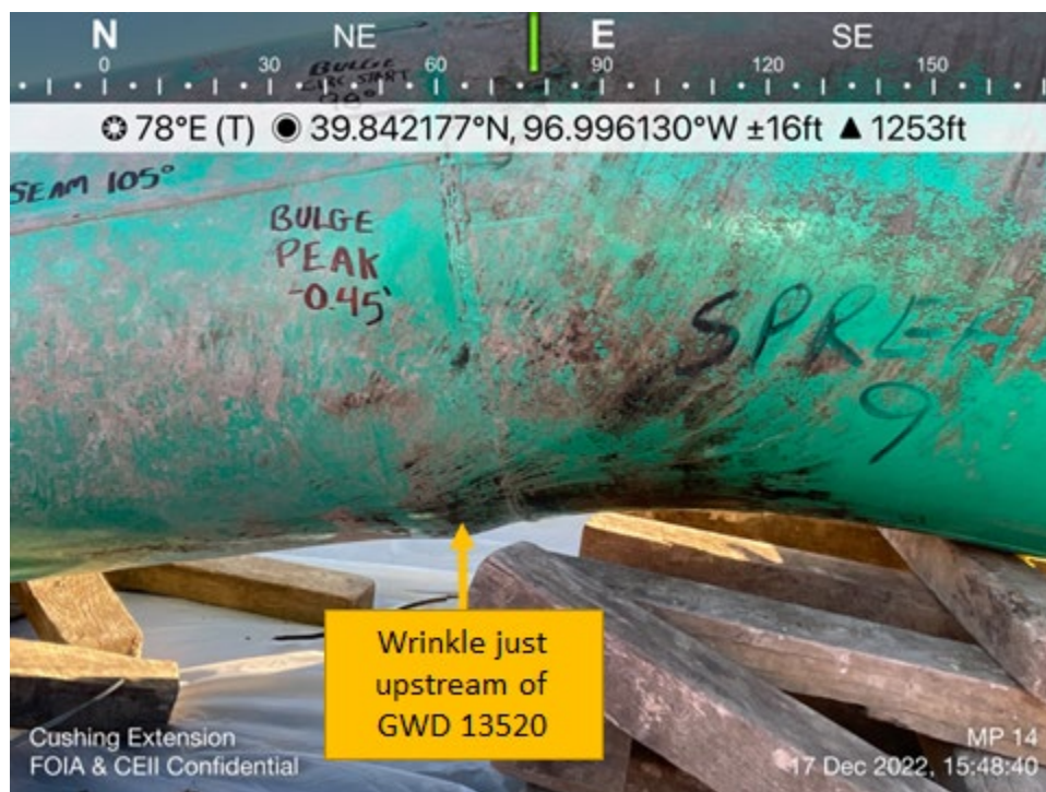
Figure 7. Wrinkle Feature Upstream of GWD 13520 – December 17, 2022
