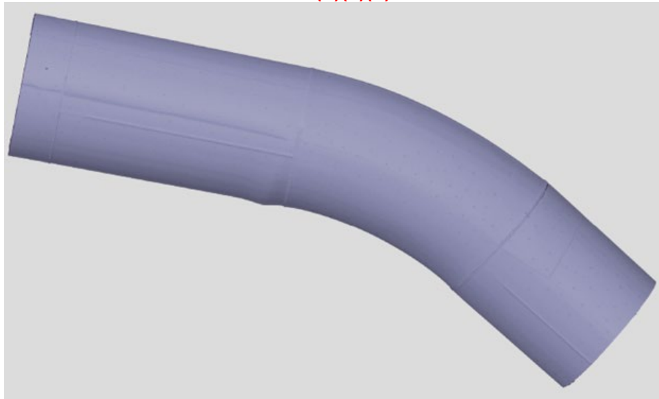
Figure D.3. STL Model of the Elbow from Laser Scanner
