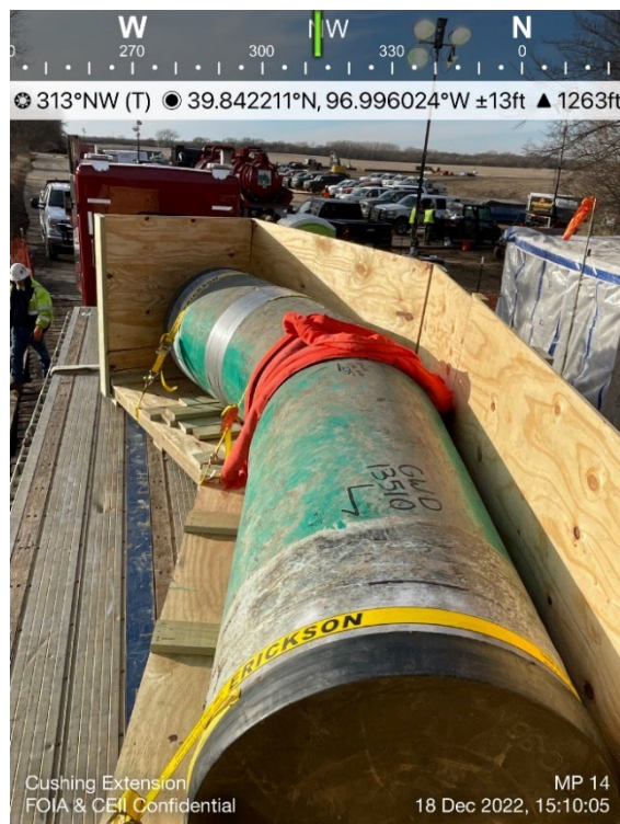
Figure 9. Pipe Segment Sent to Anderson for Metallurgical Evaluation (December 18, 2022)
