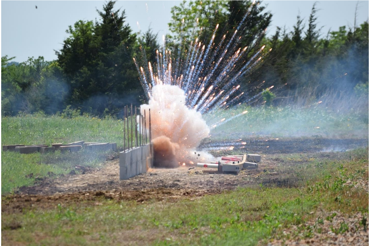
Figure 6. Ignition of Pyrotechnic Shell due to Impact.
