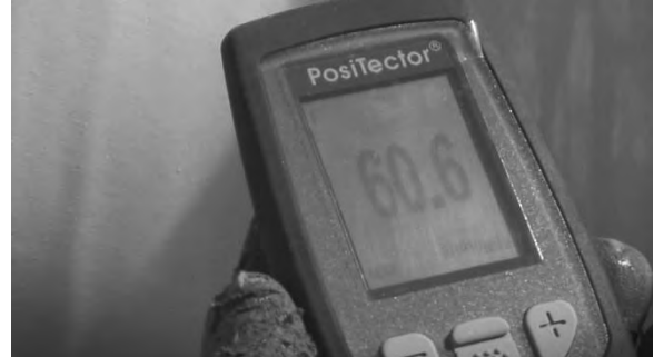
A dry film thickness gauge to check coating thickness.
