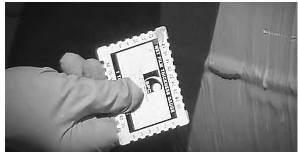
A wet film thickness gauge to check film thickness during application.
