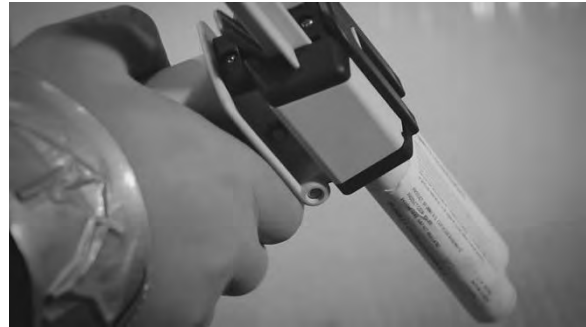
An SPC cartridge system with a dispense gun and static mixer
