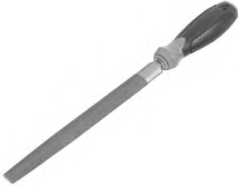
A steel file to remove weld spatter.
