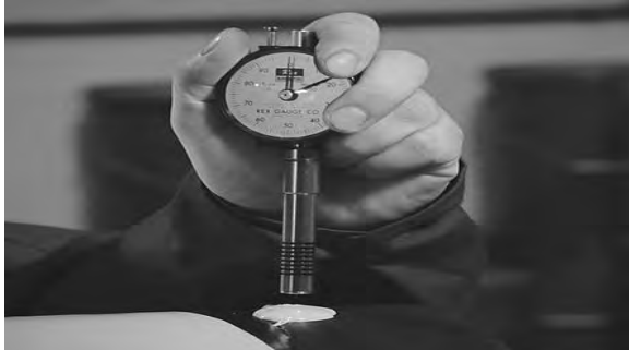
A Shore-D durometer hardness tester to measure coating hardness.
