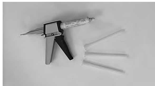
OR an SPC epoxy cartridge and dispense gun with static mixer
