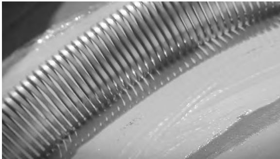
A holiday detector to test for coating imperfections.
