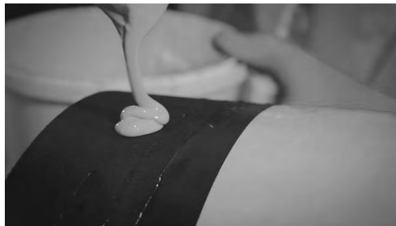
The test sample must be placed at the top and outer edge of the newly applied coating.
