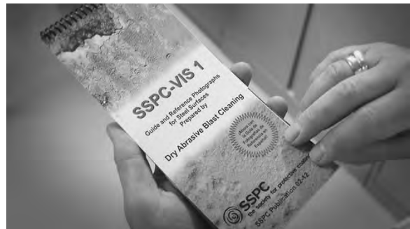
Blasted steel or visual photo comparators to determine the accuracy of the steel blast.
