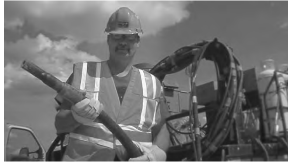
An abrasive blaster to clean the surface area, produce an anchor profile and enhance surface adhesion.
