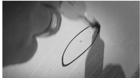
And a felt pen to mark coating deficiencies.
