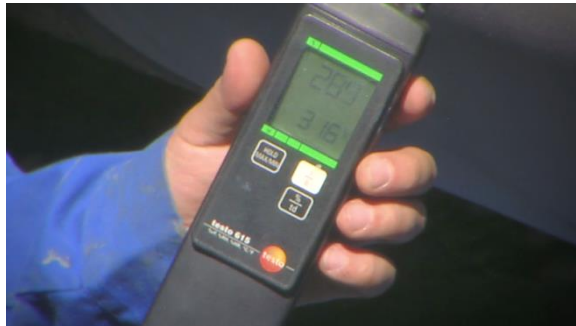
A digital hygrometer to measure ambient temperature, dew point temperature, and relative humidity.
