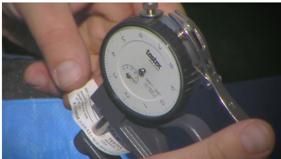
A Testex spring micrometer and replica tape to measure surface profile of the substrate.
