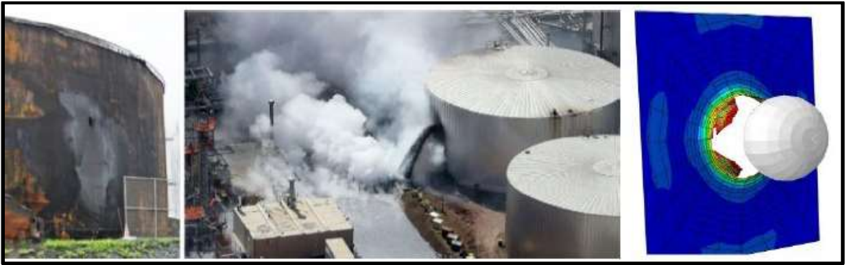
Figure 9 Modeling cascading effects from vapor cloud explosions to improve safety guidance. Courtesy DNV GL.
