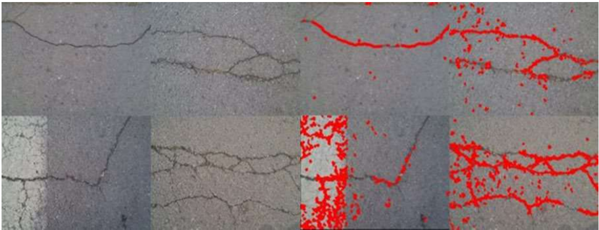
Figure 7 Testing with artificial intelligence analysis (shown in RED) of structured light sensors to improve defect detection.
