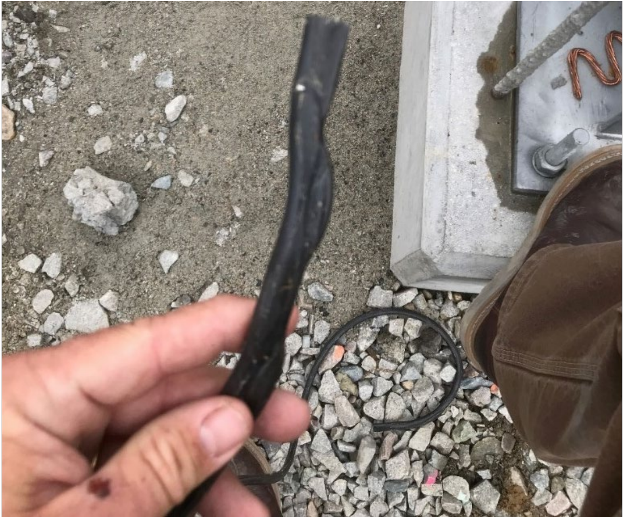
Figure 5. Photograph provided by AGT showing the failed O-ring.
