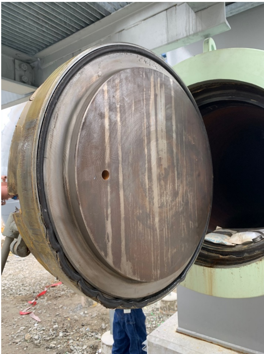
Figure 6. Photograph provided by AGT showing a similarly damaged O-ring on a closure door of Filter Separator FS-02. Desiccant packs can also be seen inside the closure hub.
