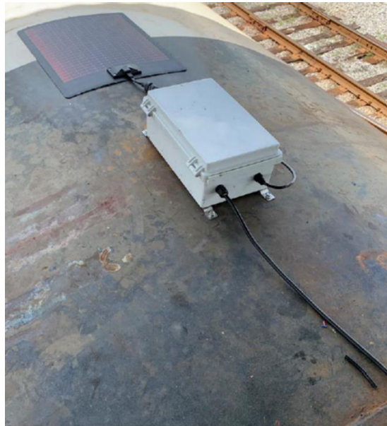
Figure 4.3 - Solar Panel and Battery Box
