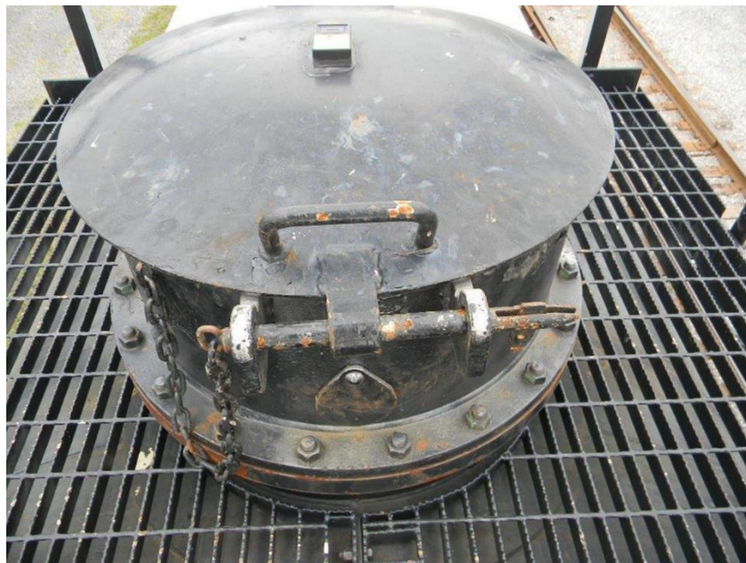
Figure 4.1 - Traditional Dome Hatch Lock Configuration
