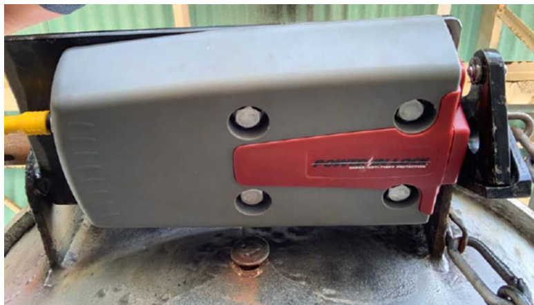
Figure 4.5 - Power-In-Lock Attached to Mounting Plate and Cabled to Solar Panel
