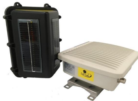
Figure 3.2 - LoRa Hardware (left: STU, right: Lat-Lon gateway)
