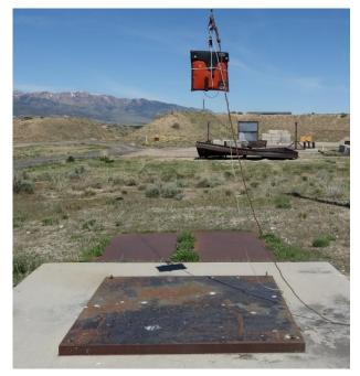
Figure 31: Fire Containment Concepts 14" PED SAFE-PAK Drop Test Setup
