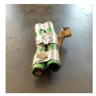
Figure 38: Batteries After Failure in Thermal Test
