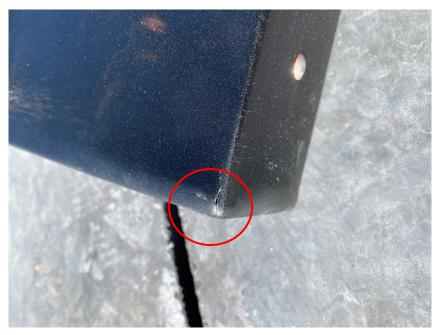
Figure 29: Cracking Sustained by the Container After the First Drop Test in the Lithium Fire Guard PG100
