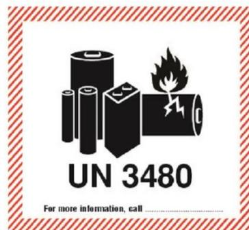
Figure 3: UN 3480 Lithium Battery Handling Label
