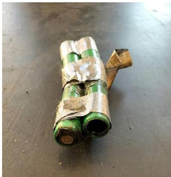
*Figure 38: Batteries After Failure in Thermal Test*
