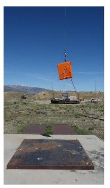
Figure 35: Brimstone Battery Fire Containment Bag Drop Test Setup
