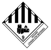
Figure 2: Lithium Battery Class 9 Placard
