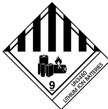
Figure 2: Lithium Battery Class 9 Placard
