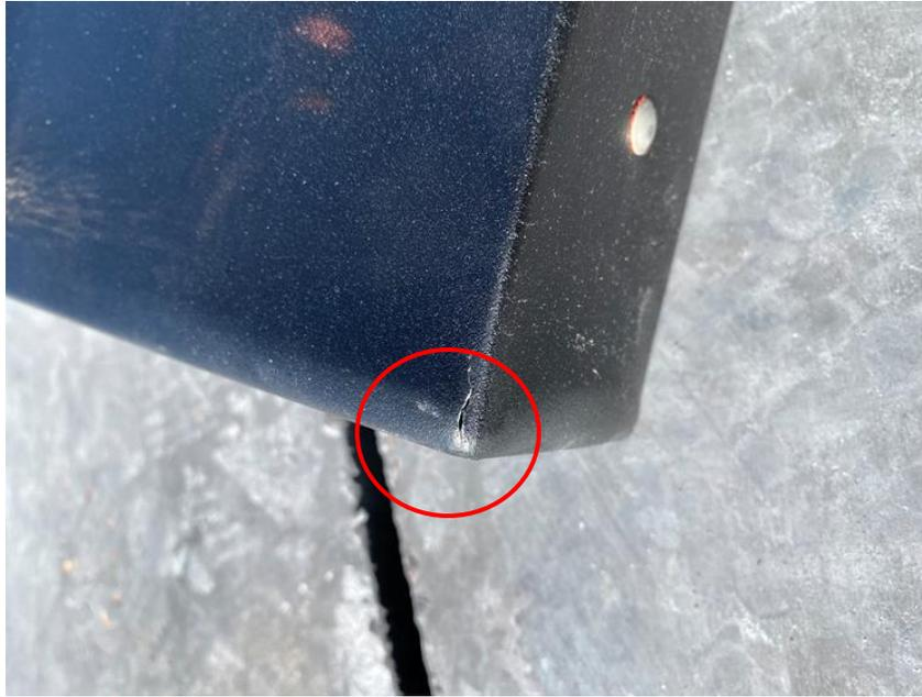
*Figure 29: Cracking Sustained by the Container After the First Drop Test in the Lithium Fire Guard PG100*
