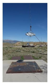
Figure 33: Newtex Z-Block™ Fire Containment Tote-Style Bag Drop Test Setup
