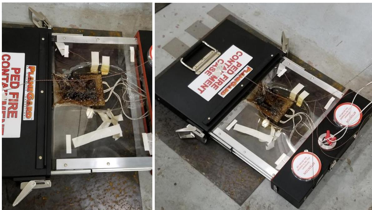
*Figure 37: Melted/Burned Internal Plastic – Post Test*
