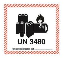
Figure 3: UN 3480 Lithium Battery Handling Label
