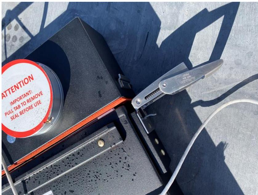
*Figure 30: Open Latches After the Second Drop Test in the Lithium Fire Guard PG100*
