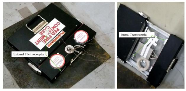
Figure 21: External Thermocouples – Pre-Test
