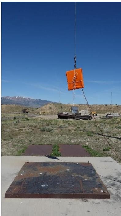
Figure 35: Brimstone Battery Fire Containment Bag Drop Test Setup
