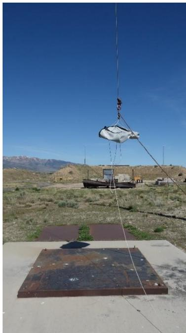
Figure 33: Newtex Z-Block™ Fire Containment Tote-Style Bag Drop Test Setup
