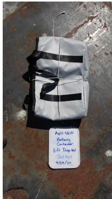
Figure 34: Newtex Z-Block™ Fire Containment Tote-Style Bag Drop Test Result
