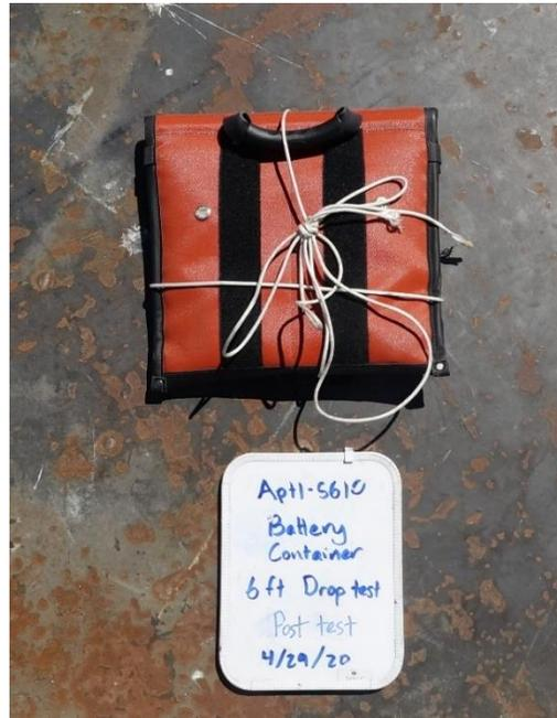
Figure 32: Fire Containment Concepts 14" PED SAFE-PAK Drop Test Result
