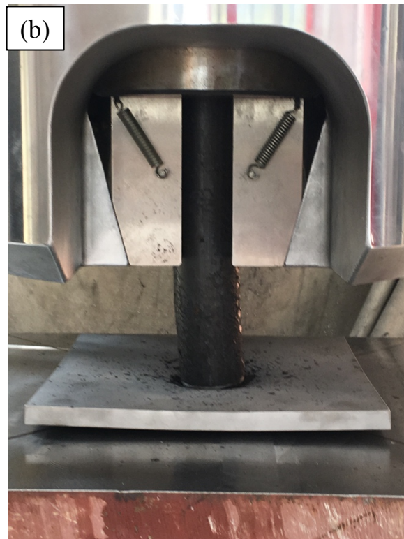
Figure 18. (a) Solid Work design of the puncture test set up for quasi-static loading and (b) bottom deformed puncture tool under loading.
