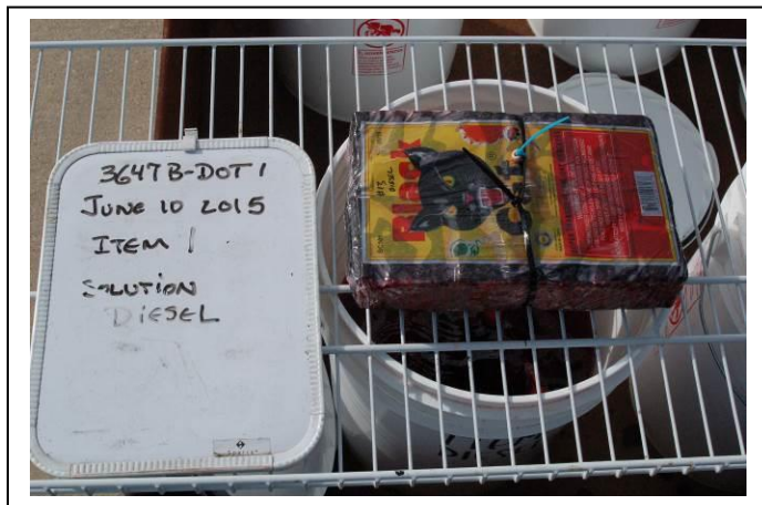
Figure 10: Firecrackers from diesel are drained on grate over the container.
