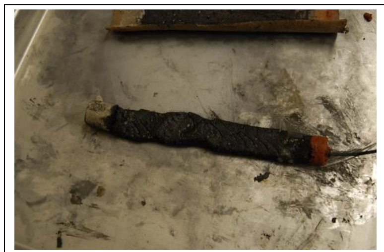
Figure 26: Fountain powder from Water, totally saturated and pasty texture, Level 3
