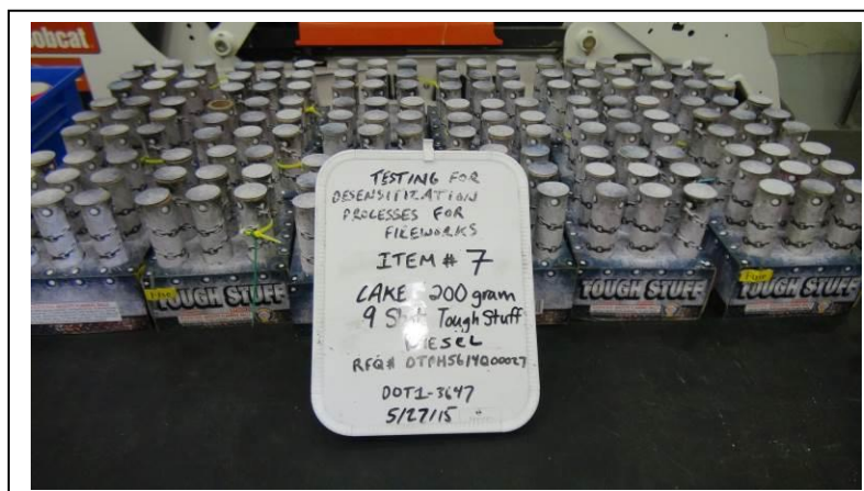
Figure 3: 200 Gram Cakes prepared for Diesel Solution soaking. Each article was marked with a bead and zip tie fastened around one of the aerial tubes.
