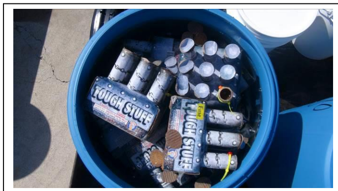
Figure 7: 200 gram cakes were placed in a 57-gallon drum and covered with solution.
