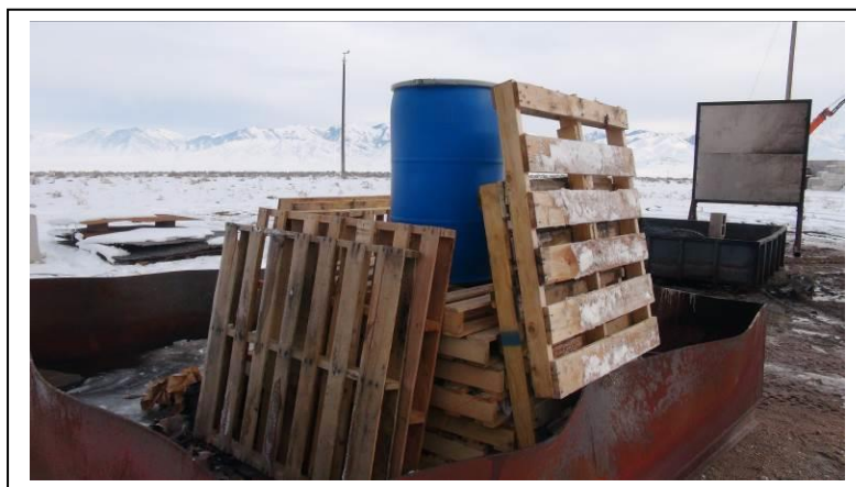
Figure 45: Fire stack arrangement typical for the batch process tests.
