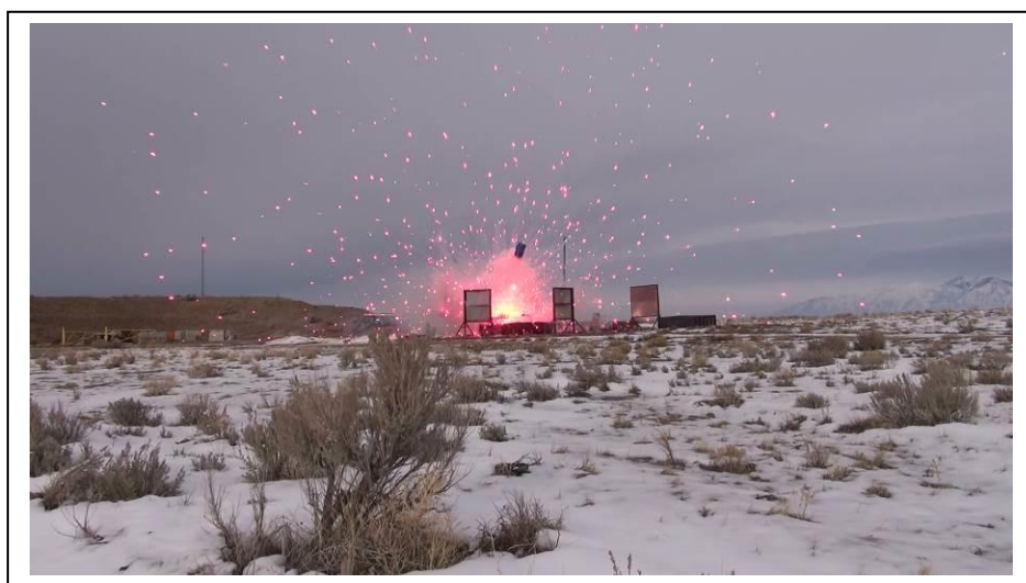
Figure 46: Baseline dry shells event with 6 inch shell. Dark object above screens is the drum that was blown up into the air.
