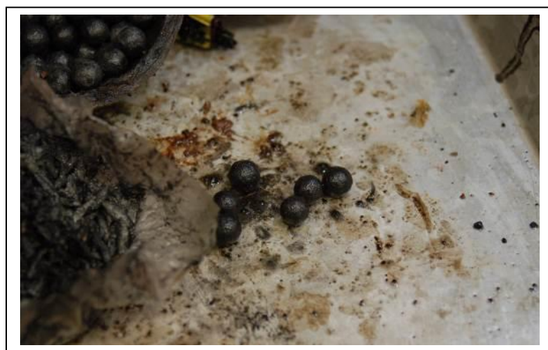
Figure 23: Wet but hard stars from 3-inch shell in diesel, Level 8.
