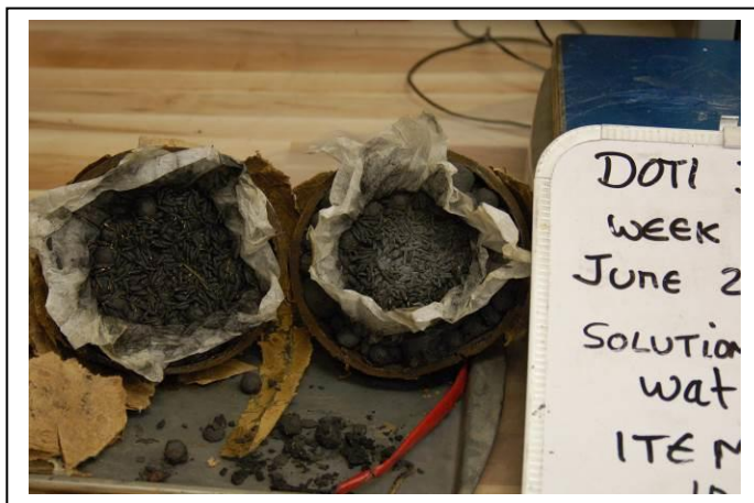
Figure 13: Shells were cut apart, contents examined and condition recorded. This 6-inch shell shows signs of crumbling stars after 3 weeks.
