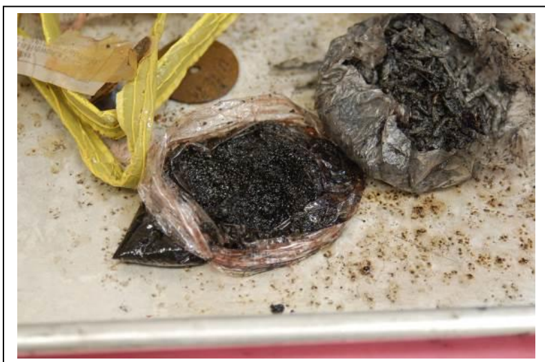
Figure 22: Gritty powder after soaking in Diesel, Level 6
