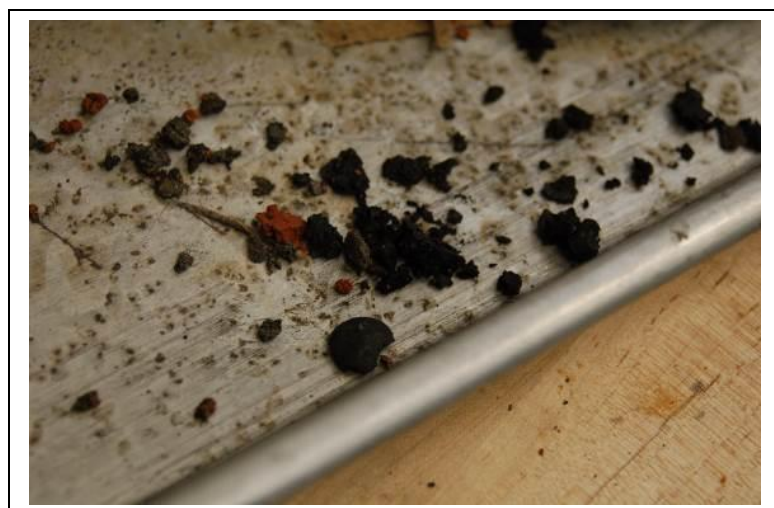
Figure 25: Star from Roman Candle in Water/Soap, totally crumbly under finger pressure, Level 5.
