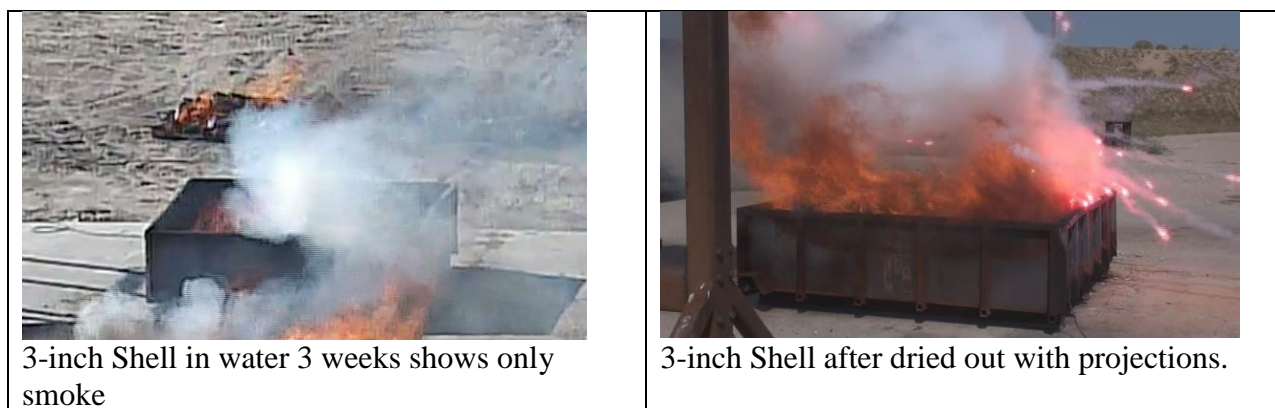
Figure 34: The water soaked 3-inch shell showed similar results with fireball and projections after a 3-week drying period, returning to a 1.4 class reaction.
