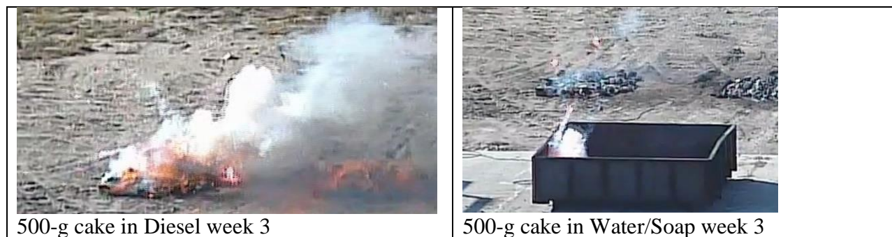
Figure 32: Comparison of events from 500-gram Cake at week 3 in Diesel and Water/Soap show both still throw projections over 3 feet, but Diesel reaction is much larger.
