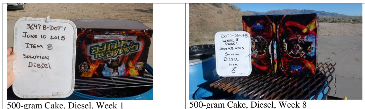
Figure 19: Diesel has the least effect of all solutions on the physical deterioration of the articles.
