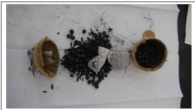
Figure 21: Dry stars and burst in 3-inch shell, Level 10.
