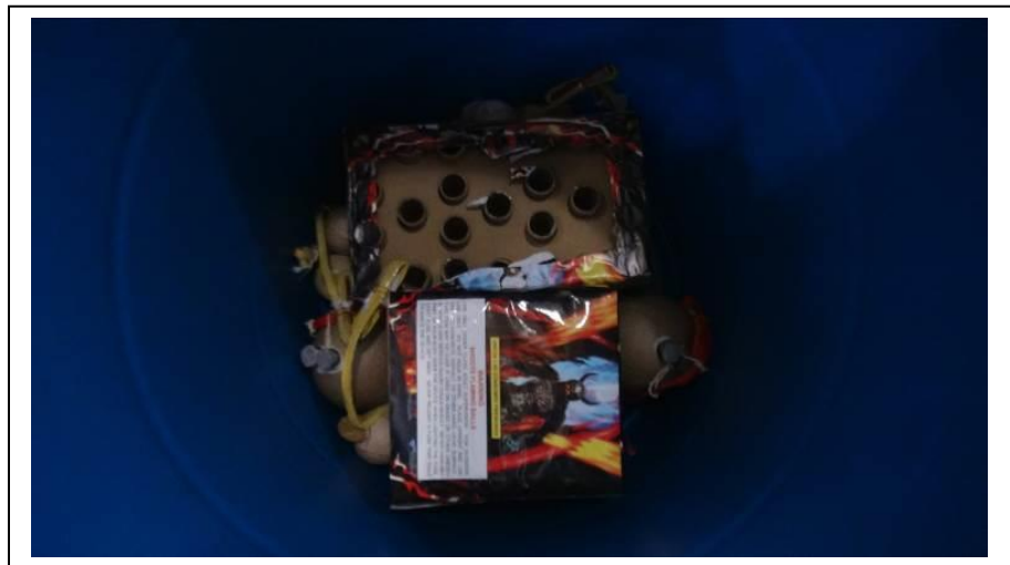
Figure 41: Bottom layer with shells and large cakes. Order of loading was not specific. Materials were placed to take up space.
