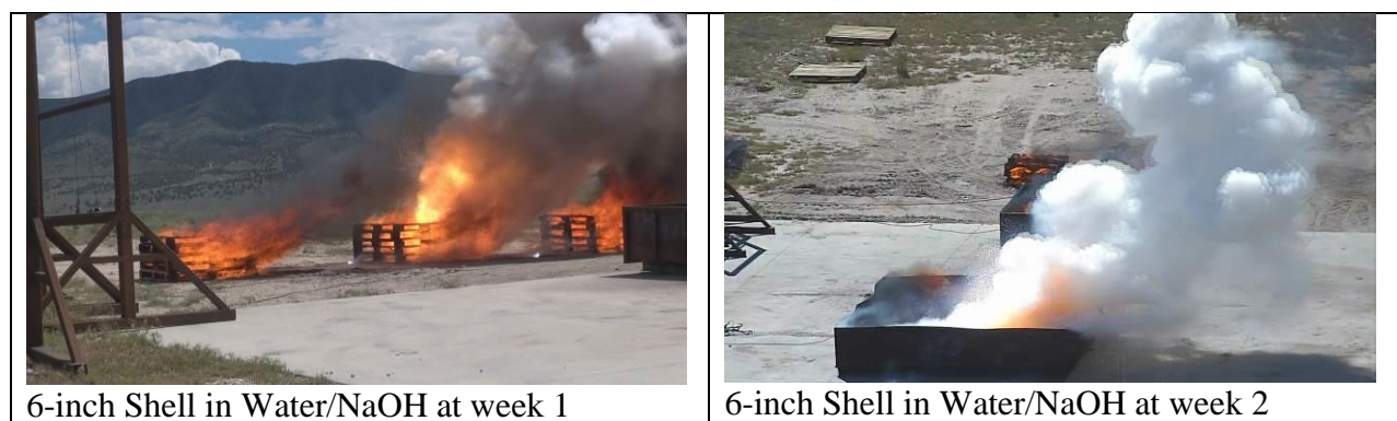
Figure 31: Progressive decrease in reactivity is quickly noted between weeks 1 and 2 in Water/NaOH moving from 1.4 to a 4.1 reaction level.
