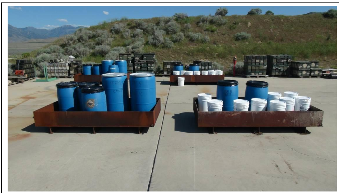
Figure 9: Containers used for soaking were labeled with solution and item number and placed in containment pans. Two pans were used for each solution. The pans were located on a concrete pad in an outside storage area.
