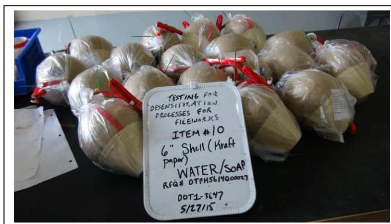
Figure 4: The 6-inch shells were marked on the fuze with a bead and zip tie. The plastic wrapping around each shell was breached with tears to allow solution to contact the shell directly.
