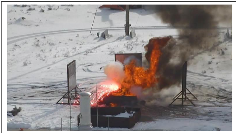
Figure 49: Maximum event from Diesel fire throws effects about 15 feet.
