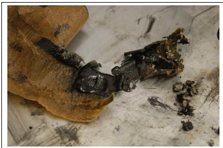
Figure 27: Sky Rocket powder liquefied in Water/NaOH solution, Level 1.
