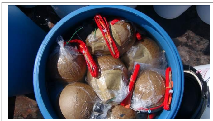
Figure 8: The 6-inch shells were placed in a 30-gallon drum. Initially floating, the shells eventually sunk below the surface.
