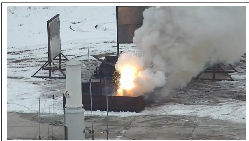
Figure 50: Maximum event from water soaked fireworks shows that drying will allow materials to burn.
