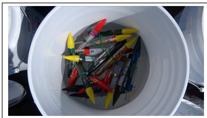
Figure 6: Sky Rockets in Water float but would eventually saturate and sink to the bottom of the container.
