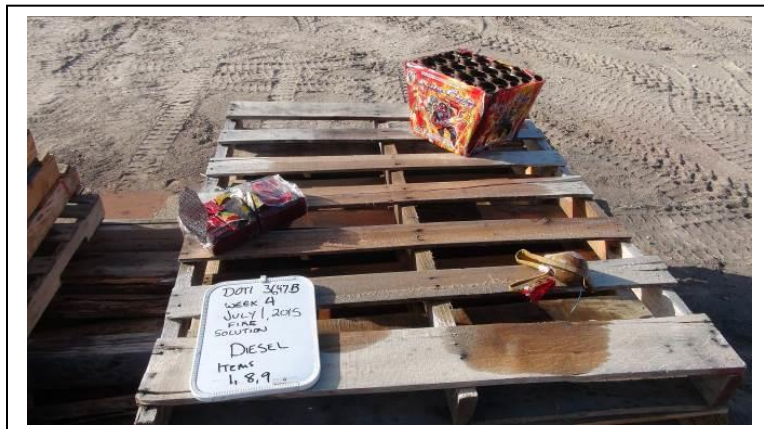
Figure 15 shows a typical wood fire. Two to four articles were typically placed on each pallet stack. Their locations were marked on a layout sheet that accompanies the test data.
