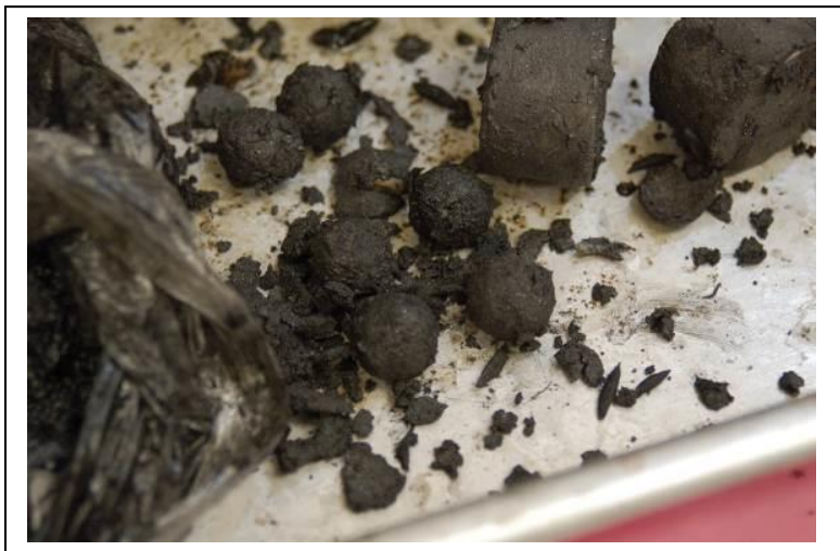
Figure 24: Crumbly exterior with hard center from 6-inch shell in Water/Soap, Level 7.
