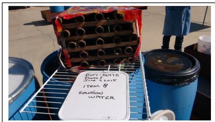
Figure 11: 500-gram cake was tipped on its side to drain standing water from inside tubes
