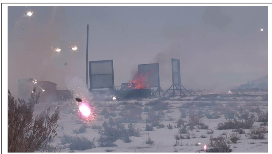
Figure 48: Exploding aerial effect from 500 g cake near camera at 150 feet from fire.
