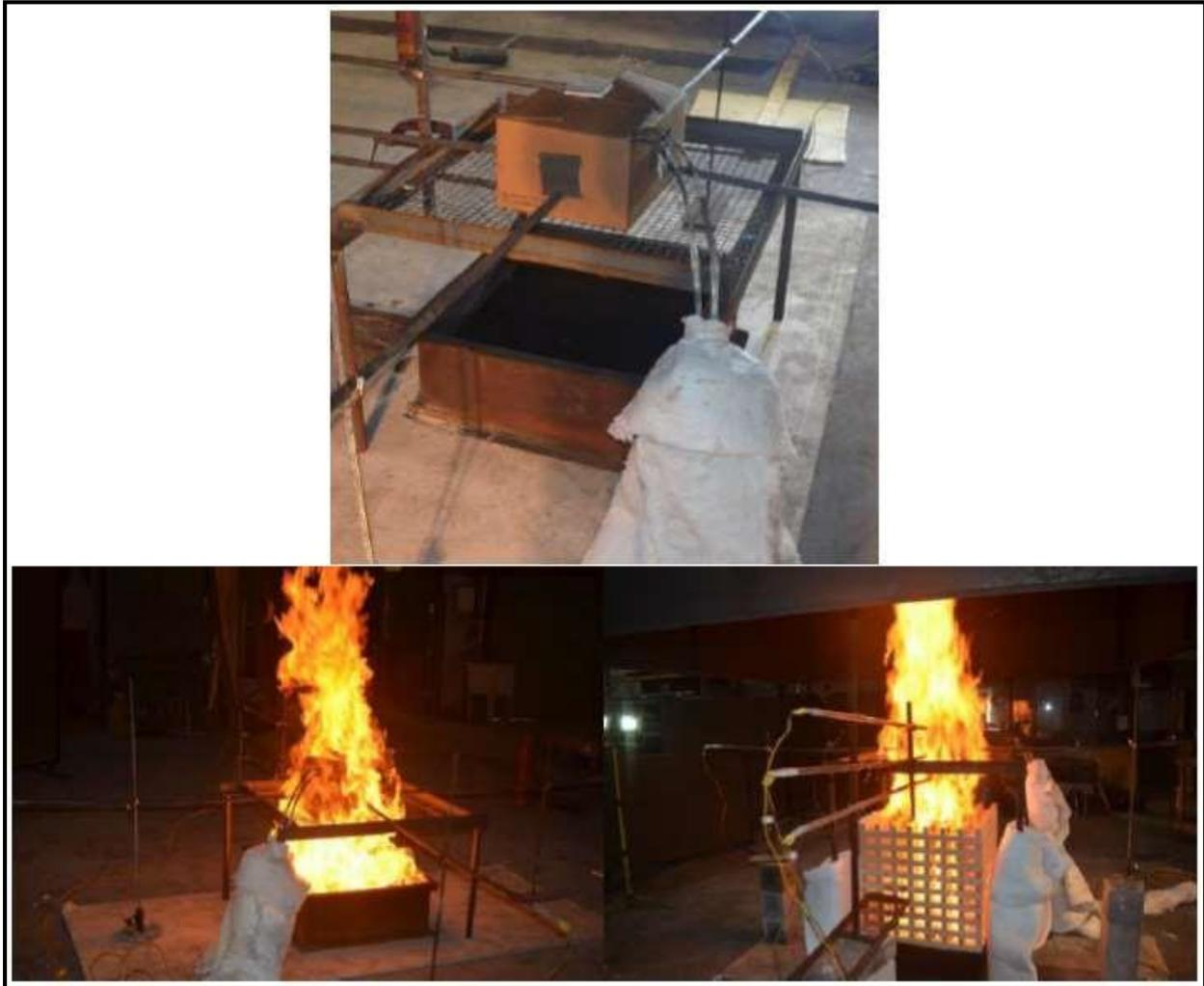
Figure 23. Typical Setup; Package (top), Pan Fire (left), Wood Crib Fire (right)
