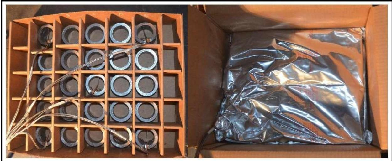
Figure 22. Tray Layer (left) and Vapor-Barrier Wrapped Tray inside 4G Box (right)
