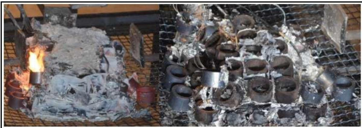
Figure 25. Package Debris and Surrogate Charges after Test 1
